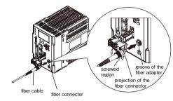
· If insertion of the fiber and tightening of the fixing screw shown as "x" on Fig. 1 and 2 are incomplete, the optical signal cannot be transmitted properly, resulting in incorrect measurement. Make sure that they are properly positioned as shown as "O" on Fig. 1
