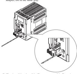
(3) Cleaning of the edge of the fiber connector of the Extension fiber cable and the Sensor Head
