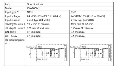
\*1 For both NPN/PNP. Wire the product properly according to the specifications of the external devices
