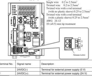
Important Wiring with the power being supplied may cause short circuit and failure of the product. Wire the
