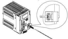
(3) Cleaning of the end face of the fiber connector of the sensor head side Remove the cap of the fiber connector, and wipe up and down the end face of the fiber connector around three times. Clean around the two guide pins as well
