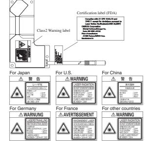
This product is classified into class 2 by the GB7247.1:2012 (IEC60825-1:2007) standard. When using in China, warning labels must be replaced by Chinese ones supplied with the product.
