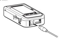
(2) For AC adapter, connect the AC plug into an outlet (100 VAC to 240 VAC). For DC cable, connect the cable with white line to the power supply (24 VDC±10%) and cable without a line into the 0 V.
