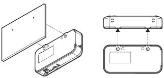
There are two hook holes below the convex section of the upper unit. Use M3 screws to hook the screw head on the screw hook holes. Set an interval of 2.5 mm or more between the bottom of the screw head and the wall surface.
