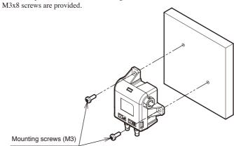
Insert the air tube into the pressure inlet. There are inscriptions at the high pressure side ( $\blacktriangledown$  Hi) and low pressure side ( $\blacktriangledown$  Lo) at the top of the pressure inlet. Properly connect air tubes according to a subject to be measured. When pressure at the high pressure side is high, the measured value is positive, and when pressure at the low pressure side is high, the measured value is negative.
