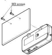
The unit screw hole depth is 4 mm. Be careful not to tighten the screw for more than 4 mm.
