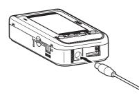
(2) For AC adapter, connect the AC plug into an outlet (100 VAC to 240 VAC). For DC cable, connect the cable with white line to the power supply (24 VDC $\pm$ 10%) and cable without a line into the 0 V.
