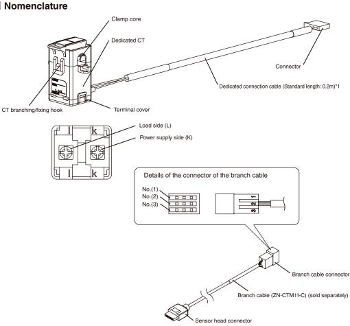
\*1 The dedicated connection cable is attached to the unit by the factory default. When replacing the terminals, connect the K side of the connection cable to the power supply side (K) of the CT terminal and the L side of the cable to the CT terminal load side (L). A recommended tightening torque: 0.69 to 0.88N•m
