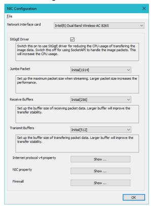
**3** Set the Ethernet card to connect the GigE camera to **Network interface card**.
