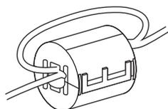
Make two loops with the cable as shown.
