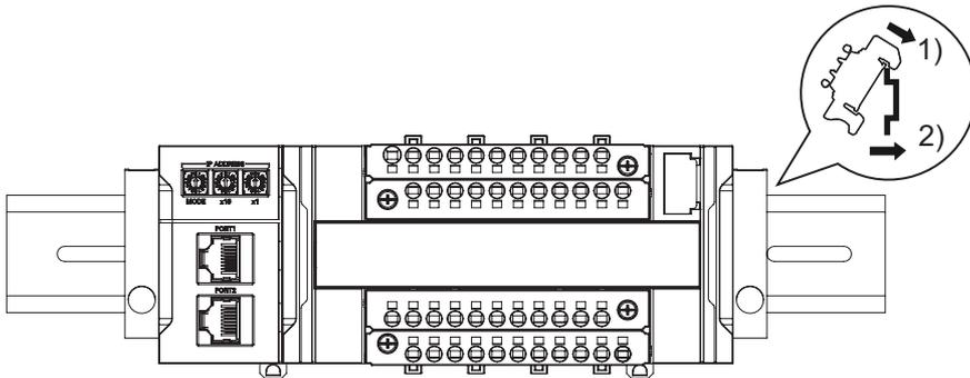
To remove an End Plate 1) insert the tip of a flat-blade screwdriver into groove "a" and 2) use "b" as a fulcrum and lift the end of the screwdriver, as shown in the following diagram.
