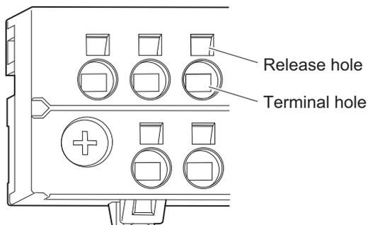
Shown above is the bottom terminal block. Layout of the top terminal block is upside down of this.
