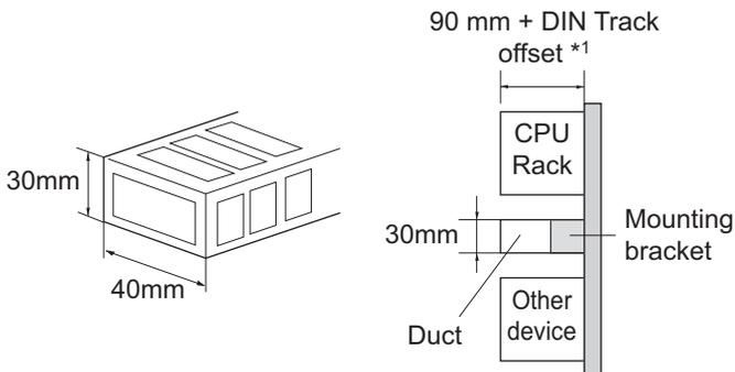
\*1. It varies depending on the DIN Track to be used. Refer to *Installation Dimensions* under 4-1-6 *Assembled Appearance and Dimensions* on page 4-12 for details. It corresponds to the dimension (B).
