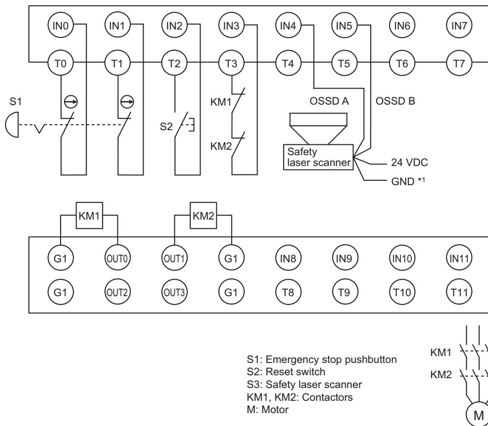
\*1. GND of the safety laser scanner must be connected to the G0 terminal of the safety I/O terminal.
