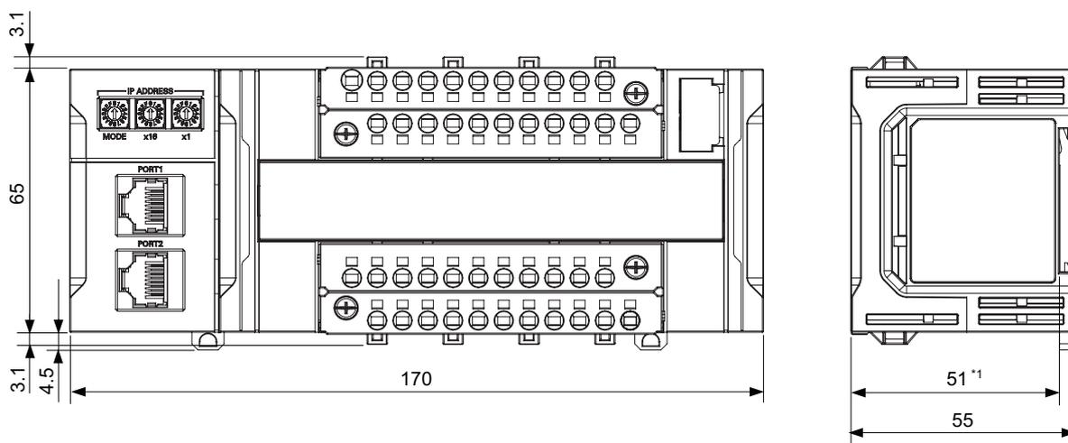
\*1. D This is a dimension from the DIN Track seat to the safety I/O terminal surface.
