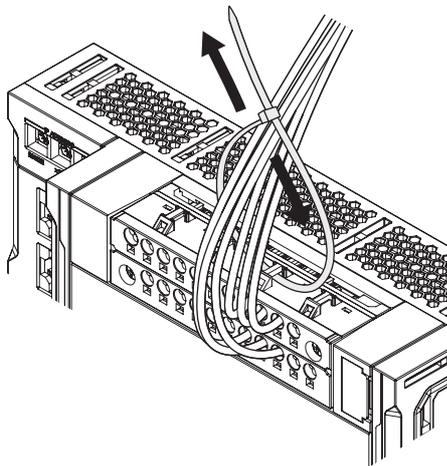
Wires must be secured so that they should be within 30mm from the screwless clamp terminal block. Also, ventilation must be ensured for above and below the CPU rack as shown below.
