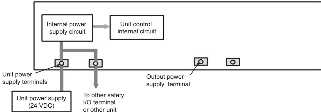
\*1.GI-SID1224 has no output control circuit and no output power supply nor output device can be connected.
