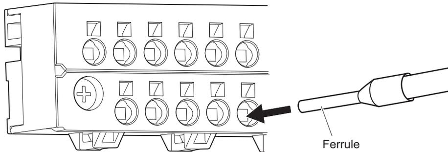
After attaching, make sure that the rod terminal is secured on the terminal block.
