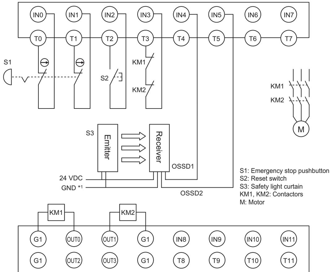
\*1. GND of the safety light curtain must be connected to the G0 terminal of the safety I/O terminal.
