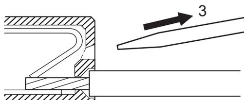
After attaching, make sure that the stranded/solid wire is secured on the terminal block.
