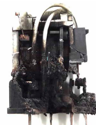
Burn damage due to insulation failure
