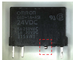
Deformation of the relay terminal
