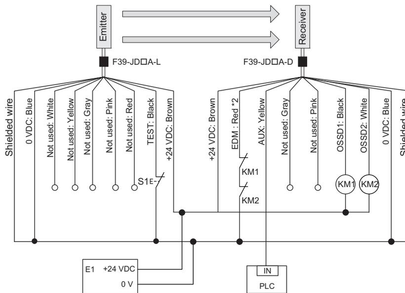
\*1. The functions are configurable with DIP Switch. Refer to *Chapter 3 Setting with DIP Switch* for more information on setting the functions by the DIP Switch.
