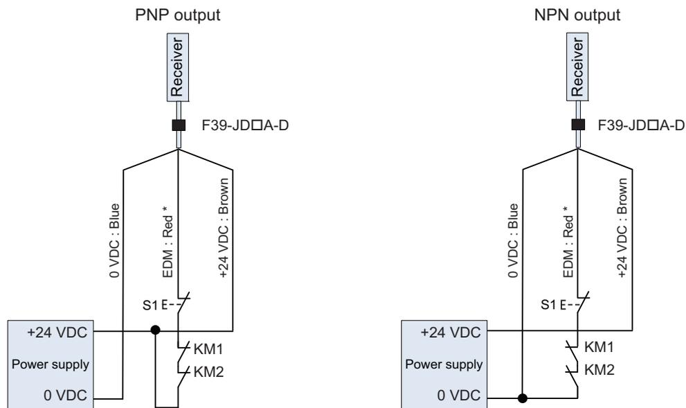
S1: Lockout Reset Switch (When the switch is not required, connect the EDM input to 24V (PNP) via the external relay (KM1, KM2) (NC contact) or 0V (NPN).
