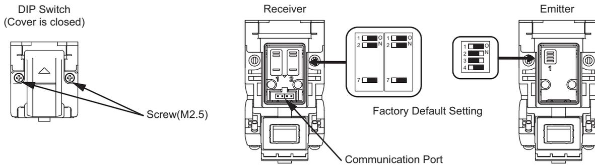
**💡** When attaching the cover, tightly fasten the screws (M2.5, recommended torque: 0.35N.m). Failure to do so may cause the cover to come loose, leading to deterioration of the protective functions.
