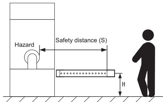
Also, you must include a hazardous condition under which a person may go through under a detection zone if  $H$  exceeds 300 mm (200 mm for other purpose than industrial use) into risk assessment.
