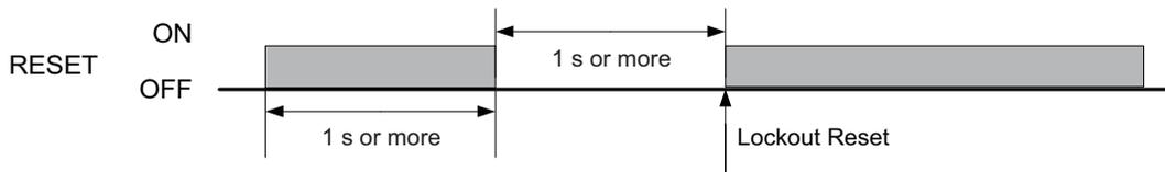
The table below shows the relation between the ON/OFF states and external lines.
