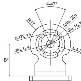
\* When you use this bracket with the Standard Adjustable Bracket (F39-LGA), the Dimension B must be 27.25 mm.
