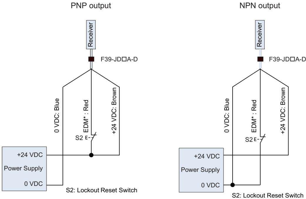
\* Also used as Lockout Reset input line.
