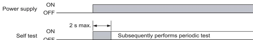
If an error is found in the Self-Test, the F3SG-R enters the Lockout state, keeps the safety output in the OFF state, and indicates the error at the same time.
