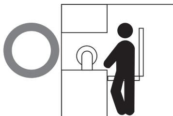
Safety distance reflects the possible access to the hazardous zone by reaching over the detection zone.
