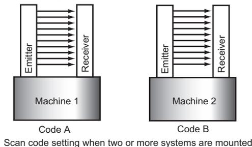
The emitter and receiver units must be set to the same scan code for the receiver to enter the Machine Run state. The scan code is selectable by the DIP Switch on the emitter and receiver units.
