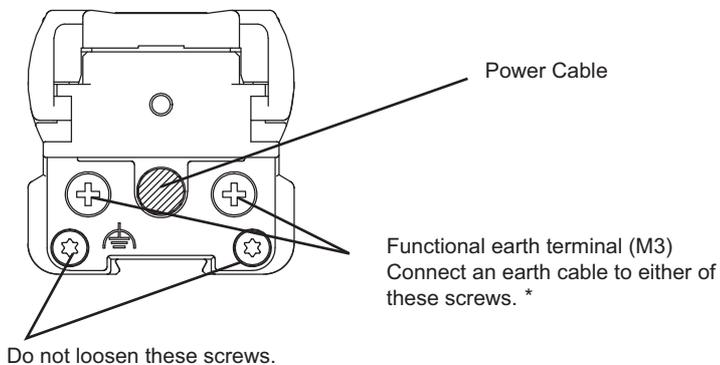
\* Select either of the terminals of the emitter and receiver according to your environment.
