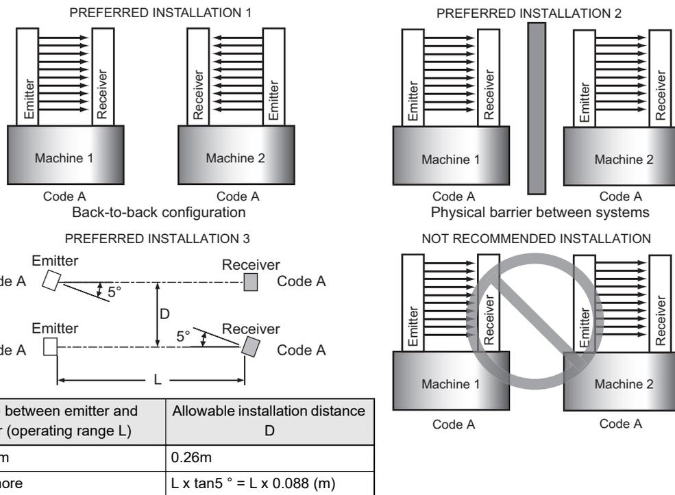
The scan code feature of the F3SG-R system allows for placement of systems in close proximity and in line with each other. The distinctive coding of the beams provide for unique operation of a system while in view of another system with a different scan code. Two unique codes are available on the F3SG-R.
