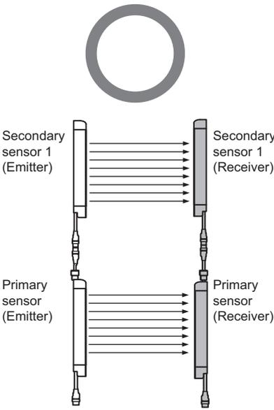
Do not series-connect an emitter and receiver. They will enter lockout state.
