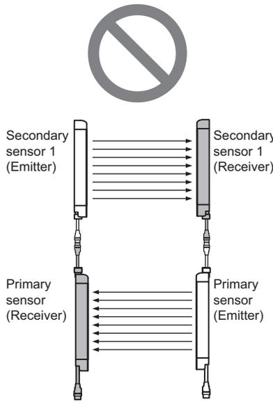
Do not face different models of emitters and receivers toward each other. They will enter lockout state or will be unable to detect objects
