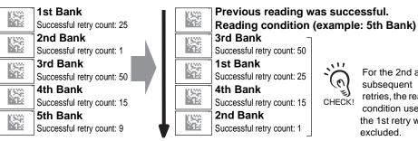
For the 2nd and subsequent retries, the reading condition used for the 1st retry will be excluded.
