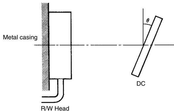
**(1) Reduction in Transmission Distance for Misalignment in V600-D23P71**
