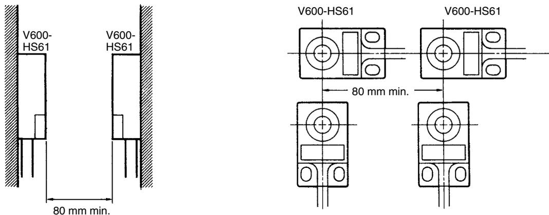
**Note** Mutual interference will not occur between R/W Heads unless they communicate at the same time. R/W Heads can thus be mounted next to each other in any application where communications will never be simultaneous. Here, “communications” refers to the oscillation of the R/W Head when a command is received.
