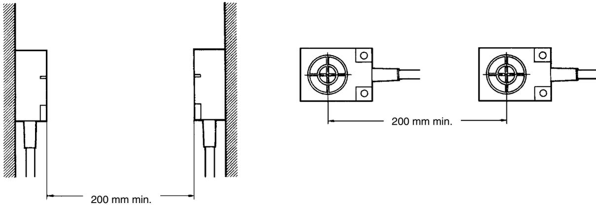
**Note** For applications in which no two R/W Heads transmit or receive data at the same time (i.e., in which the R/W Heads read and write independently), there is no risk of mutual interference and the R/W Heads can be installed in proximity. Transmission and reception in this case refer to the R/W Heads oscillating after receiving commands.
