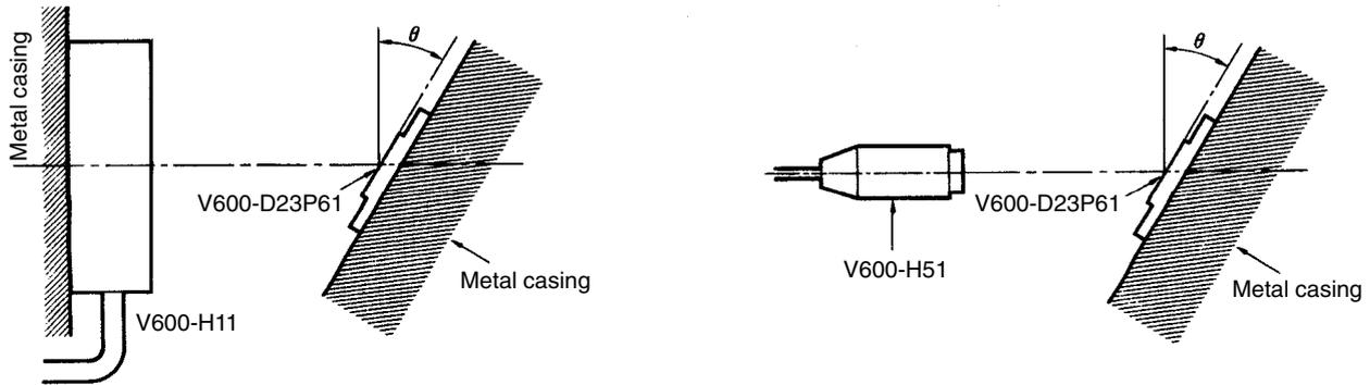
**(2) Reduction in Transmission Distance for Misalignment in V600-D23P53**
