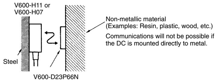
For details regarding R/W Head and DC installation, refer to *Section 4 Installation*.
