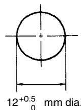
**Note** Mount the R/W Head to the bracket so that the lock washers and nuts clamp onto the bracket. The maximum tightening torque is 6 N·m (approx. 60 kgf·cm).
