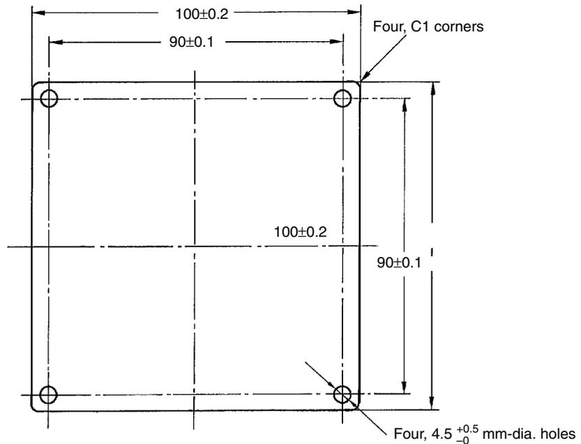
**Note** A mounting bracket is provided with the V600-H07. It is not necessary to use this bracket if a metal mounting plate larger than the 100×100 mm “footprint” of the R/W Head is used for installation.
