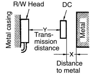
V600-A84 Holders can be used to adjust the distance between a Data Carrier and a metal surface by pilling up more than one Holder. The Holders will lock in place if they are pilled in alternating directions. Each Holder is 5 mm thick. Refer to 2-2-1 Specifications and Outer Dimensions for details.
