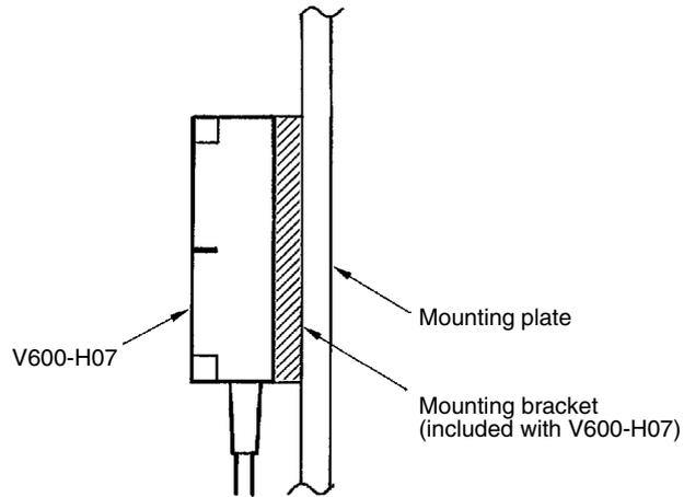
**Caution** Be sure to ground the mounting surface of the R/W Head if it is metal.
