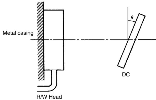
**(1) Reduction in Transmission Distance for Misalignment in V600-D23P66**
