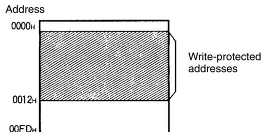
2. The entire memory except address 0000<sub>H</sub> is write-protected by setting the ending address to 00<sub>H</sub>, as shown below.
