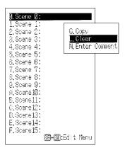
3. When "L. Clear" is selected, a message will be displayed asking for confirmation to clear the scene data. To clear the data, select "X. Execute". If you do not want to clear the data, then either select "C. Clear" or press the Escape Key.
