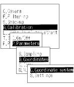
3. Set the coordinate system and unit. In this example, "righthand" is selected as the coordinate system and "mm" is selected as the unit.
