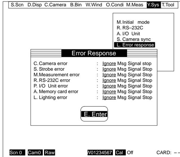
When “L. Lighting error” is set to other than “Ignore” then at the time of measurement the density in the monitor area will be checked according to the items set at the “C. Camera/L. Light level adjustment” menu. If the density fluctuates by  $\pm 20\%$  with respect to the reference density that has been set, then the error processing specified by this menu will be executed.
