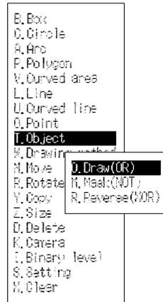
When the "T. Object" screen appears, the image type will be changed to binary.
