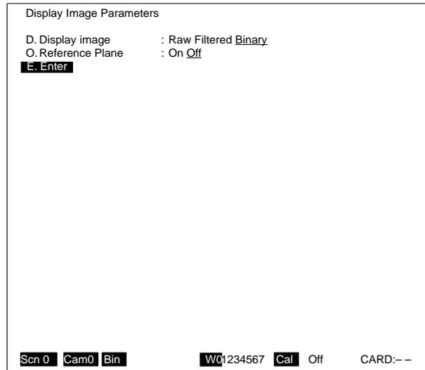
Settings made by means of this menu are valid only during window-drawing operations for the window that is currently being set. As soon as the window-drawing menu is quit, the display will revert to the status prior to the settings made in this menu. The operations are as follows for the items in this menu:
