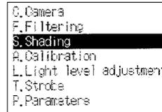
2. Select either “0. Master 0” or “1. Master 1”. Master 1 will cause the image input from the camera to be synthesized with the shading master for display. If no shading master has been created, then the display will not change even if master 0 or master 1 is selected. It makes no difference whether shading master selection or creation is executed first.
