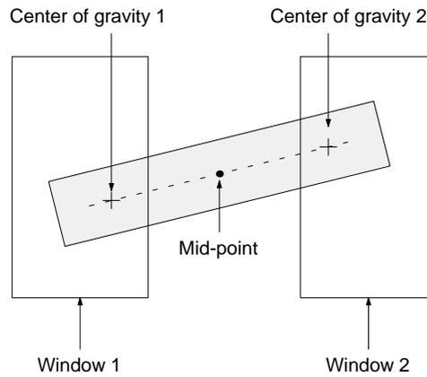
**Angle of Inclination Between the Centers of Gravity**
