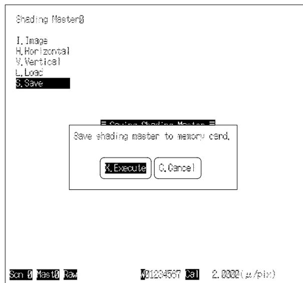
**Loading Shading Masters** Once shading masters have been saved to a memory card, they can be loaded to the F300. The shading masters will have been saved as master 0 and master 1, so select one of them before beginning operations.
