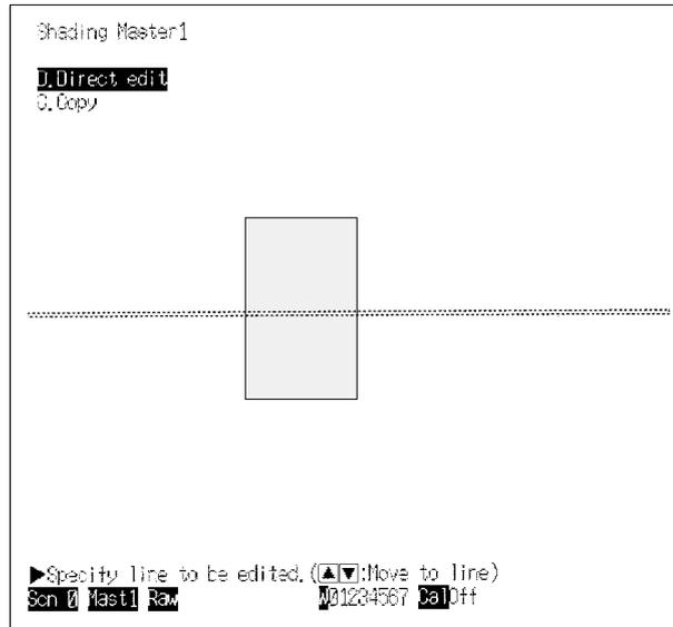
2. The light level on the specified horizontal line will be displayed as a graph. Use the Right and Left Keys to move the cursor to the X-coordinate position where the light level is to be changed. Use the Up and Down Keys to change the light level. To change several pixels on the same line, use the Right and Left Keys to move the cursor one pixel at a time and use the Up and Down Keys to change the light level for each pixel.
