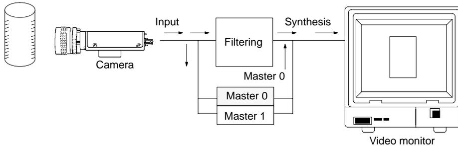
For shading compensation, the shading master is then integrated with the image input from the screen, including filtering.
