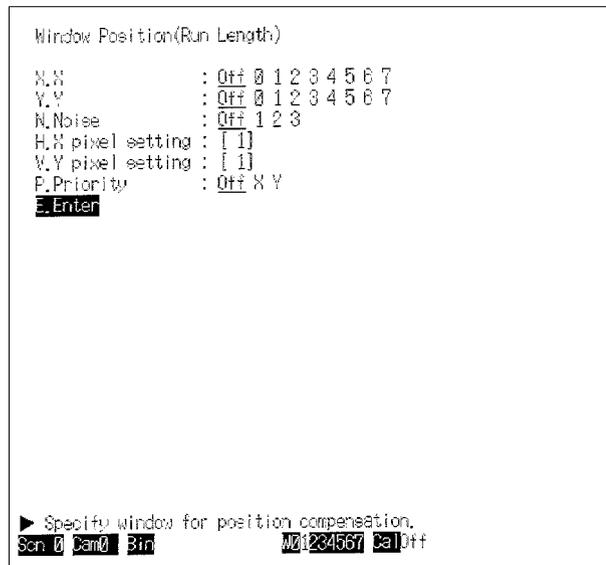
“Run length” refers to the boundary coordinates for white to black or black to white pixels. When measuring run length, use a rectangular window for the position displacement compensation window.
