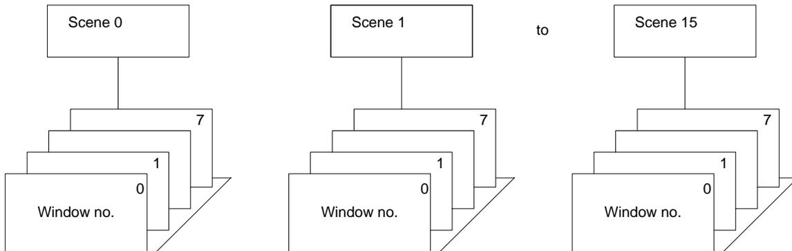
Multiple window shapes can be created for a single window plane. The data for the shape that has been drawn, the numbers of the cameras to be used, binary level, measurement mode, and the relationship to window plane 7 are all saved as window data.
