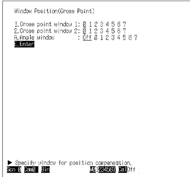
Rectangular windows must be used for measuring the point of intersection. Window 1 and window 2 must each be drawn in separate window planes.
