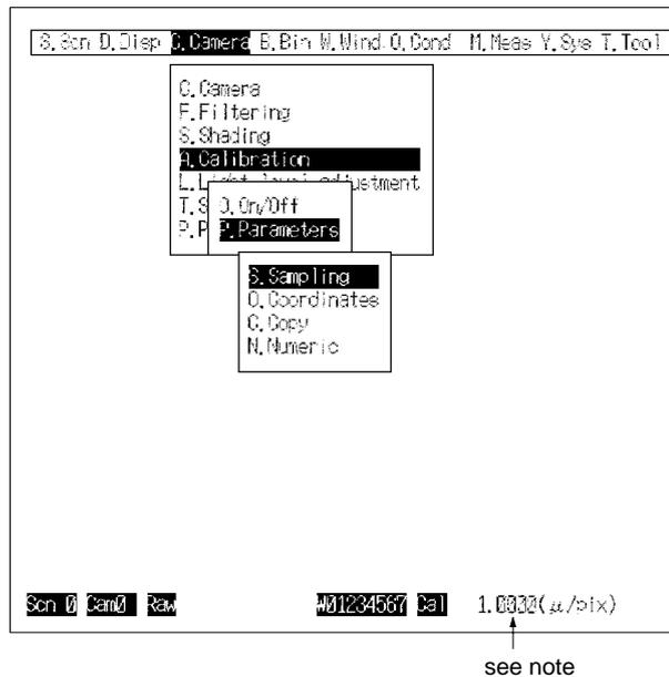
**Note** When calibration is set to On, the calibration data (the actual value per pixel) will be displayed.
