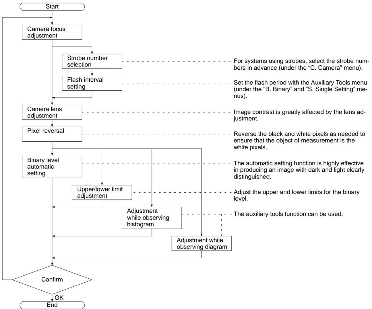
Examples on how to adjust the upper and lower limits are as follows.
