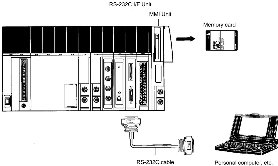
**Note** The memory card must be initialized before it can be used. To initialize a memory card, execute "C. Memory Card" under the "T. Tool" menu.
