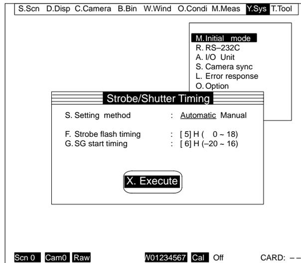
When “Automatic” is specified for “S. Setting method,” the values that have been set by the system according to the Camera I/F Units that are used will be displayed for “F. Strobe flash timing” and “G. SG start timing.” (The numbers that are displayed on the screen at that time cannot be changed.) When “Manual” is specified for “S. Setting method,” numeric values can be input for “F. Strobe flash timing” and “G. SG start timing.”
