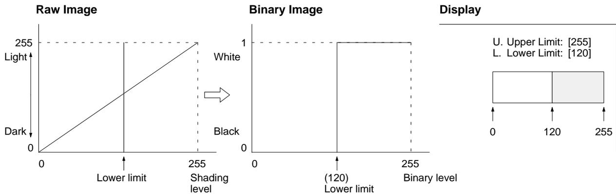
If the lower limit is set to 120, then the shading level region from 0 to 119 of the input image (i.e., the raw image) will be converted to black, and the region from 120 to 255 will be converted to white.
