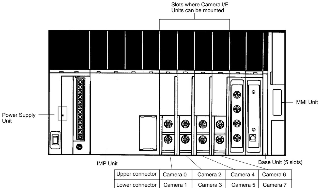
A maximum total of four Camera I/F Units may be mounted to the Base Unit (F300-B5/B3). These four Camera Units may include normal, normal simultaneously, shutter, and shutter simultaneously types.
