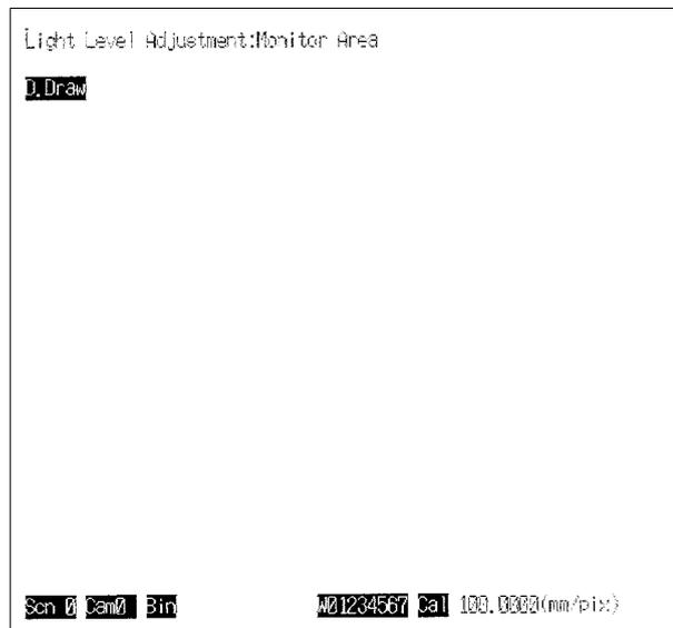
8. Designate a square in an area that will not be affected by the presence of the object that is to be measured.
