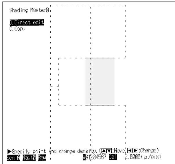
When the Enter Key is pressed, the shading master will be changed to the revised light level shown in the graph.
