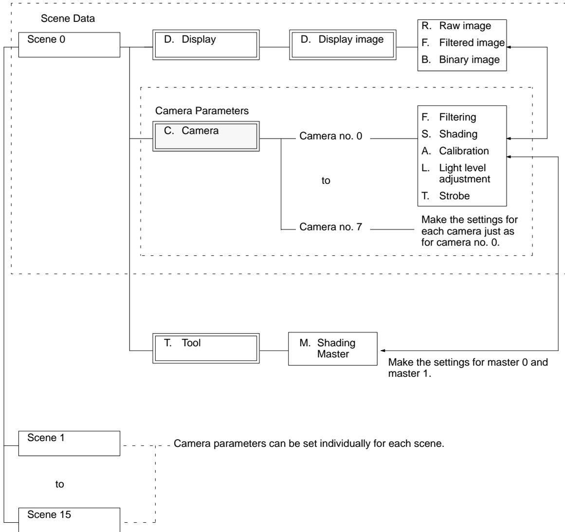
If “F. Filtered Image” is selected from the dialog box under the “D. Display” menu, the image set by “F. Filtering” under the “C. Camera” menu will be displayed.
