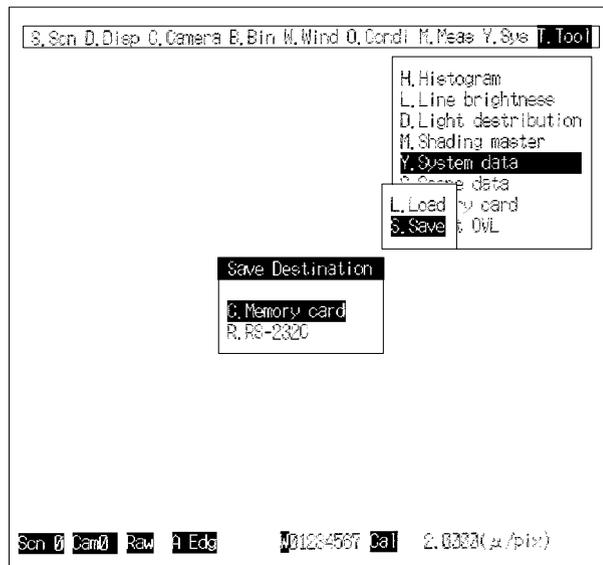
When saving to a memory card, a filename consisting of up to eight normal letters or numbers must be input. When inputting the filename, the Shift and Escape Keys can be simultaneously pressed to display a list of characters. It will then be easy to input the characters with the Console.
