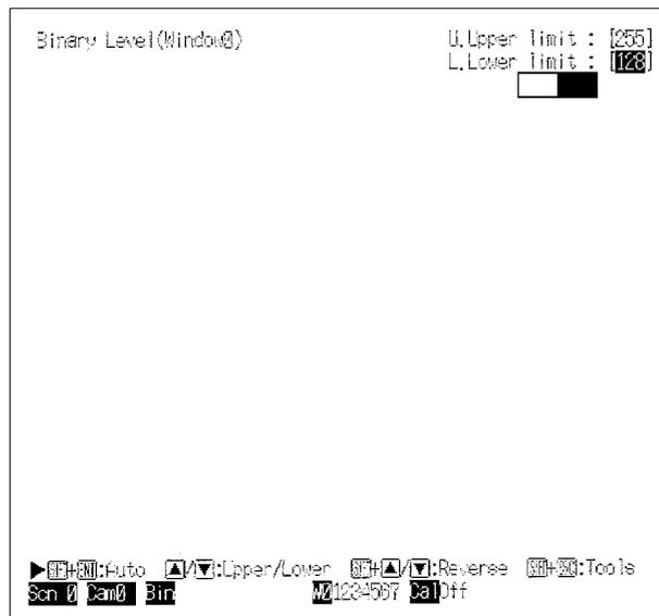
**Note** If the binary level is set with “S. Single Setting” after binary level settings have already been made for individual windows with regard to a particular camera, all of those previous settings will be changed.
