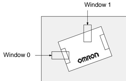
Windows for correcting the position of the windows used for measurement
