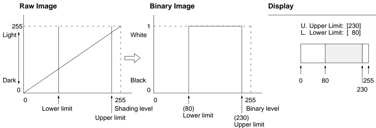
If the upper limit is set to 230 and the lower limit to 80, then the shading level regions from 0 to 79 and 231 to 255 of the input image (i.e., the raw image) will be converted to black, and the region from 80 to 230 will be converted to white.
