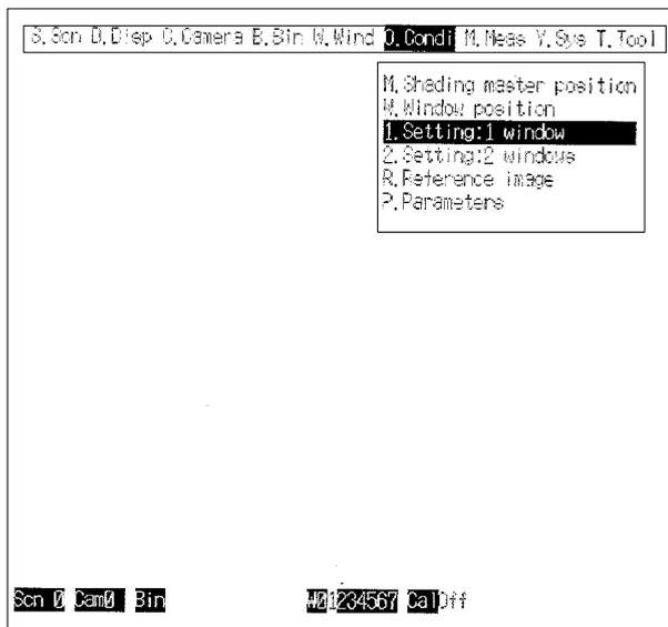
2. Select the number of the window plane to be used for measurement. You cannot overlap a window plane that has been selected for position displacement compensation.
