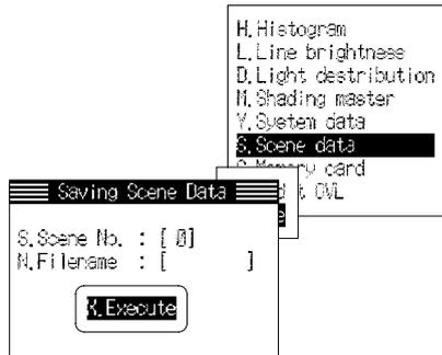
**Saving Data to a Device Connected to the RS-232C I/F Unit**
