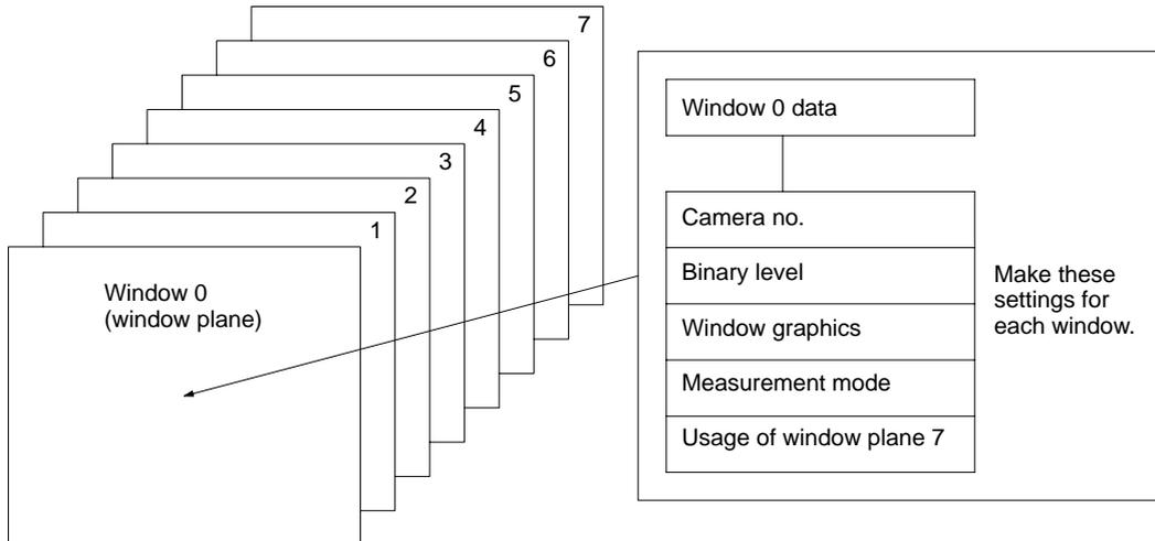
Window plane 7 can be used as an ordinary window plane, but it can also be used as a paint window or a pattern matching window for complex measurements in conjunction with window planes 0 to 6.
