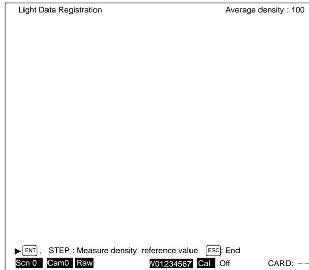
The average image density in the monitor area set by the "L. Light level adjustment" menu (accessed through "C. Camera") is measured and taken as the reference value for light level adjustment.
