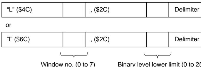
Designate the window number and the lower limit for the binary level in ASCII code.
