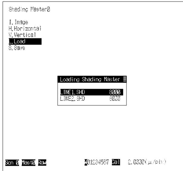
3. When "X. Execute" is selected, the data from the memory card will be loaded to the specified master number.
