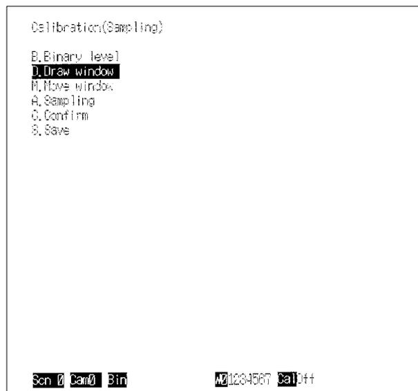
9. Move the cursor to the center of the position where the window is to be created, and then draw a circular window.
