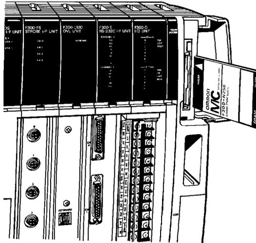
2. The memory card must be initialized before a shading master can be saved to it. To initialize a memory card, execute "C. Memory Card" under the "T. Tool" menu.
