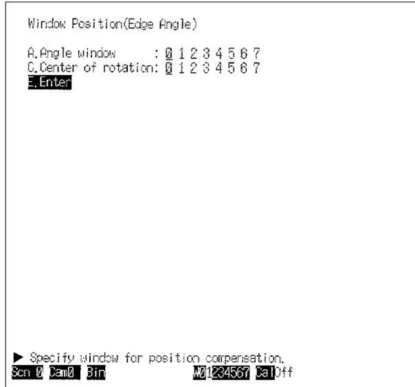
Rectangular windows must be used for detecting edge angles. Draw only one graphic in a window plane.
