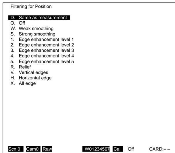
If “D. Same as measurement” is selected here, the image filtering at the time of position displacement compensation will be the same as that set for “F. Filtering” under the “C. Camera” menu. If anything other than “D. Same as measurement”
