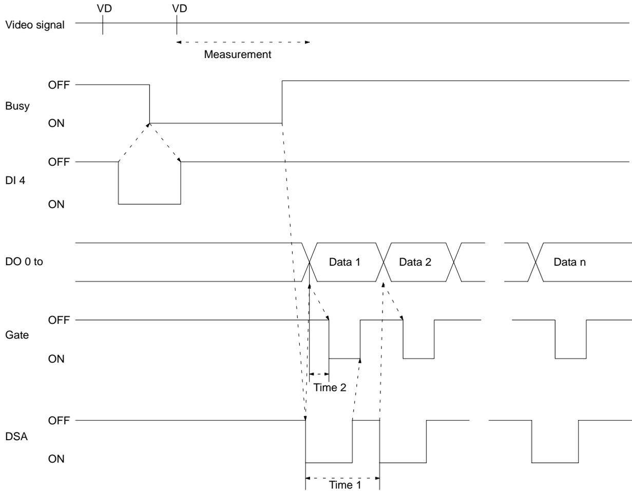
Timeout control will be based on time 1 in the illustration above. Set the maximum allowable time (the timeout) for time 1, as well as time 2, by means of the "Y. System/A. I/O Unit menu.
