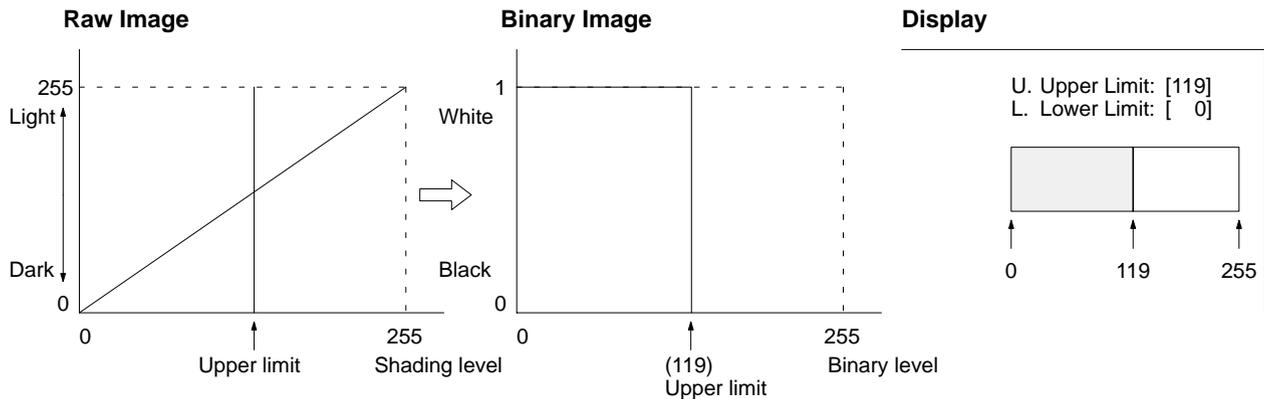
If the lower limit is left at 0 and the lower limit is set to 119, then the shading level region from 0 to 119 of the input image (i.e., the raw image) will be converted to white, and the region from 120 to 255 will be converted to black. This would be the same as reversing the results of the processing associated with setting only the lower limit, as described previously.
