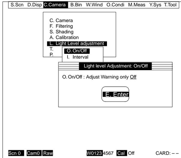
When either “Adjust” or “Warning only” is set here, an alarm will be output if the density value that was registered as a reference standard is exceeded by  $\pm 20\%$ . The alarm method can be specified by means of “L. Lighting error” (accessed through “Y. System/L. Error response”).
