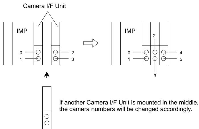
2. Do not use Normal-type Camera I/F Units and Shutter-type Camera I/F Units together.
