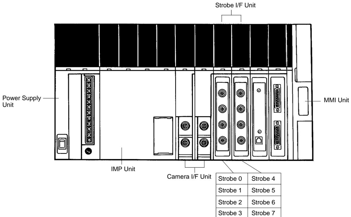
A maximum of two Strobe I/F Units can be mounted in any of the slots between the IMP Unit and the MMI Unit. When adding a new Strobe I/F Unit to an existing
