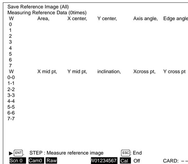
Measurement is carried out when the Enter Key is pressed or a STEP signal is input, and the measurement results are displayed on the screen. When saving images as a group, the operation will be carried out for all measurement items in all windows. When saving images window by window, it will be carried out for all measurement items in the designated window.
