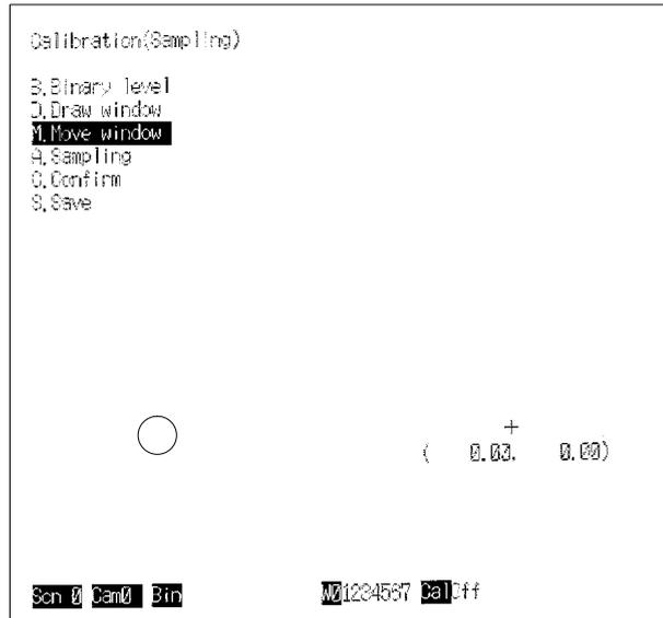
Sampling will be conducted at coordinate point (100, 0) of the graph paper, and coordinate 100 for the X axis and coordinate 0 for the Y axis will be input.
