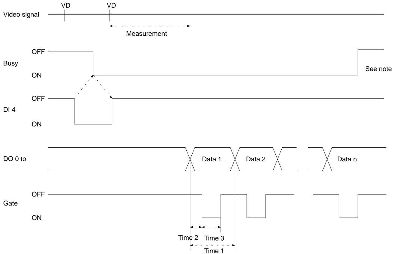
Times 1 to 3 are set with the "Y. System/A. I/O Unit menu.
