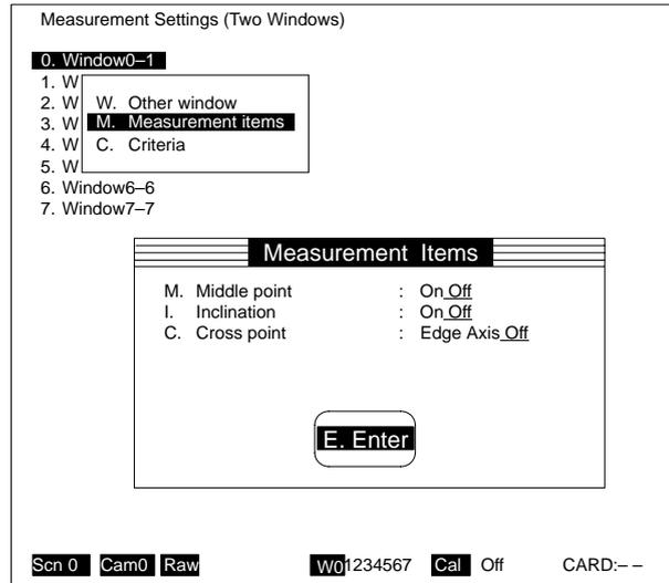
The mid-point and angle of inclination are set just as in Version 1.□□, but with Version 2.00 the user can choose between “edge cross point” and “axis cross point” for the cross point. When “cross point” is indicated on other menus, such as the menus for setting criteria or displaying measurement values, it will refer to whichever of the two types of cross point is specified here.
