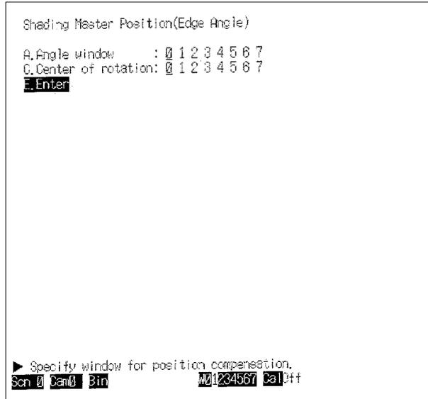
Rectangular windows must be used for detecting edge angles. Draw only one figure in a window plane.
