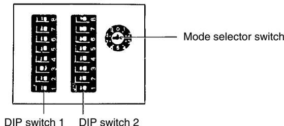
When the switch cover is opened, a mode selector switch and two DIP switches, 1 and 2, are visible.
