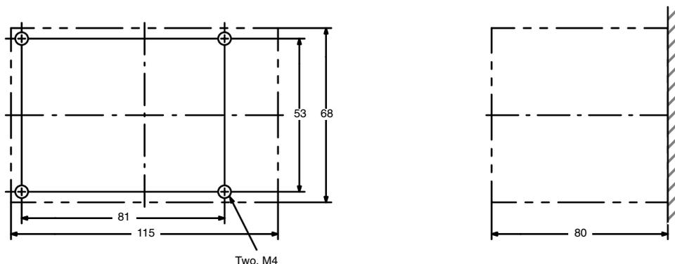
When installing the ID Controller in a control panel, be sure to use plane washers and M4 screws.
