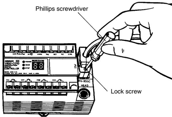
To connect the connector, be sure to hold the housing of the connector, and securely insert the connector. After the connector has been inserted, tighten the two lock screws with a screwdriver.
