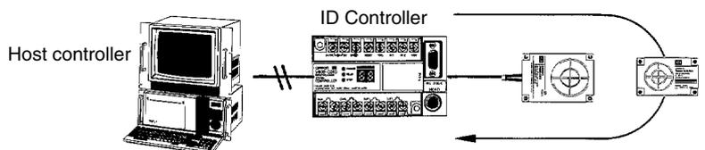
In the TEST Mode, two kinds of tests can be conducted: Read and Write Tests. The Read Test repeatedly reads 1-byte data, while the Write Test repeatedly writes 1-byte data. At this time, however, the contents of the DC's data have not changed. Use this TEST Mode for initial checking of the system.
