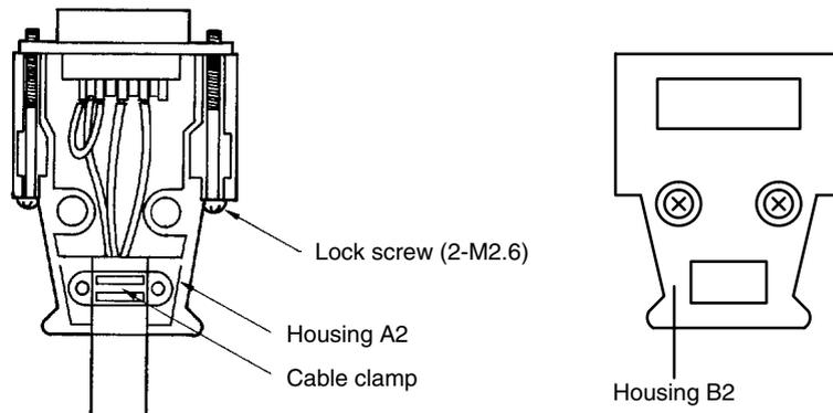
4. Set the two connector tightening screws and attach housing B2 to A2 to complete the connector.
