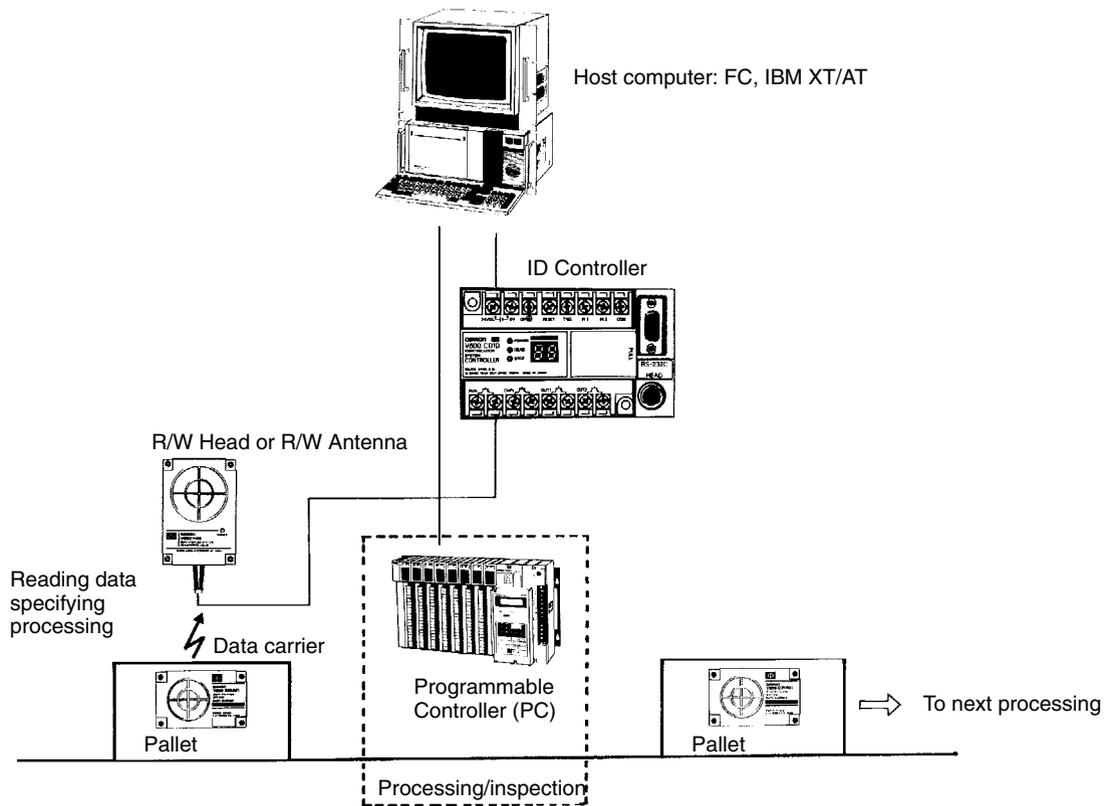
When a command is sent from the host computer (FC, IBM XT/AT compatible) to the ID Controller, the R/W Head (or R/W Antenna) enters the stand-by state, waiting for a signal from the DC.
