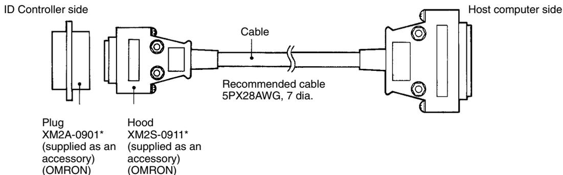
\*Use the accessory connector as the communications connector. Separately prepare the connecting cable and the connector of the host computer. The connector of the ID Controller is made by OMRON and takes countermeasures against EMI.
