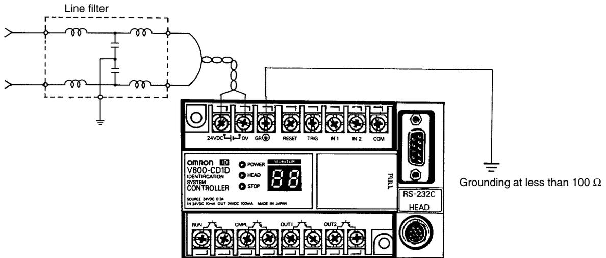
M3.5 screws are used for the Power and ground terminals. In the case of solderless terminals, use the following. Keep the tightening torque to within 8 kg-cm.
