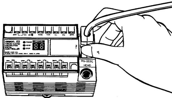
To disconnect the connector, completely loosen the two lock screws, hold the projection of the connector hood with your fingers, and pull the connector straight out, while holding down the Controller with the other hand.
