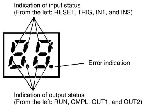
**Note** The Display Mode is set by the internal DIP switch.
