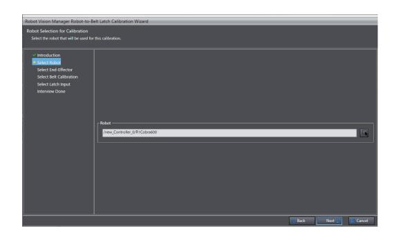
3 Select a robot used for a calibration with the robot selection button. Then click the Next button. The End Effector Selection for Calibration window is displayed.
