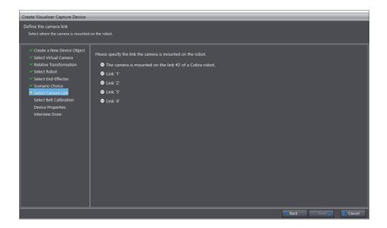
This screen is displayed only when you selected the **mounted on the robot** option for **1)** camera is on the **Scenario Choice** page.
