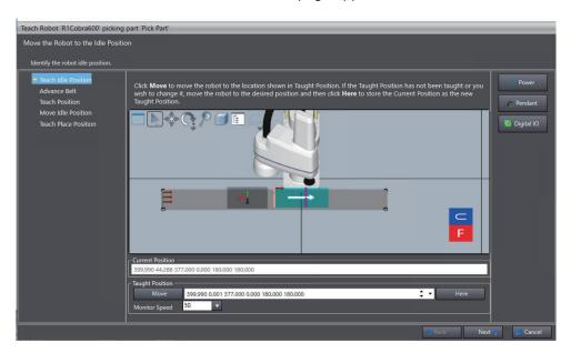
14 Specify a position where the robot stands by until a processing of the part or the part target begins.
