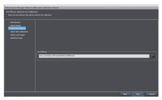
**4** Select an end effector used for the calibration with the end effector selection button. Then click the **Next** button.
