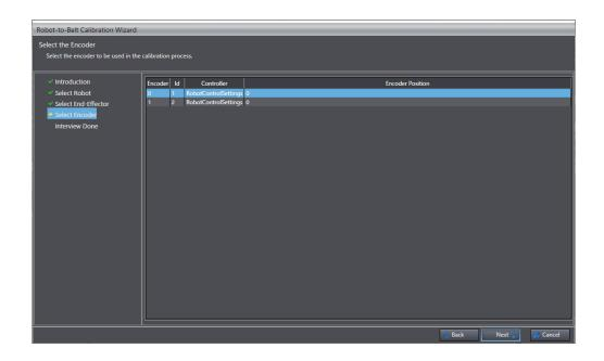
**5** Specify an encoder used in a calibration process, then click the **Next** button. The **Interview Completed** window is displayed.
