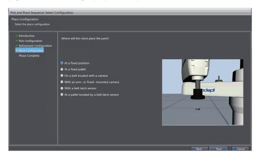
Selecting a Method to Determine Part Placement Position
