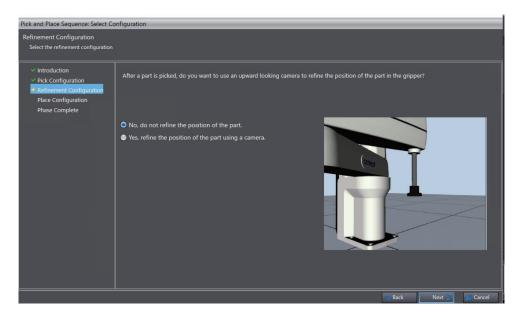
If you want to refine the part position in the gripper with a camera, select the option **Yes, refine the position of the part using a camera**.
