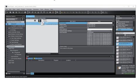
The robot is registered. The registered robot is displayed under **Configurations and Setup** – **Robot Control Setup** – **Robot Settings**.
