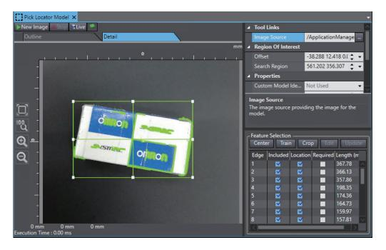
**9** Double-click **Pick Locator** under **Configurations and Setup** in the Multiview Explorer. The **Pick Locator** tab page is displayed.
