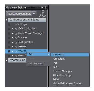
A new Part Buffer object will be added to the Process.
