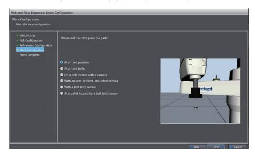
The following methods are available to determine a part placement position.
