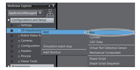
Place the 3D shape data on the possible point where the robot arm may contact, e.g., by the conveyor belt. Refer to *5-4 3D Visualization* on page 5-7 for the details of adding a 3D shape data.
