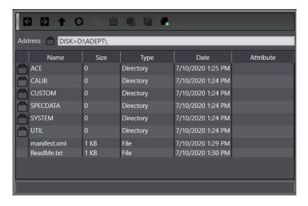
The V+ File Browser works with the Windows clipboard to enable easy transferring of files to and from controllers.
