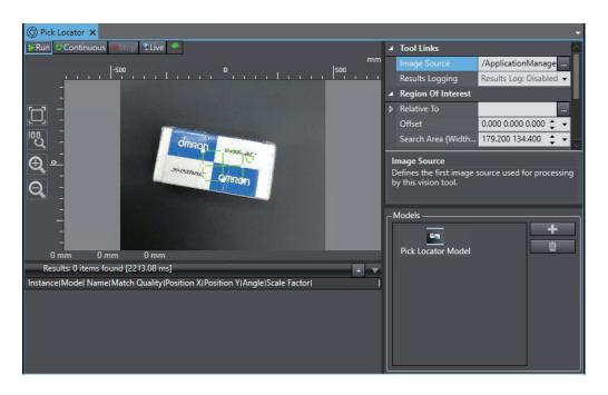
If a Locator Model is not shown, click the add button in **Model**, then select the **Pick Locator Model**.
