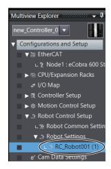
It is necessary to set the cycle of the primary periodic task to 2 ms or more in the task setting when you use a robot. Refer to the *Sysmac Studio Version 1 Operation Manual (Cat. No. W504)* for how to operate the task settings.
