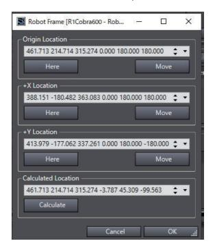
Robot Frames are only available when a part or target object is configured as **Static: Fixed Position** and a Pallet object is defined in that object.
