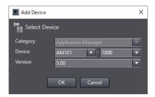
Check the version of the ACE software package running on the IPC Application Controller, and set the Application Manager version of the Sysmac Studio in **Version**, in consultation with the following **Version Information**. You can check the version of ACE from the ACE toolbar or the Help menu.
