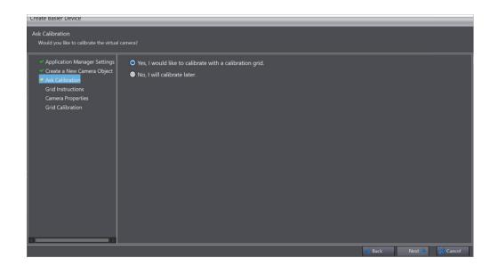
3 Select "Yes, I would like to calibrate with a calibration grid", then click the Next button. If you select "No, I will calibrate later", go to Step 6.
