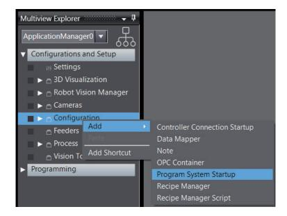
A new **Program System Startup** will be added to **Configuration**.
