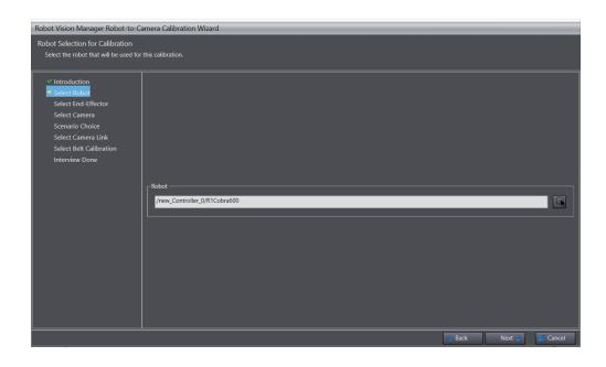
3 Select a robot used for a calibration with the robot selection button. Then click the Next button. The Select End-Effector dialog is displayed.
