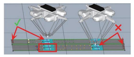
Incorrect belt direction of travel can be corrected by rotating the roll angle of the Belt object 180 degrees to align the direction of belt travel between the Belt object and the associated belt calibrations, and adjusting X and Y position to accurately represent the physical belt in the system. The following figure shows, once corrected, that both robots can process parts as expected. Any parts not processed by the upstream robot can be processed by the downstream robot.
