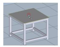
To change the mode of snapping, click the icon and select its function in the following window. Or, press the T + number keys. To close the window, click  $\times$ .
