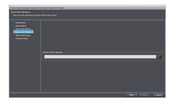
Select a Belt Calibration you want to connect to the latch sensor with the belt calibration selection button. Then click the Next button.
