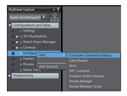
A new Controller Connection Startup will be added to Configuration.
