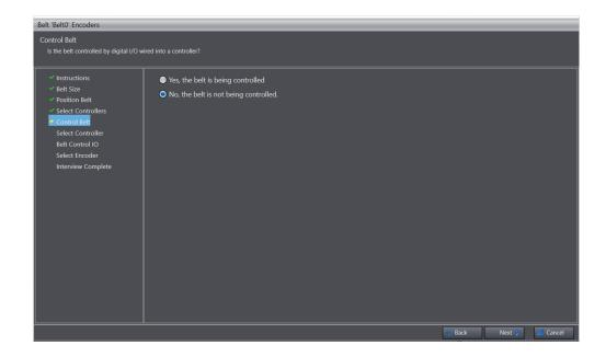
**6** Check the applicable item to see if the belt is controlled by the digital I / O connected to the controller, and click the **Next** button.
