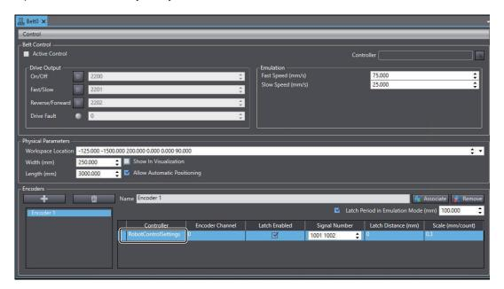
Specify the latch signals used by each camera in the Signal Number field.
