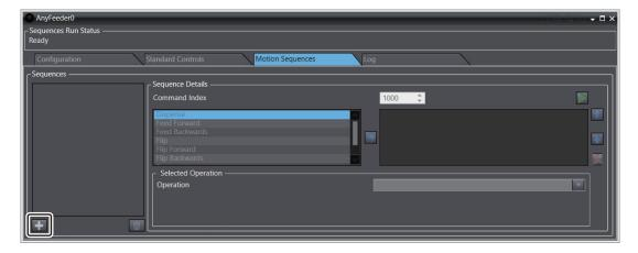
A new sequence will be placed in the sequence list. Adjust the Command Index value if necessary.
