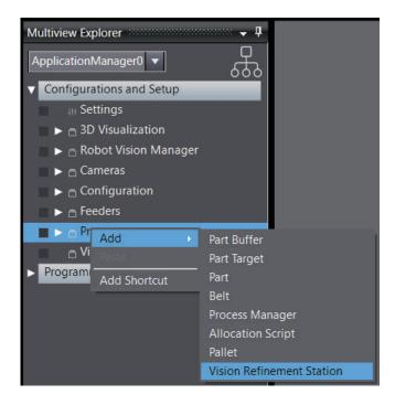
A new Vision Refinement Station object will be added to the Process.
