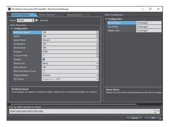
When approach and depart heights are specified, the robot moves in three distinct motions. In the first motion (Approach segment), the robot moves to a location directly above the specified location. For the second motion, the robot moves to the actual location and the gripper is activated. In the third motion (Depart segment), the robot moves to a point directly above the location.
