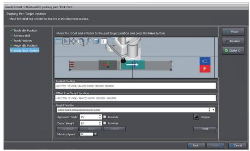
Move the robot's end effector to the part placing point.
