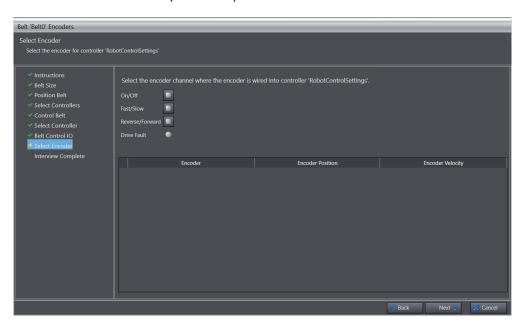
9 Select the encoder channel to connect to the controller and click the Next button. The Interview Complete pane is displayed.
