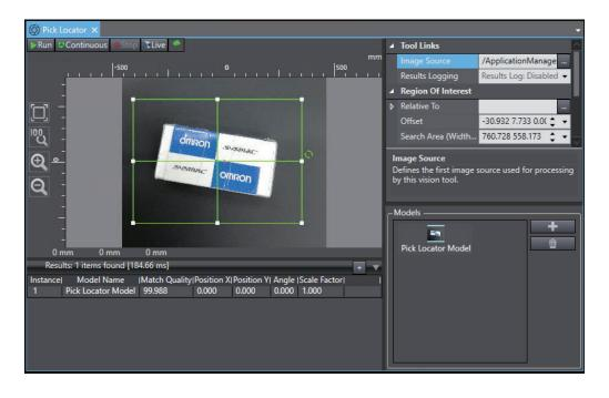
In the same way, detect the locator in other areas and images to test detections.
