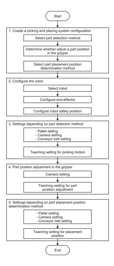
1 Creation of a pick-and-place system configuration To build a pick-and place system configuration, select elements such as part detection method, necessity of part position refinement in the gripper, and method to determine part placement position.
