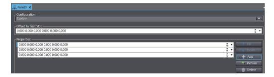
Use the **Add**, **Delete**, **Up** and **Down** buttons to create and arrange each Pallet slot position.
