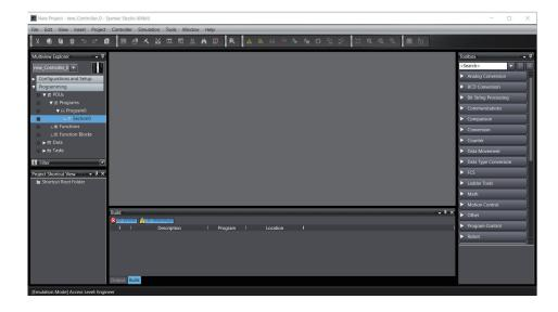
**3** Display the EtherCAT tab page from **Configurations and Setup** in the Multiview Explorer, and register the robot to use.
