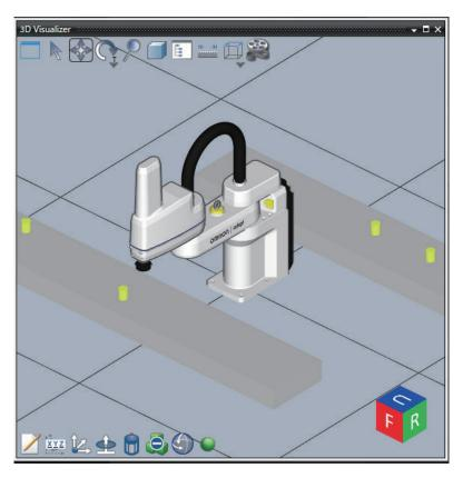
The icons displayed at the lower left of the 3D Visualizer are associated with the objects that you selected in the 3D Visualizer. If no object is selected, these icons are not displayed. Some icons are associated with specific objects as described in the following table.
