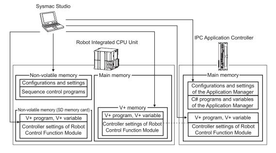
To locate the data as illustrated above, you must transfer settings and programs of the Robot Integrated System with the IPC Application Controller through an online connection to the respective devices. Establish an connection and transfer the data following the procedure described below.
