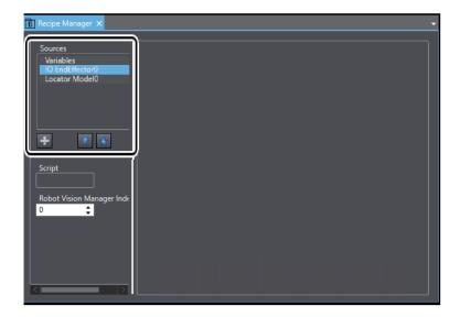
When a data source is added to the Sources list, you can select it to display the settings in the Configuration window. Configuration window options will vary based on the Source type selected. All Source types include settings for the following items.
