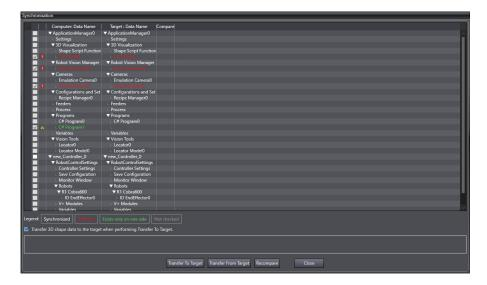
The results of the comparison are displayed as shown below. For V+ Programs, you can display the detailed comparison window.
