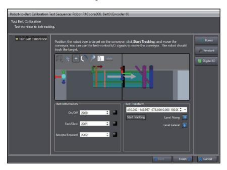
Use the following procedure to test the robot-to-belt calibration.
