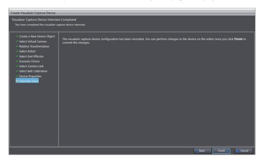
Click the **Finish** button. **Visualizer Capture Device0** is now added under **Configurations and Setup – Cameras** in the **Multiview Explorer**.
