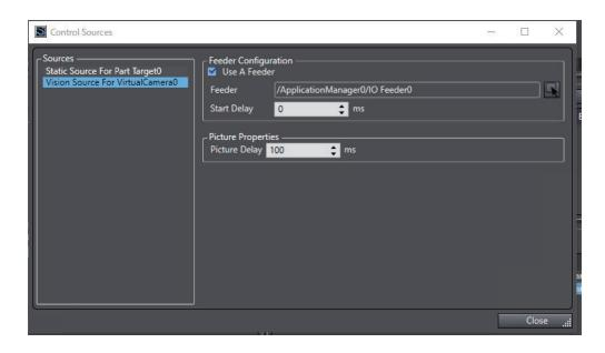
Vision Sources are used for fixed-mounted cameras. They can be associated with IOFeeder objects, similar to Static Sources.
