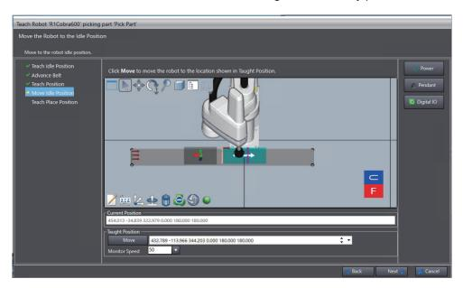
**2** After moving the robot to the registered standby position, click the **Next** button.
