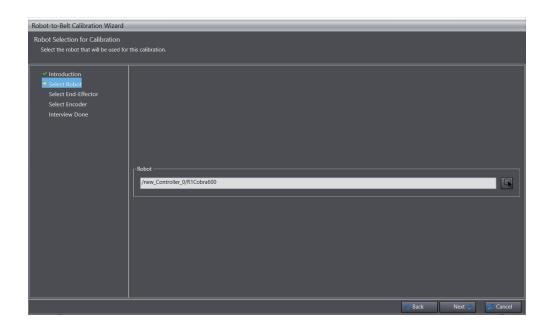
3 Select a robot used for a calibration with the robot selection button. Then click the Next button.
