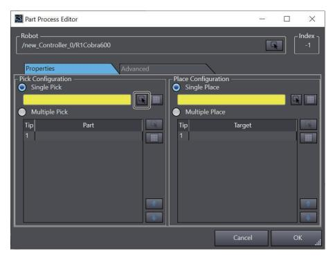
If you want to use a pallet, use the **Pallet Slot Selection** button to select the pallet slots the robot can access for pick or place configurations. This button is only available when a Pallet object is configured for the selected part / target.
