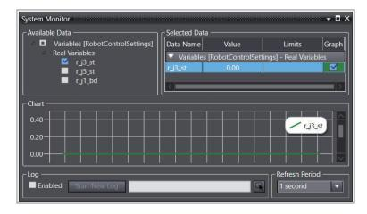
4 Select the folder in which to save a log in the **Log** area and check the Enabled box. Then click the **Start New Log** button.
