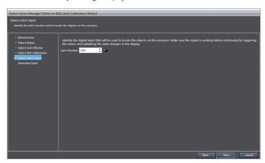
**6** Enter a latch signal number of the encoder used for latch input in the **Latch Number** field. Then click the **Next** button.
