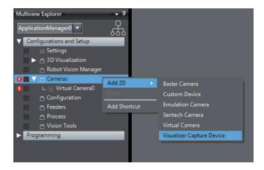
The **Create Visualizer Capture Device** wizard starts and the **Create a New Device Object** page is displayed.
