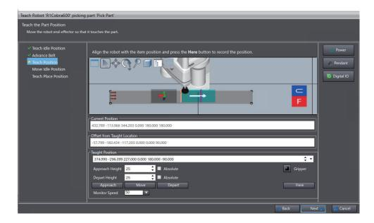
**17** Move the robot's end effector to the part.
