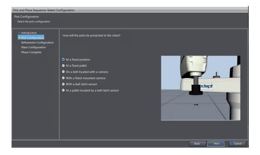
**3** Select **On a belt located with a camera** to detect parts on the conveyor belt with a fixed camera.
