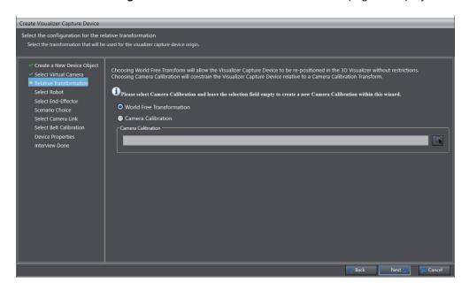
Selecting the **World Free Transformation** option directly brings you to the **Device Properties** page. Selecting the **Camera Calibration** option allows you to use a pre-set camera calibration. If you select **Camera Calibration** with the **Camera Calibration** field left empty, a new calibration camera will be created.
