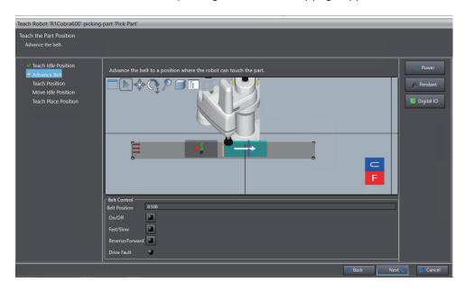
Move the belt as the part approaches to the robot's moving range by clicking the **ON/OFF**, **Fast/Slow**, and **Forward/Reverse** buttons.
