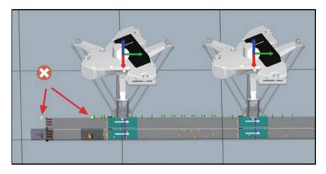
Instead, the sensors should be close together, as shown in the figure below. It is normal for there to be a small deviation due to differences between physical assemblies and ideal positions in 3D visualization.
