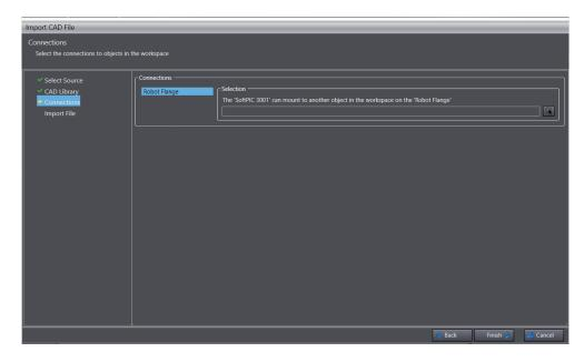
**4** To connect a CAD file 3D shape data to an existing 3D shape data, select a target 3D shape data, then click the **Finish** button.
