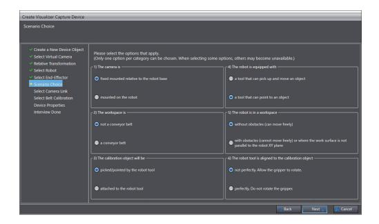
Select options for categories 1 to 6 in order and then click the Next button. Here, for 1) The camera is, select the mounted on the robot option.
