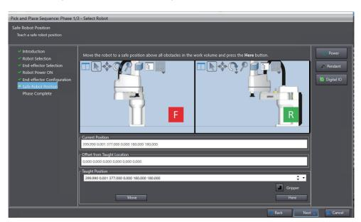
You can modify a robot position by clicking and dragging the robot in the robot view area.
