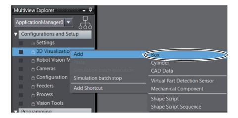
A box or a cylinder is added and displayed under **3D Visualization** in the Multiview Explorer.
