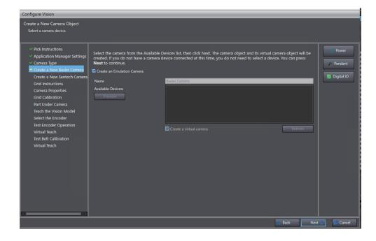
4 Confirm that the Create an Emulation Camera box is checked, then click the Next button. The Select Encoder dialog is displayed.
