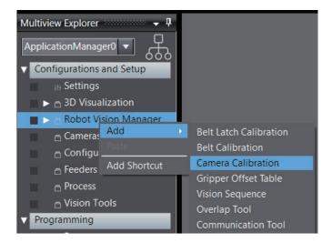
Robot Vision Manager Robot-to-Camera Calibration Wizard will open.
