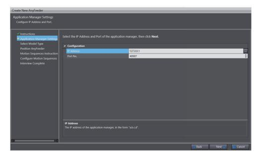
**3** Provide the IP address and port of the Application Manager, then click the **Next** button. The **Select Model Type** window is displayed.
