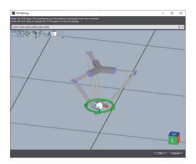
Enter the coordinate values or drag the TCP in the dialog box to specify the position. The TCP setting values are X, Y, Z, y (yaw), p (pitch), and r (roll), from left to right.
