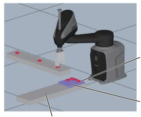
The parts that come in contact with the pallet are "picked" by the pallet and follow the pallet's movement.
