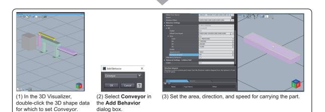
Enter the mechanical component settings that define what motion the mechanical component will give to the part.
