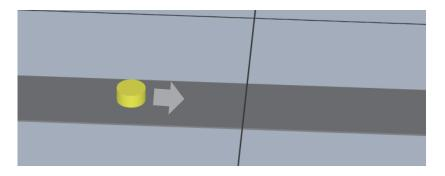
If you set the execution interval to 50 ms, the conveyor belt speed is 100 mm/s, so the part is drawn to move 5 mm on the 3D Visualizer.
