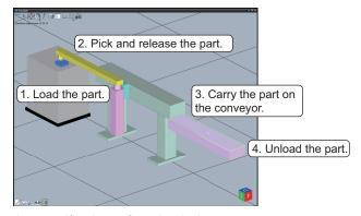
Operation specifications of mechanical components considered in the equipment design phase
