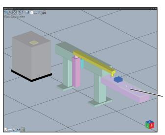
The slider moves and releases the part on a box simulating the conveyor.
