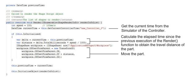
Executing the script causes the part on the 3D Visualizer to move on the conveyor belt.
