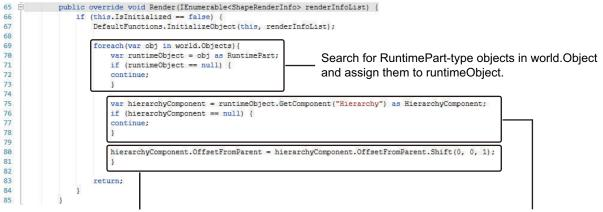
Move the object hierarchyComponent corresponding to the part identified in the above processing by 1mm in the Z direction. Get "Hierarchy", which is an attribute of a part object in RuntimeObject, as a key and assign it to hierarchyComponent.
