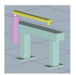
To import CAD data for movable part that consists of a base, an X-axis slider, a Z-axis slider, and an arm with a rotary axis as the mechanical component *X-Y table (XY Theta)*, create a CAD data file for each of the base, X-axis slider, Z-axis slider, and arm with a rotation axis. (In this example, Z axis is applied to the Y axis of the X-Y table (XY Theta).)
