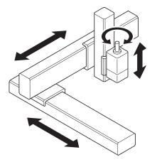
For the X-Y-Z stage + rotation axis (upward direction) model, set the following parameters.
