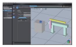
A virtual equipment model consists of a *mechanical component*<sup>\*1</sup> that represents a movable part of the equipment, a *part* that represents the target to be carried, and a *Virtual Part Detection Sensor* that detects the part.
