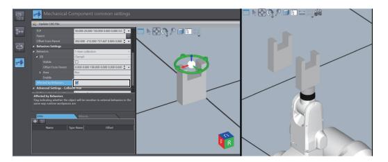
The tool will operate by following the master plate when it enters the area of the master plate set by the *Clamp* Behaviors Settings and the *Clamp* Behaviors Settings are enabled.
