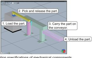
Operation specifications of mechanical components considered in the equipment design phase
