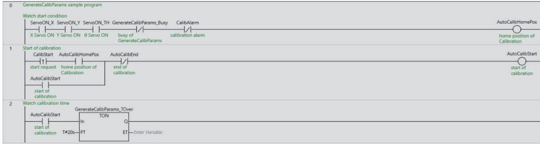
This circuit in the alignment control sample programming is a common circuit for both the Motion Control Function Module of the CPU Unit and the Fault Monitoring circuit of the EtherCAT Master Function Module.
