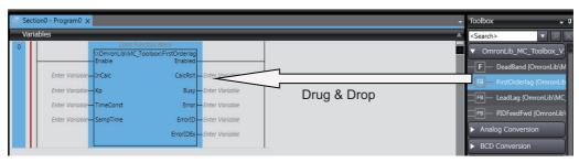
• Right-click the programming editor, select **Insert Function Block** in the menu, and enter the fully qualified name (\\name of namespace\name of function block).
