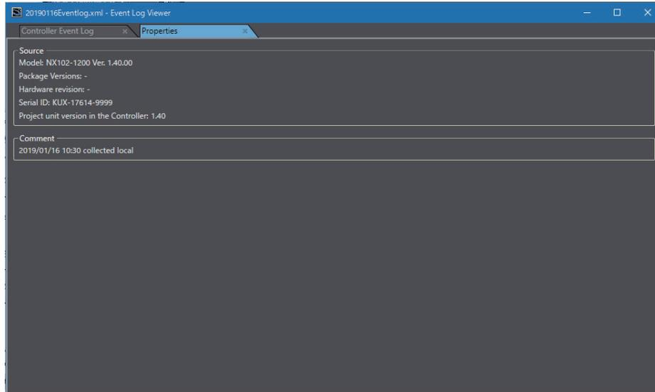
The controller information and comments when the controller event logs were obtained are displayed in the **Properties** Tab.
