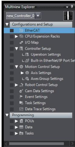
The focus moves to the Configurations and Setup item or Programming item for the selected shortcut.
