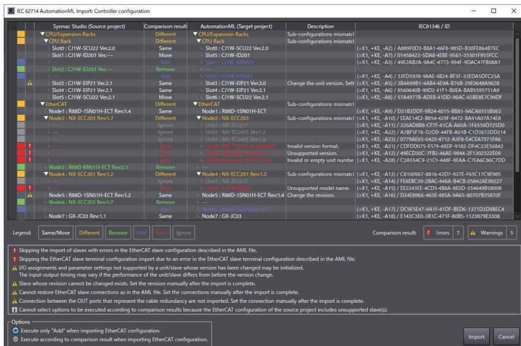
**5** In **Options**, select the import option and then click the **Import** Button. The import of the controller configuration and device variables is executed.
