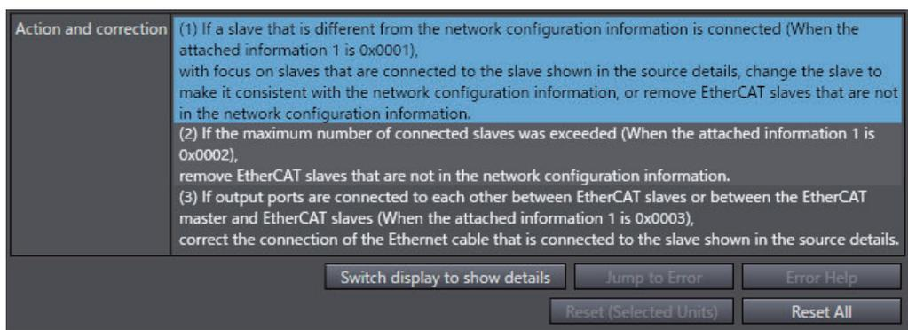
If you select a correction that allows you to jump to the Correction View, the **Jump to Error** Button is enabled.
