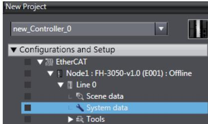
The Setup Tab Page for the scene or system data is displayed in the Edit Pane. Make all of the required settings. Refer to the *Vision System FH/FHV Series Operation Manual for Sysmac Studio (Cat. No. Z343)* for the setup procedures.
