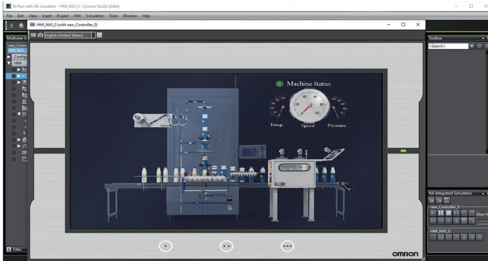
The Simulation Pane has a button that is used dedicatedly for simultaneous simulation of the Controller with an NA-series PT. Refer to *Dedicated Window for Simultaneous Simulation with NA-series PT* on page 7-116 for information on this pane.
