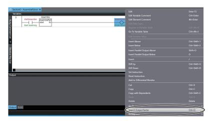
The ladder diagram rung that includes the target of the output factor search is displayed on the Search Output Factor Tab Page.
