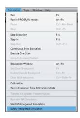
When a safety integration simulation is in progress, the device list in the MultiView Explorer displays only the Controller and Safety CPU Unit being simulated. Perform offline debugging by switching the device as needed.
