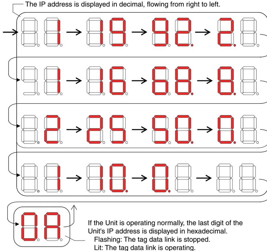
If an error occurs, the error code will be displayed alternately with the rightmost byte of the affected device's IP address. For details on error codes, refer to *Section 15 Troubleshooting*.
