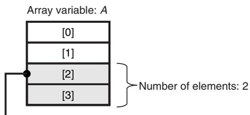
If the service data (*ServiceDat*) is *Array[2]* and number of elements (*Size*) = 2, *Array[2]* and *Array[3]* are sent.
