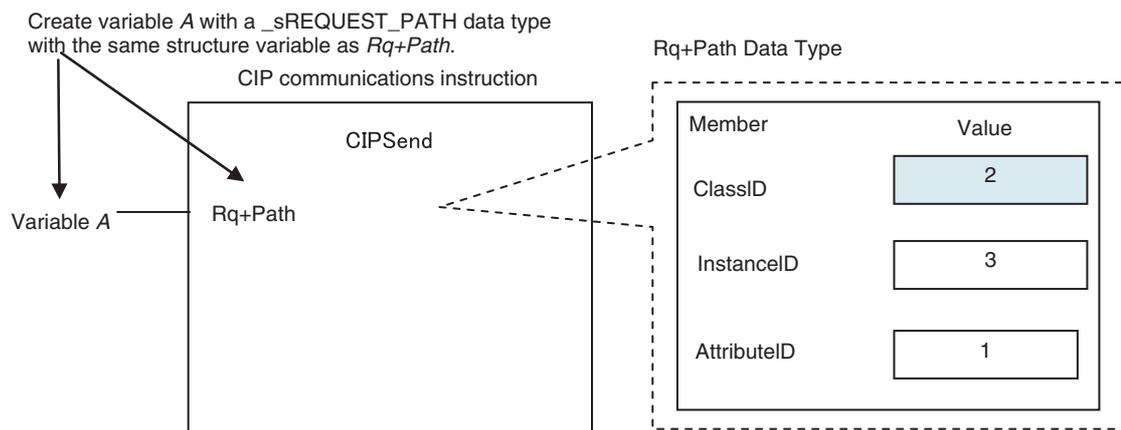
To create a variable in a variable table, select the pre-registered CIP communications instruction data type `_sREQUEST_PATH`. This is a structure variable with the same configuration as *Rq+Path*.
