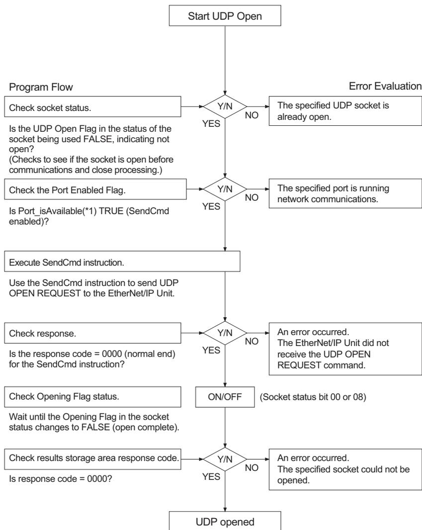
(\*1) \_Port\_isAvailable is a system-defined variable for the Controller to determine whether or not SendCmd is enabled. Refer to the *NJ/NX-series CPU Unit Software User's Manual* (Cat. No. W501) for details.
