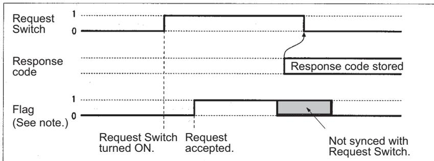
**Note** The Sending Flag and Receiving Flag will not be changed to TRUE if the high-speed socket service option is selected. Therefore, the program can be controlled only by changing the Send Request Switch and Receive Request Switch to FALSE.
