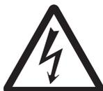
The triangle symbol indicates precautions (including warnings). The specific operation is shown in the triangle and explained in text. This example indicates a precaution for electric shock.
