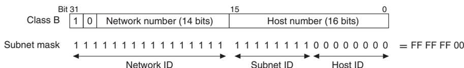
Set the same subnet mask for all of the nodes on that subnetwork. The EtherNet/IP Unit supports CIDR (Classless Inter-Domain Routing). The subnet mask can be set to 192.0.0.0 to 255.255.255.252. If subnetworks are not used, set the following subnet mask values for IP address classes A to C.
