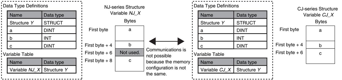
To align the memory configurations in the NJ-series and CJ-series CPU Units, offsets are set in the Sysmac Studio.
