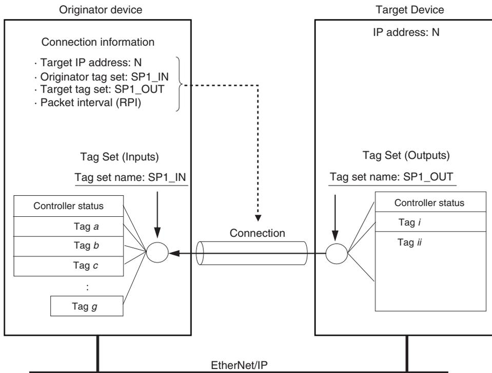
There are both input (consume) and output (produce) tag sets. Each tag set can contain only input tags or only output tags. The same input tag cannot be included in more than one input tag set.
