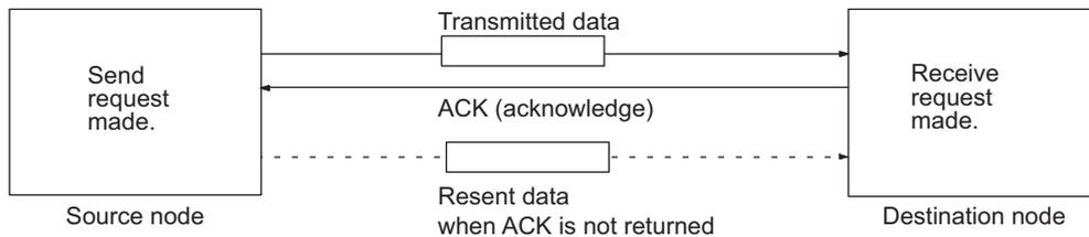
With the TCP protocol, the remote IP address and remote TCP port number are specified when an open request is made for a socket. When a send request is made, the number of bytes to send and the send data are specified.
