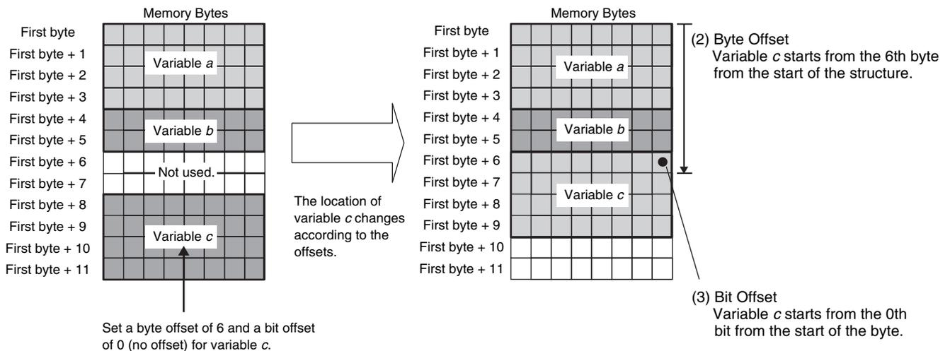
● **Method 2: Changing the Memory Configuration of the Structure Variable in the Remote Device**
