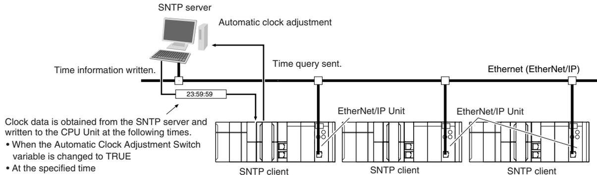
**Note** In accordance with SNTP protocol specifications, automatic adjustment will not be possible from February 7, 2036. This function will no longer operate in the EtherNet/IP Unit from February 7, 2036 (an error message will not be displayed).
