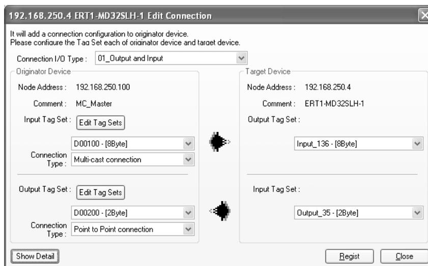
The connection I/O type list box in the upper part of the Connection Settings Dialog Box displays the connection I/O types that can be selected. Select the connection I/O type according to your application.
