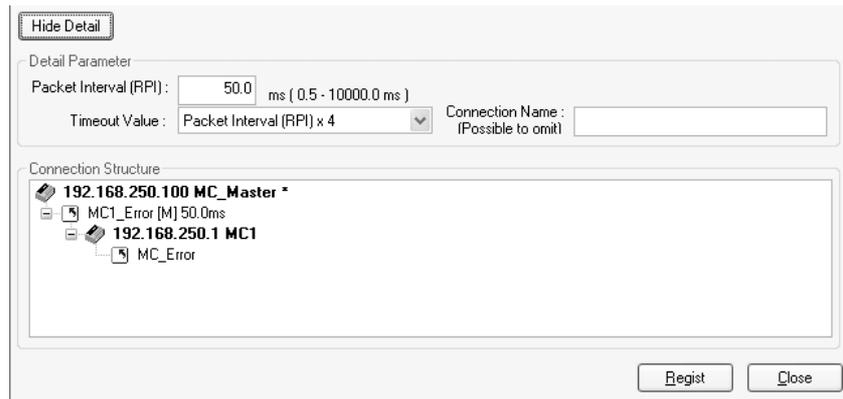
The specified values for detailed parameters will be displayed. Change the values as required. Connection names are automatically created using the following rule.
