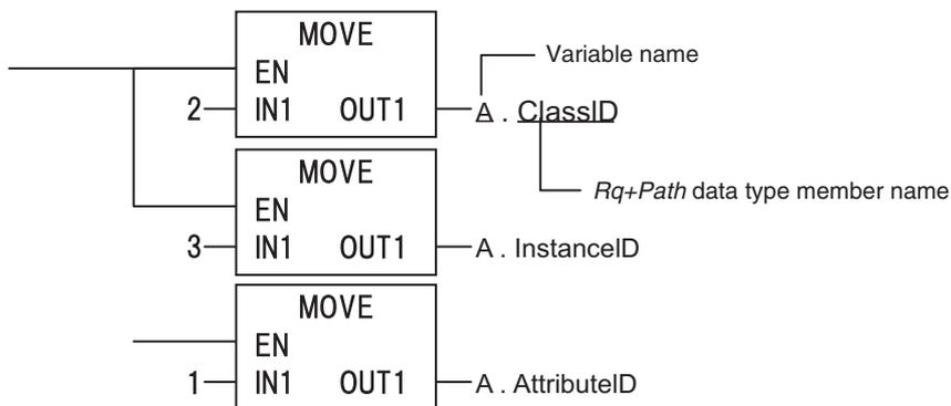
**Preparing Array Variables to Input and Output Service Data and Response Data**
