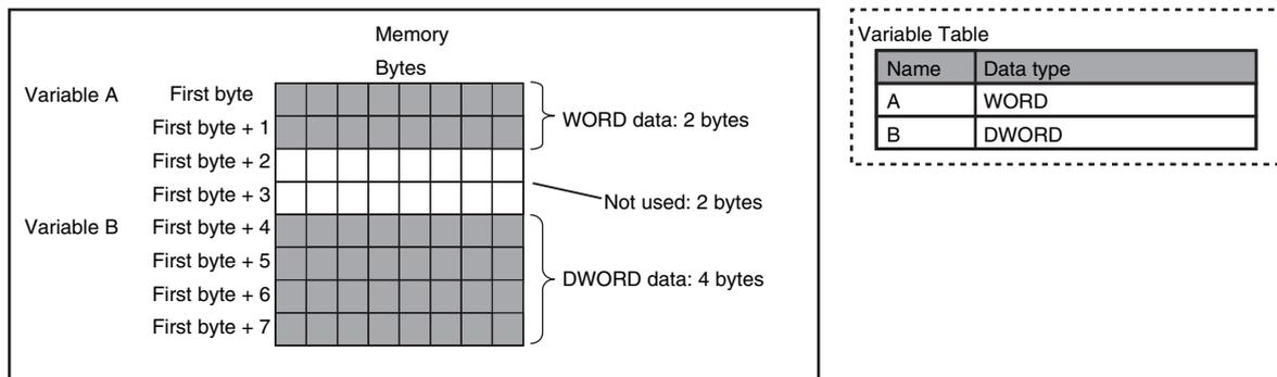
This information for determining the location of a variable in memory is called the alignment. The alignment is determined for each data type. The amount of memory and the memory locations for the variables are given below.
