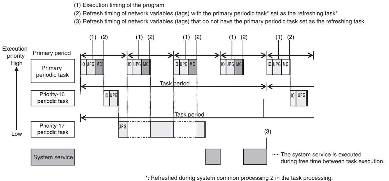
\*: Refreshed during system common processing 2 in the task processing.
