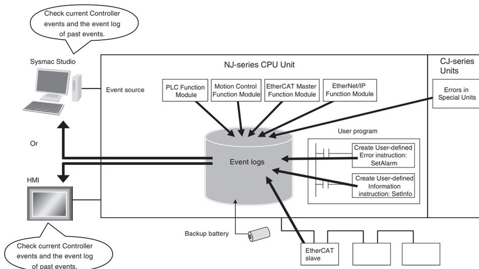
To use an HMI to check events, connect the HMI to the built-in EtherNet/IP port on the CPU Unit.
