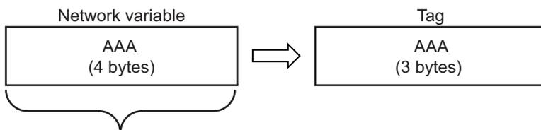
The CPU Unit memory is consumed in units of two bytes. To assign tags of odd numbers of bytes to network variables, specify even byte numbers (i.e., sizes of the tags + 1) to the network variables.
