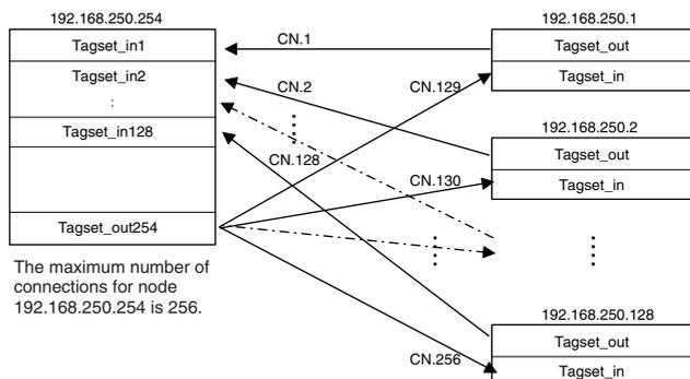
An EtherNet/IP Unit must be mounted to the Controller to increase the maximum number of connections. (Refer to the following figure.)
