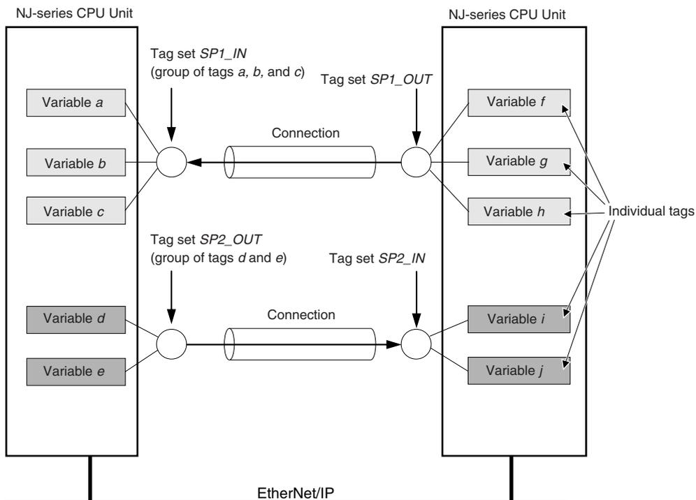
**Note** To enable a connection, each tag set must include only input tags or only output tags. (Both input and output tags cannot be included in the same tag set.)
