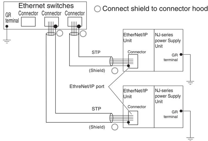
b) Connecting the shields on the Ethernet switch side only
