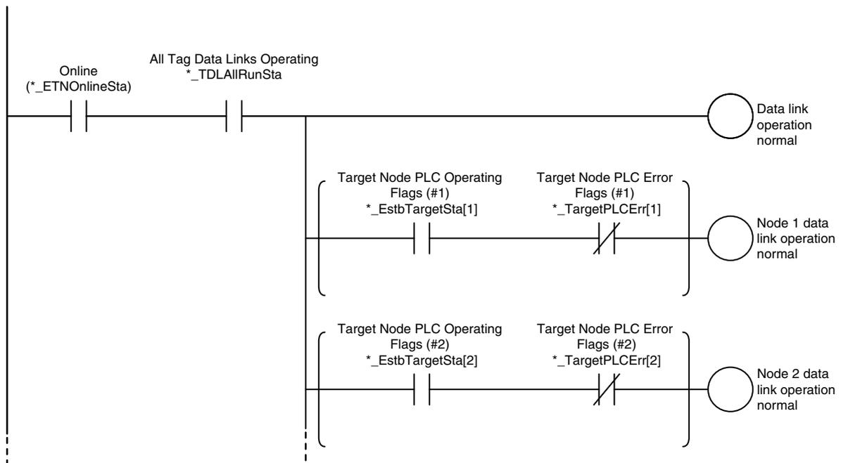
● **Programming Example to Detect Errors**
