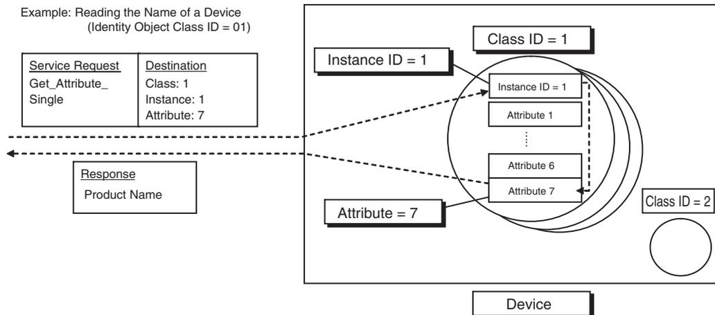
These are called Internal Object Identifiers (IOI) because they identify the Class ID, Instance ID, and Attribute ID within the device. Refer to 8-3 CIP Objects Sent to the EtherNet/IP Unit for the class ID, instance ID, attribute ID, and service code for each object.
