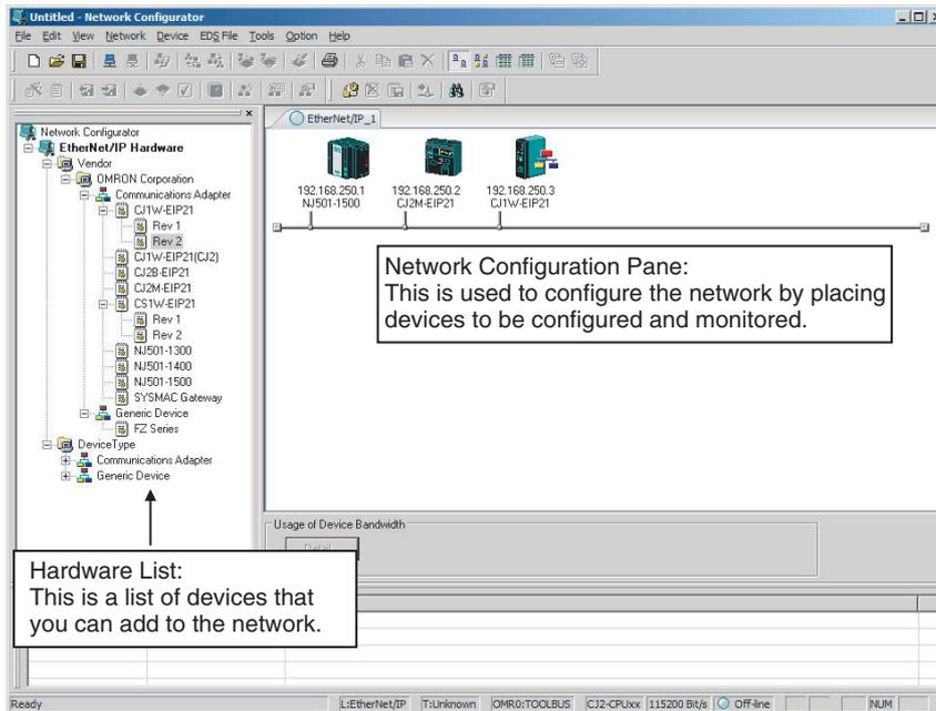
To manage two or more networks, you can select **Network – Add** to add a new Network Configuration Pane. You can add a new Network Configuration Pane.
