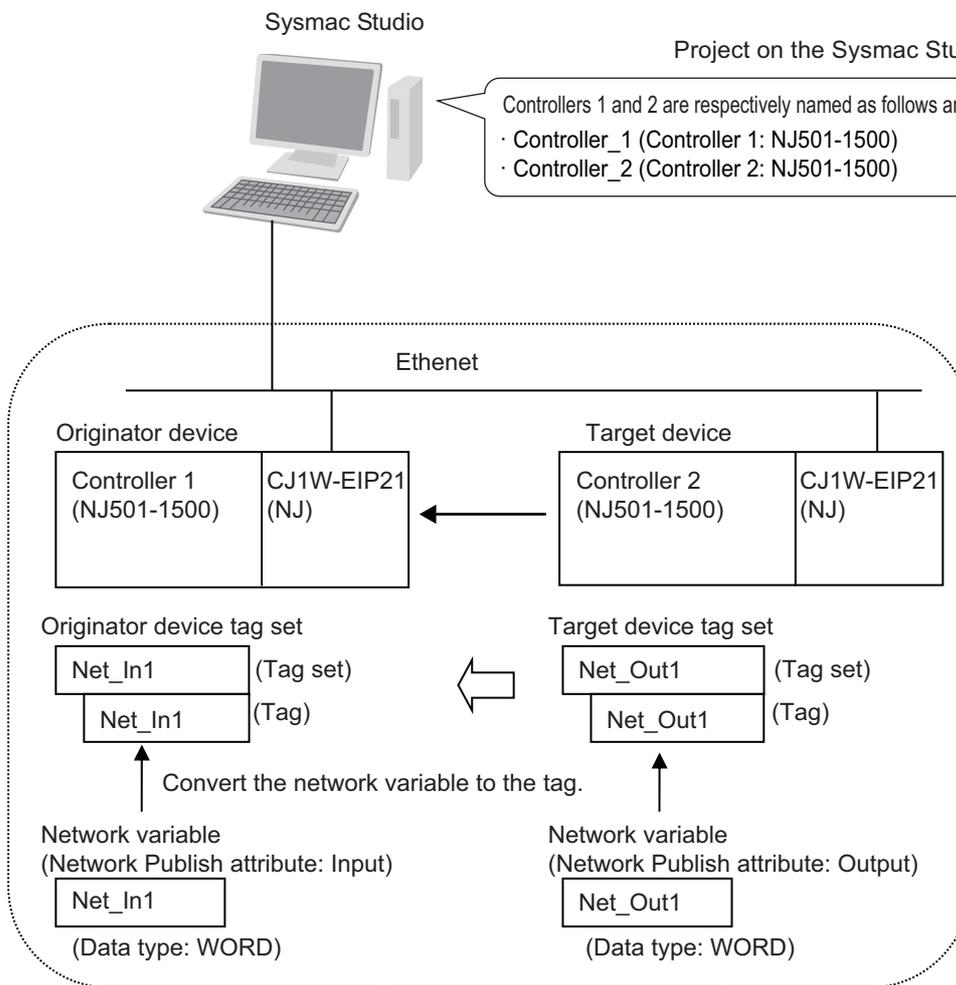
Follow the flow below to set the settings to Controllers 1 and 2 for which to establish EtherNet/IP connections.
