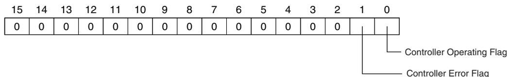
To receive the Controller status, specify the Controller status for the In - Consume Tab Page in the dialog box used to edit the receive tag set. (Select the *Include* Option for the *Controller Status* in the upper right of the Edit Tag Set Dialog Box.) When a tag data link is started, the contents of the Controller status is stored in the device variables for the CJ-series Unit that are given below.
