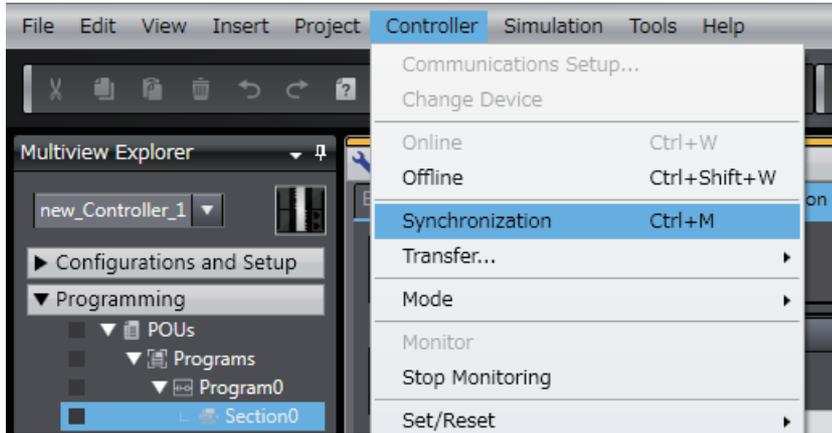
The Synchronization Window is displayed, and comparison of the user program and parameter settings between the Sysmac Studio and the Controller is started.
