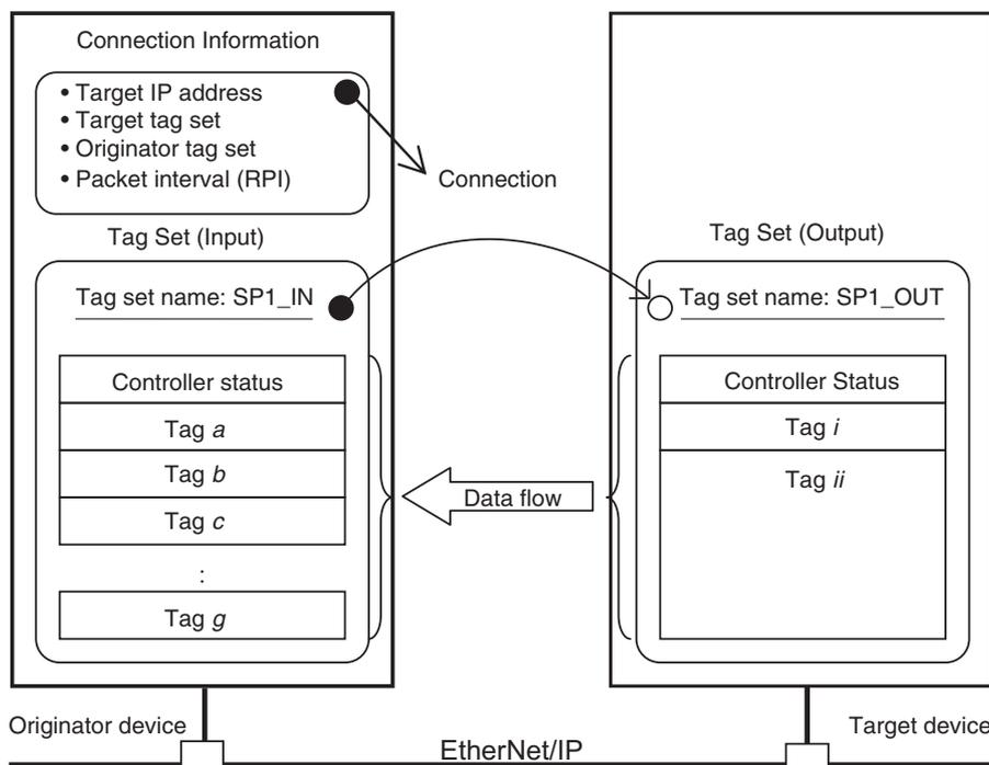
\* In this example, a connection is established with the originator's tag list with tags a to g (inputs), which are in a tag set called SP1\_IN, and the target's tag list with tags i and ii (outputs), which are in a tag set called SP1\_OUT.
