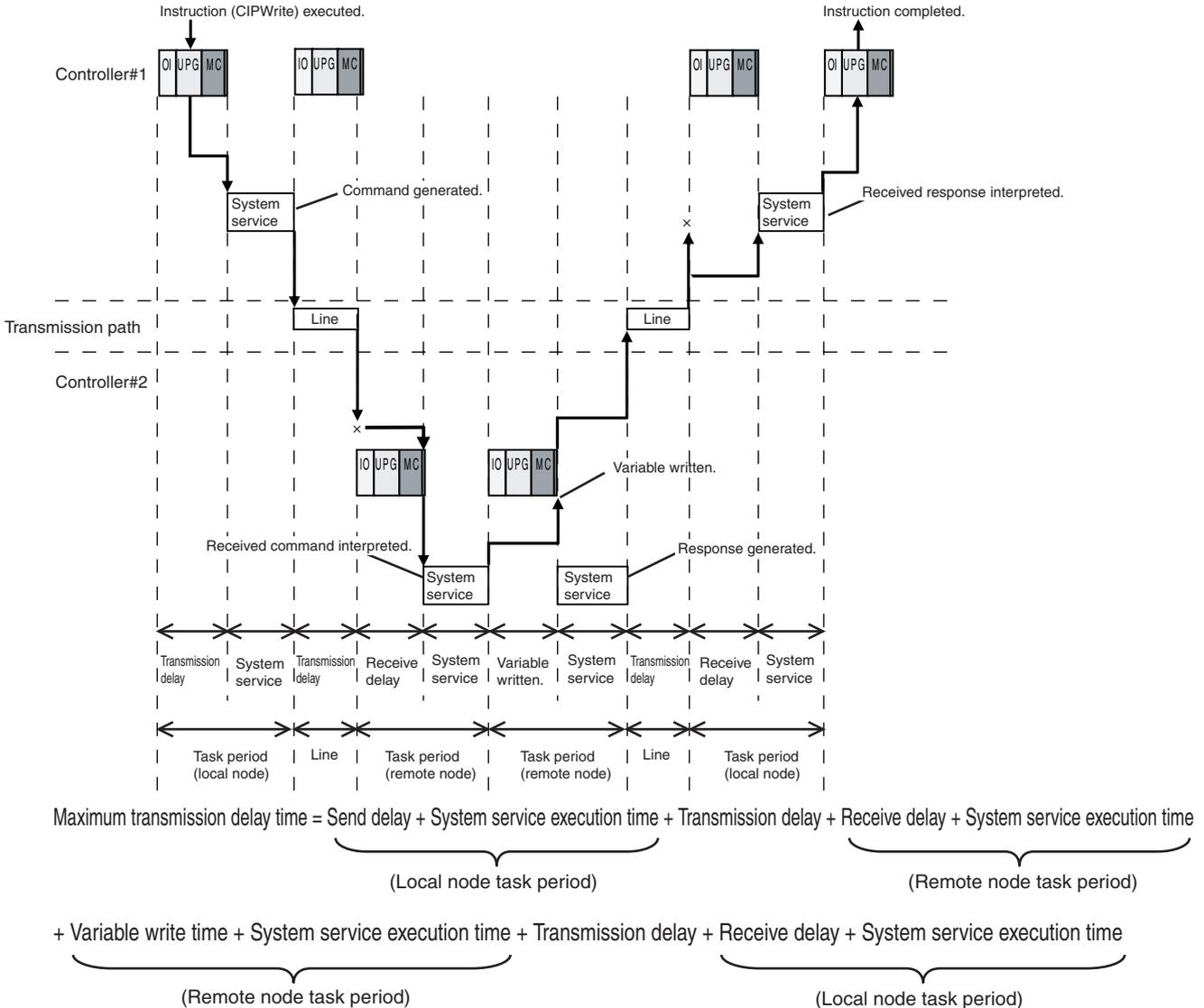
Processes that cause a delay time are processed in the task periods at each node as shown in the above diagram. Line-based delays are as follows:
