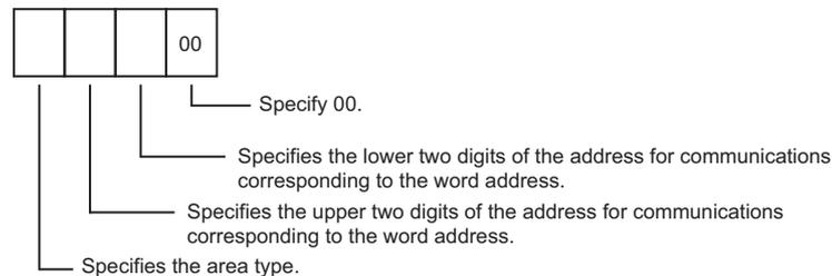
For the area type and the address for communications corresponding to the word address, the specification method is the same as described in *Send/Receive Data Address* (on page 13-22).
