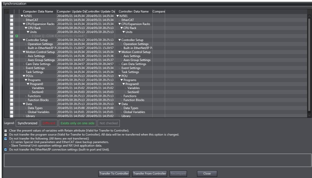
**3** Clear the *Do not transfer the EtherNet/IP connection settings (built-in port and Unit)* Check Box and click the **Transfer to Controller** Button. Then the EtherNet/IP connection settings are transferred along with the not-synchronized data. If no EtherNet/IP connection settings are set in the Sysmac Studio, no data will be sent.
