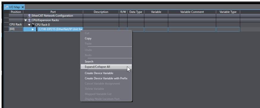
The I/O ports in the target replacement model CJ1W-EIP21S are expanded.
