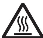
The triangle symbol indicates precautions (including warnings). The specific operation is shown in the triangle and explained in text. This example indicates a precaution for high temperatures.
