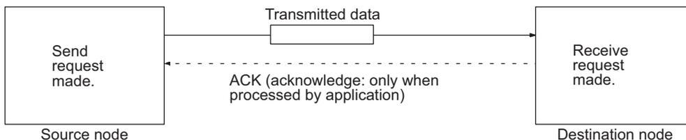
With the UDP protocol, the remote IP address and remote UDP port number are not specified when an open request is made for a socket. When a send request is made, the remote IP address, the remote UDP port number, the number of bytes to send, and the send data are specified.
