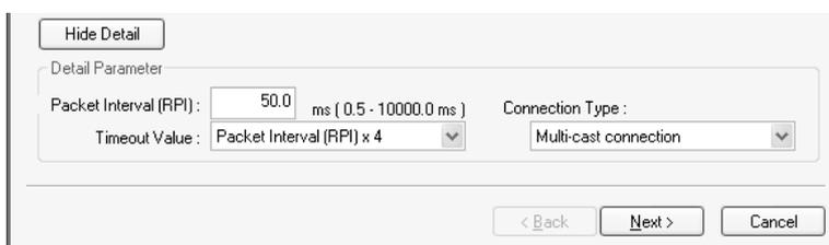
The specified values for detailed parameters will be displayed. Change the values as required. The connection name cannot be set. They are automatically created using the following rule. default\_N (where N is a 3-digit number (001, 002, etc.) starting from 1)
