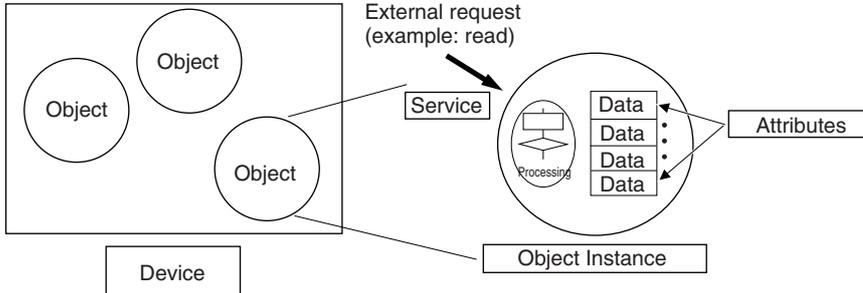
In the CIP Common Specification, “Object,” “Class,” “Instance,” “Attribute,” and “Service” are defined as follows: (Source: CIP Common Specification)
