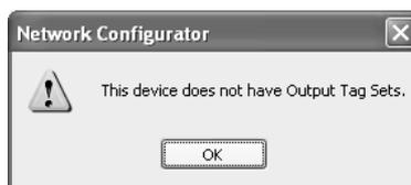
Before dropping again, refer to the manual of the applicable device and create the I/O data (i.e., output tag sets) required to create a connection.
