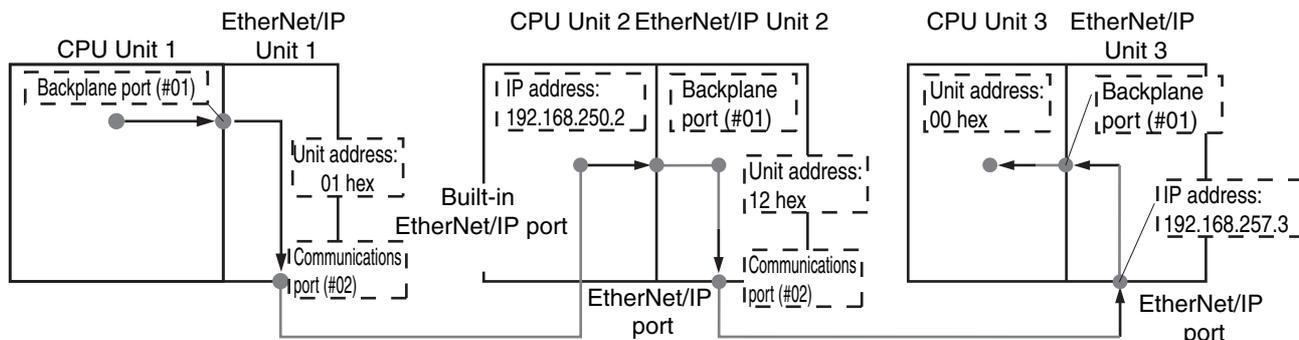
**(1) CPU Unit 1 to EtherNet/IP Unit 1**
