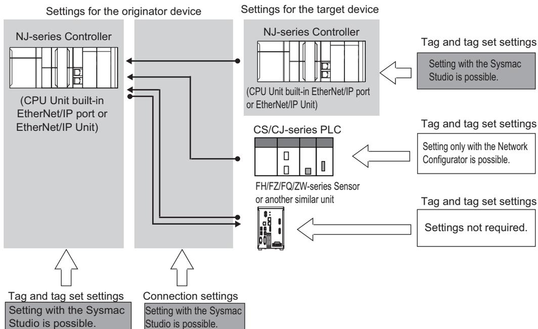
Use the Network Configurator if a CS/CJ-series PLC operates as the originator device.
