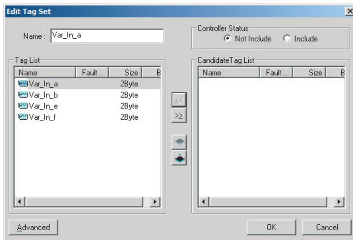
You can register up to eight tags in a tag set. (If you include the Controller status in the tag set, you can register up to only seven tags, and two bytes are added to the size.)
