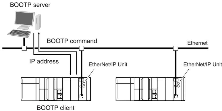
The EtherNet/IP Unit IP address is obtained from the BOOTP server when the power is turned ON.
