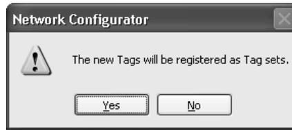
If the **No** Button is clicked, more tags can be registered at the end of the tag set. Refer to step 18 for details on adding tags to the end of the tag set.
