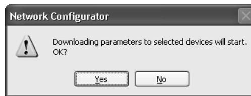
3. Click the **Yes** Button to download the tag data link parameters to the EtherNet/IP Unit.
