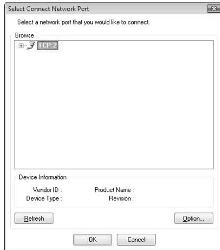
The Network Configurator will connect to the EtherNet/IP network, and “On-line” will be displayed in the status bar at the bottom of the window when connection has been properly made online.
