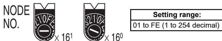
The left switch sets the sixteens digit (most significant digit) and the right switch sets the ones digit (least significant digit). The node address is factory-set to 01.
