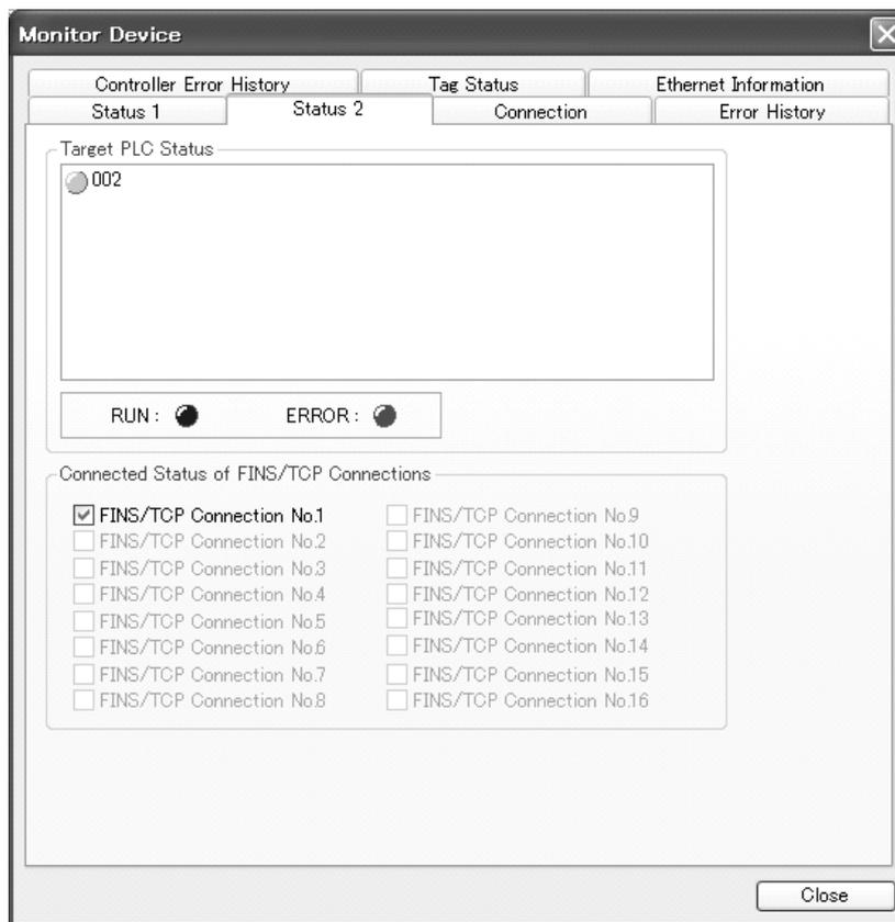
**Note** The target PLC status can be used when the PLC status is selected for all the target sets for both originator and target connections. For those that are not selected, the status will be grayed-out.
