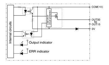
When overcurrent is detected, the ERR indicator will light, and the corresponding flag in the Basic I/O Unit Information Area (A050 to A069) will turn ON.
