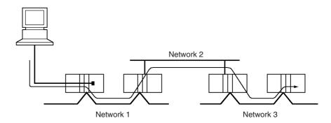
**Note** With CS/CJ-series CPU Units Ver. 2.0 or later, remote programming/monitoring is possible up to 8 levels away. Refer to 1-7-2 *Improved Read Protection Using Passwords* for details.
