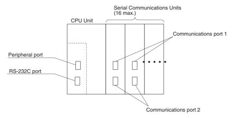
Expanding the system configuration as shown above allows a greater number of serial communications ports, and greater flexible and simpler support for different protocols.
