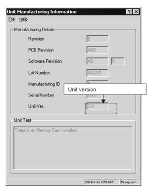
Use the above display to confirm the unit version of the CPU Unit connected online.
