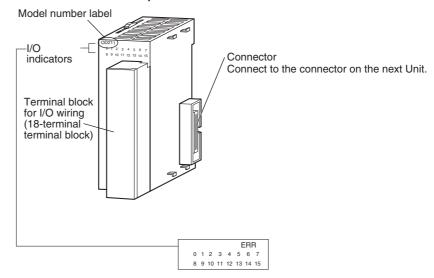
**Note** The CJ1W-OD202, CJ1W-OD204, and CJ1W-OD212 also have an ERR indicator for the load short-circuit alarm.
