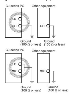
Do not share the PLC's ground with other equipment or ground the PLC to the metal structure of a building. The configuration shown in the following diagram may worsen operation.
