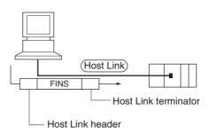
Note In Host Link mode, FINS commands contained between a header and terminator can be sent from the host computer to any PLC on the Network. Communications are possible with PLCs on the same or different types of interconnected Networks up to two levels away (three levels including the local level but not including the Host Link connection).
