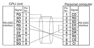
D-Sub, 9-pin connector Male connector on cable D-Sub, 9-pin connector Female connector on cable
