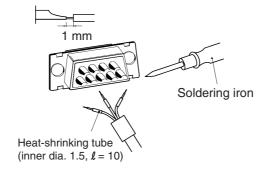
4. Move the heat-shrinking tubes onto the soldered area and shrink them into place.
