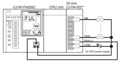
Connect the negative terminal of the 24-VDC power supply to the Input Unit common (COM) terminal.
