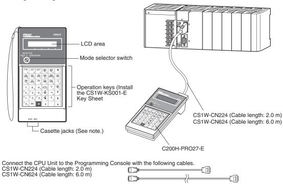
Note The cassette jacks are not used with CJ-series CPU Units.
