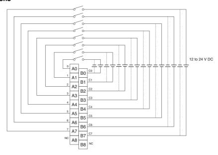
Polarity of the input power supply can be connected in either direction.
