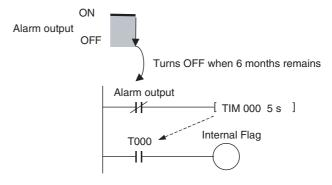
The Flag is programmed to allow for the delay in the alarm output at system startup. The Flag does not turn ON when the alarm output is ON (normal operation). When the alarm output turns OFF (replacement required), the Flag turns ON, and the replacement notification can be monitored from the system.
