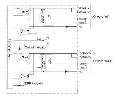
When the output current of any output exceeds the detection current, the output for that point will turn OFF. At the same time, the ERR indicator will light and the corresponding flag (one for each common) in the Basic I/O Unit Information Area (A050 to A069) will turn ON.
