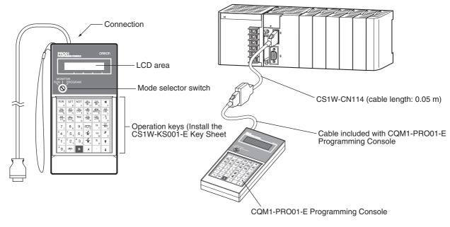
Connect the CPU Unit to the Programming Console with the following cables. CS1W-CN114 (Cable length: 0.05 m)
