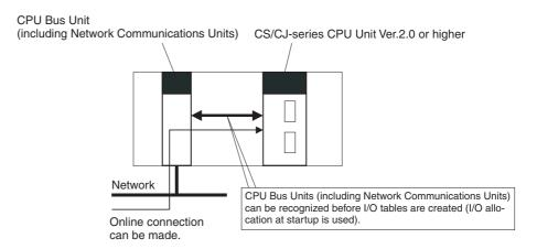
**Note** Network Communications Units include Ethernet Units, Controller Link Units, SYSMAC Link Units, and DeviceNet Units.
