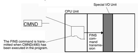
FINS commands can be transmitted to Special I/O Units in other PLCs in the network, not just the local PLC.
