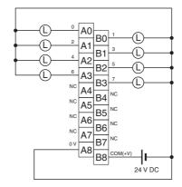
When wiring, pay careful attention to the polarity of the external power supply. The load may operate if the polarity is reversed.
