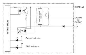
When overcurrent is detected, the ERR indicator will light, and the corresponding flag in the Basic I/O Unit Information Area will turn ON.
