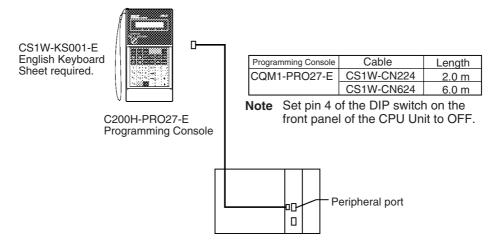
**Note** When an OMRON Programmable Terminal (PT) is connected to the RS-232C port and Programming Console functions are being used, do not connect the Programming Console at the same time.
