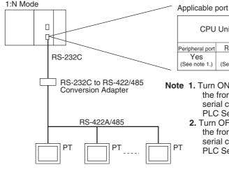
Note 1. Turn ON pin 4 on the DIP switch on the front of the CPU Unit and set the serial communications mode in the PLC Setup for an NT Link.
