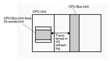
**Note** With CJ1-H CPU Units, the CPU BUS I/O REFRESH instruction (DLNK(226)) can be executed in the ladder program to refresh the CIO Area words allocated to the CPU Bus Unit of a specified unit number.
