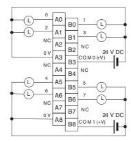
When wiring, pay careful attention to the polarity of the external power supply. The load may operate if the
