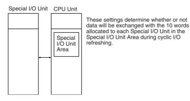
**Note** Whenever disabling a Special I/O Unit's cyclic refreshing, be sure that the I/O for that Unit is refreshed with IORF(097) or FIORF(225) (CJ1-H-R CPU Units only) in the program at least every 11 seconds during operation. A CPU Unit service monitoring error will occur in the Special I/O Unit if it is not refreshed every 11 seconds.
