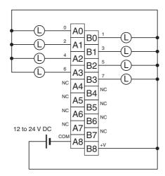
When wiring, pay careful attention to the polarity of the external power supply. The load may operate incorrectly if the polarity is reversed.
