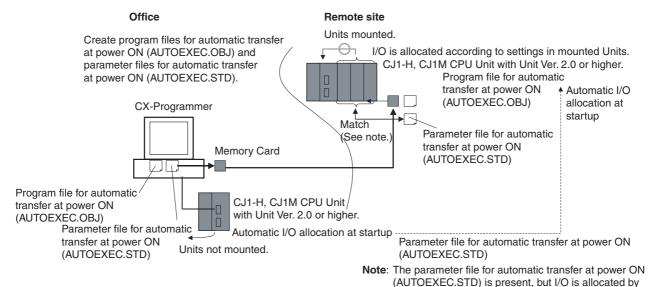
As a result, in the above diagram for example, files for automatic transfer at power ON are created in an office where the Units are not mounted. The files are then saved in a Memory Card, which is taken and installed in a CJ-series CPU Unit at the remote site, where automatic transfer at power ON is executed and I/O is allocated according to the I/O allocations in the mounted Unit using the method recorded in the Memory Card.
