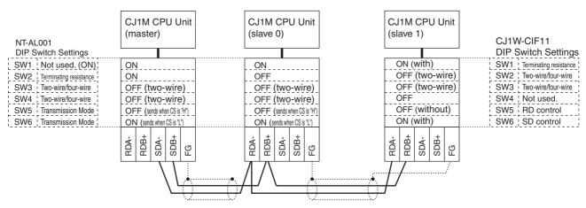
**Note** Refer to *Serial PLC Link Connection Examples (CJ1M CPU Units Only) on page 662* for wiring diagrams and settings when using CJ1W-CIF RS-422A Converters only.
