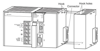
2. The yellow sliders at the top and bottom of each Unit lock the Units together. Move the sliders toward the back of the Units as shown below until they click into place.
