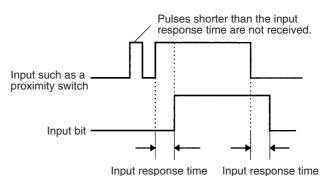
The default setting for the input response time is 8 ms and the setting range is 0 to 32 ms. When the input response time is set to 0 ms, the only delay will be the delays in the Unit's internal elements. For information on the Unit's internal elements, refer to *Appendix A Specifications of Basic I/O Units* and check the input response time for the Unit that you are using.
