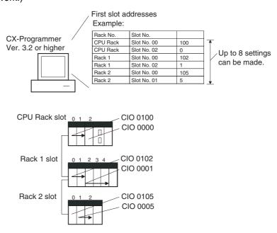
**Note** The first address settings for Racks and slots can be uploaded/downloaded from/to the CPU Unit.
