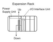
The following diagram shows examples of proper Rack connections. Connect the simple lock connectors to the I/O Control Unit on the CJ-series CPU Rack and the I/O Interface Unit on the CJ-series Expansion Rack.
