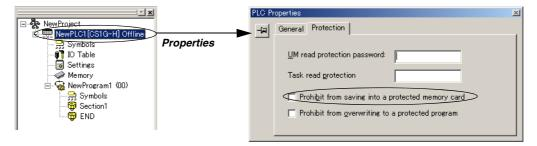
2. Either select *PLC - Transfer - To PLC* to transfer the program or select *PLC - Protection - Set Password* and click the **OK** button.
