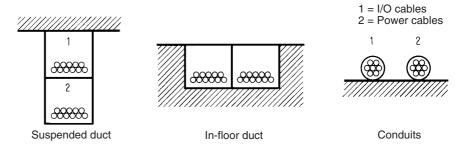
If the I/O wiring and power wiring must be routed in the same duct, use shielded cable and connect the shield to the GR terminal to reduce noise.
