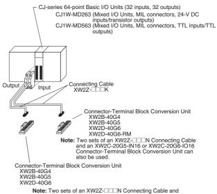
Note: Two sets of an XW2Z-IIIN Connecting Cable and an XW2C-20G6-IO16 Connector-Terminal Block Conversion Unit can also be used.
