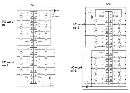
• When wiring, pay careful attention to the polarity of the external power supply. The load may operate if the polarity is reversed.
