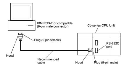
**Note** Use the special cables provided from OMRON for all connections whenever possible. If cables are produced in-house, be sure they are wired correctly. External devices and the CPU Unit may be damaged if general purpose (e.g.,
