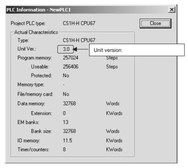
Use the above display to confirm the unit version of the CPU Unit.
