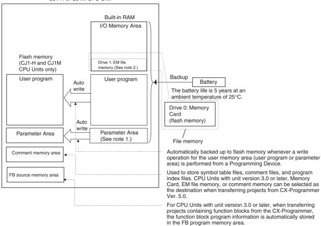
Note 1. The Parameter Area stores system information for the CPU Unit, such as the PLC Setup. An attempt to access the Parameter Area by an instruction will generate an illegal access error.
