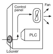
• If a Programming Console will be left on the PLC, the ambient temperature must be within the Programming Console's operating range of 0°C to 45°C.
