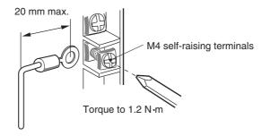
Caution Tighten the AC power supply terminal block screws to the torque of 1.2 N⋅m. Loose screws may result in short-circuit, malfunction, or fire.
