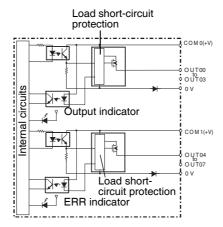
• The ERR indicator will light and the corresponding bit in A050 to A069 (Basic I/O Unit Information, two points per bit) will turn ON if an overcurrent or line disconnection is detected.
