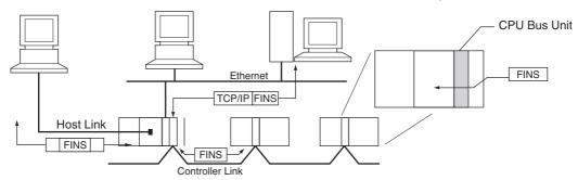
**Note** A TCP/IP header must be attached to the FINS command for an Ethernet Network, and a Host Link header must be attached to the FINS command for a Host Link Network
