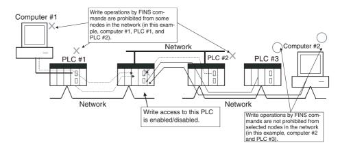
**Note** This function prohibits writing by FINS commands only, so it has no effect on write operations by functions other than FINS commands, such as data links.
