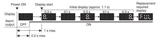
When replacement is already required, the alarm display will follow the initial display. The alarm output will turn ON approximately 0.2 seconds after the power is turned ON, and then turn OFF after approximately 5 seconds.
