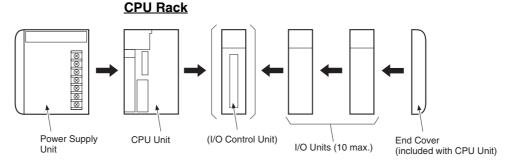
**Note** Connect the I/O Control Unit directly to the CPU Unit to enable connecting Expansion Racks.
