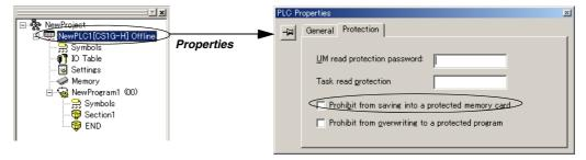
Either select PLC - Transfer - To PLC to transfer the program or select PLC - Protection - Set Password and click the OK button.
