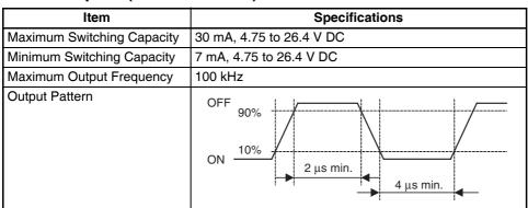
**Note** 1. The load at the above values is taken as the resistance load, and the connecting cable impedance is not taken into account.
