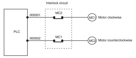
This circuit prevents outputs MC1 and MC2 from both being ON at the same time even if both CIO 000500 and CIO 000501 are both ON, so the motor is protected even if the PLC is programmed improperly or malfunctions.
