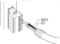
**Note** To remove the signal lines from the connector, press down on the orange tab while pulling out the signal line, as shown in the following diagram.
