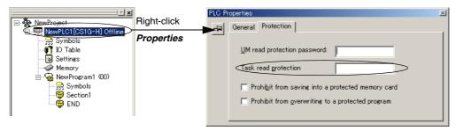
2. Select the tasks that will be password-protected and select the *Task read protect* Option in the *Program Properties* Tab.
