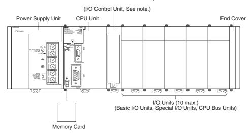
**Note** The I/O Control Unit is required only to connect an Expansion Rack. It must be connected next to the CPU Unit.
