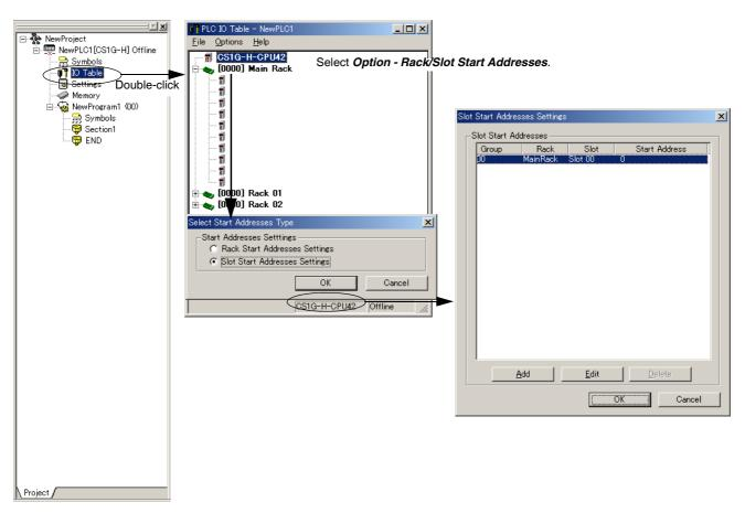
This function can be used, for example to allocate fixed addresses to Input Units and Output Units. (With CQM1H PLCs, input bits are from IR 000 to IR 015 and output bits are from IR 100 to IR 115. First slot addresses can be set when replacing CQM1H PLCs with CS/CJ-series PLCs to reduce conversion work.)
