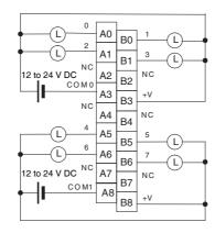
When wiring, pay careful attention to the polarity of the external power supply. The load may operate incorrectly if the polarity is reversed.
