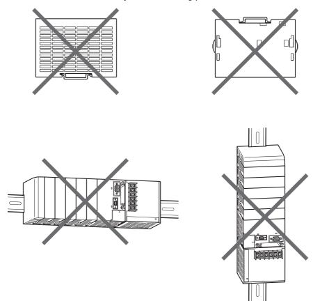
**Note** Always use the standard installation method. A nonstandard installation will decrease heat dissipation, and may delay the replacement notification signal (in particular for Power Supply Units with Replacement Notification), or degrade or damage the internal elements.
