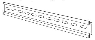
Secure the DIN Track to the control panel using M4 screws separated by 210 mm (6 holes) or less and using at least 3 screws. The tightening torque is 1.2  $N \cdot m$ .
