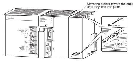
3. Attach the End Cover to the Unit on the far right side of the Rack.
