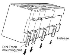
2. Fit the back of the PLC onto the DIN Track by inserting the top of the track and then pressing in at the bottom of the PLC, as shown below.
