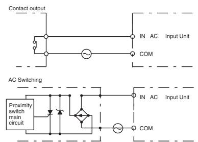
**Note** When using a reed switch as the input contact for an AC Input Unit, use a switch with an allowable current of 1 A or greater. If Reed switches with smaller allowable currents are used, the contacts may fuse due to surge currents.
