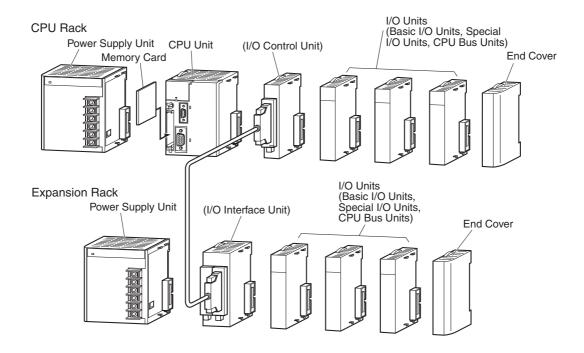
**Note** Although the CJ-series PLCs do not require Backplanes, the term "slot" is still used to refer to the relative position of a Unit in the Racks. The slot number immediately to the right of the CPU Unit is slot 1, and slot numbers increase toward the right side of the Rack.
