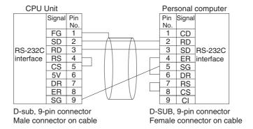
**Note** Refer to *Connection Examples on page 659* when converting between RS-232C and RS-422A/485 to connect multiple nodes. Refer to *Recommended Wiring Methods on page 664* when making your own RS-232C cable.
