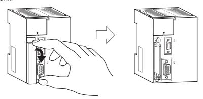
2. Insert the Memory Card with the label facing to the left. (Insert with the  $\Delta$  on the Memory Card label and the  $\Delta$  on the CPU Unit facing each other.)
