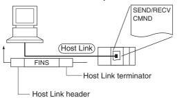
SEND(090): Sends data to the Host computer. RECV(098): Receives data from the Host computer. CMND(490): Executes a specified FINS command.
