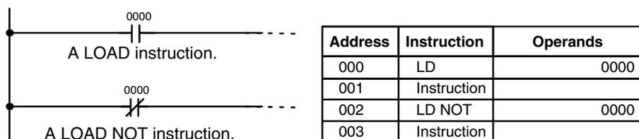
When this is the only condition on the instruction line, the execution condition for the instruction at the right is ON when the condition is ON. For the LOAD instruction (i.e., a normally open condition), the execution condition would be
