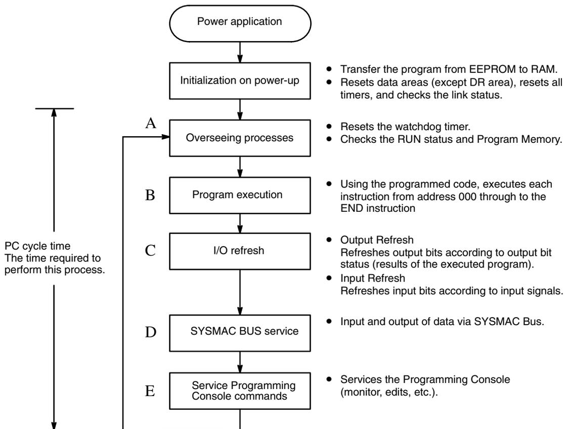
The first initialization process is performed only once, immediately after power is applied to the PC. The remaining operations are performed in cyclic fashion, with each cycle forming one cycle. The cycle time is the time that is
