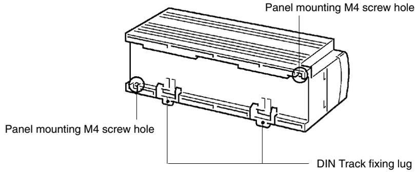
**Note** Install the SK20 such that the heat radiation from top of the unit is not restricted. Leave the plastic seal on the top surface of the unit in place during installation and wiring to prevent dust and foreign matter from entering the unit. The plastic seal must be removed after installation and wiring are complete. If it is not removed after the Unit is installed, the plastic seal will cause the Unit to overheat during operation.
