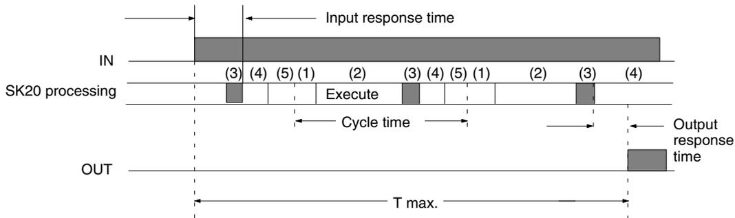
$$\text{Maximum response time} = \text{Input response time} + \text{Filter value} + (\text{Cycle time} \times 2) + \text{Output response time}$$
