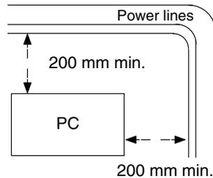
Whenever possible, use wiring conduit to hold the I/O wiring. Standard wiring conduit should be used, and it should be long enough to completely contain the I/O wiring and keep it separated from other cables.
