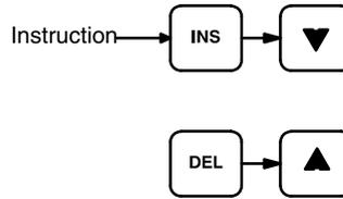
When an instruction is inserted or deleted, all addresses in Program Memory following the operation are adjusted automatically so that there are no blank addresses and no unaddressed instructions.
