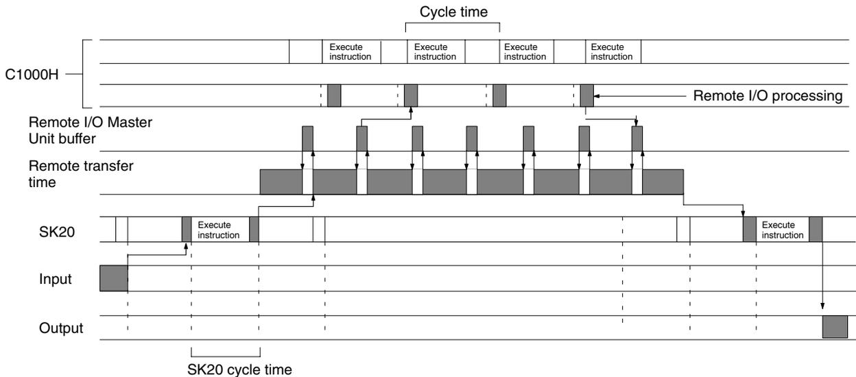
If C1000H cycle time exceeds SYSMAC BUS transfer time
