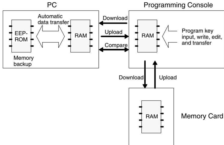
**Note** New Memory Cards must be initialized before data can be stored. Be sure to format Memory Cards before use. Placing a 18th program on the memory card will inhibit rewriting operations; do not store more than 17 programs per card. If the size of the DR area is changed after programming operations have been started or the program code accesses illegal addresses, program transfer cannot be performed and the message “???” will be displayed on the Programming Console.
