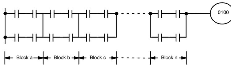
The following diagram requires an OR LOAD followed by an AND LOAD to code the top of the three blocks, and then two more OR LOADS to complete the mnemonic code.
