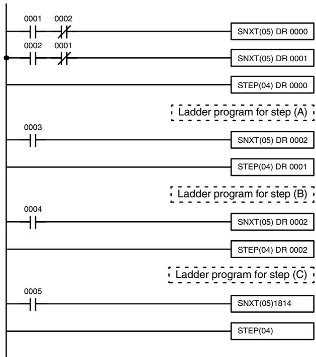
The upper-right program is used if steps (A) and (B) cannot be executed simultaneously. If steps (A) and (B) can be executed simultaneously, delete 0002 (LD NOT) and 0001 (LD NOT).
