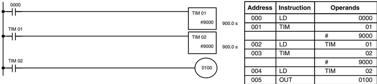
In this example, bit 0100 will be turned ON 30 minutes after bit 0000 goes ON.
