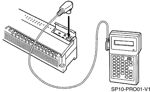
**Connecting Cable** Use one of the following Connecting Cables to connect the Programming Console.
