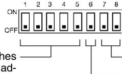
When using SYSMAC BUS, set switches SW1 to SW5 to allocate the remote I/O addresses.
