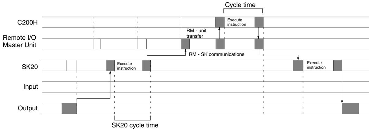
If C200H cycle time exceeds SYSMAC BUS transfer time
