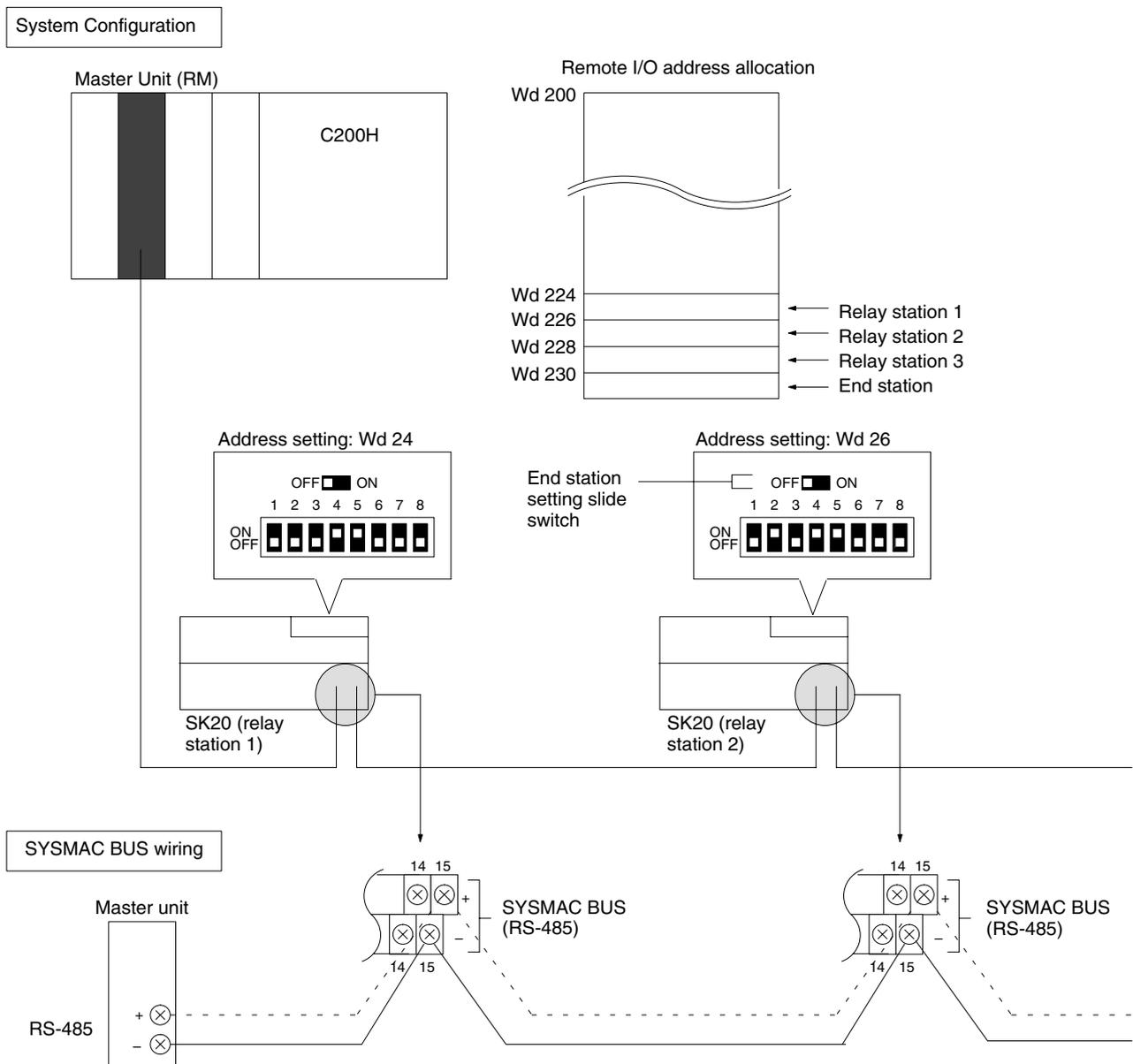
The connecting cables should be made of the recommended cable (VCTF0.75 x 2C).
