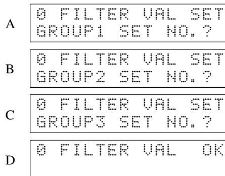
Set the filter values of groups 1, 2, and 3 at the same time. After entering the filter values, read them on the Programming Console for confirmation. Use the following key sequence. Reading is possible in either RUN or PROGRAM mode.
