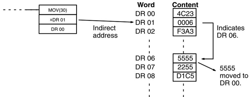
When using indirect addressing, the address of the desired word must be in BCD and it must specify a word within the DR area. In the above example, the content of \*DR 00 would have to be in BCD and between 0000 and 0015.
