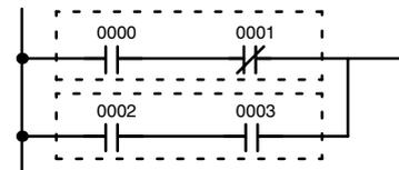
**Description** When instructions are combined into blocks that cannot be logically combined using only OR and AND operations, AND LD and OR LD are used. Whereas AND and OR operations logically combine a bit status and an execution condition, AND LD and OR LD logically combine two execution conditions, the current one and the last unused one.
