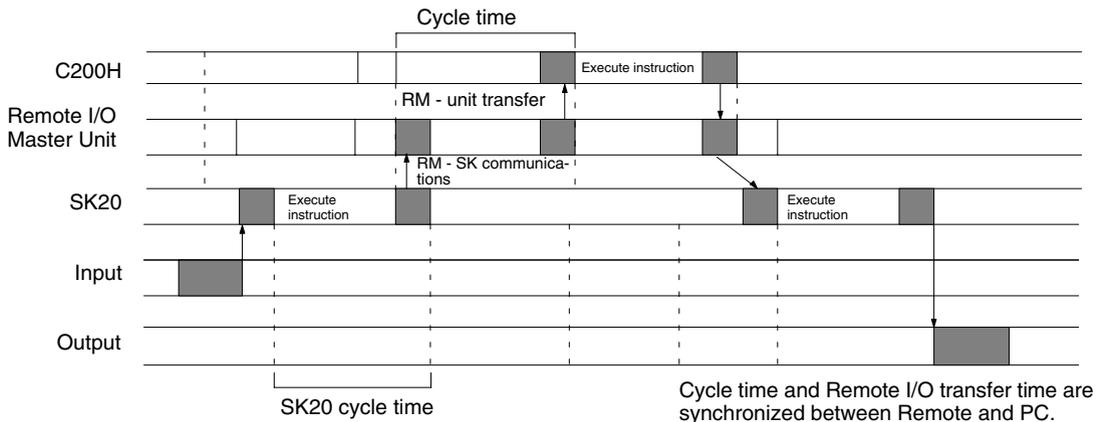
If C200H cycle time exceeds SYSMAC BUS transfer time
