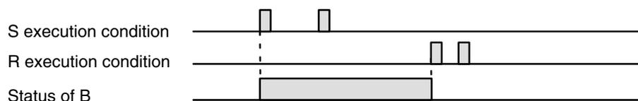
KEEP(12) operates like the self-maintaining bit described in 3-6-5 *Self-maintaining Bits (Seal)*. The following two diagrams would function identically, though the one using KEEP(12) requires one less instruction to program and would maintain status even in an interlocked program section.
