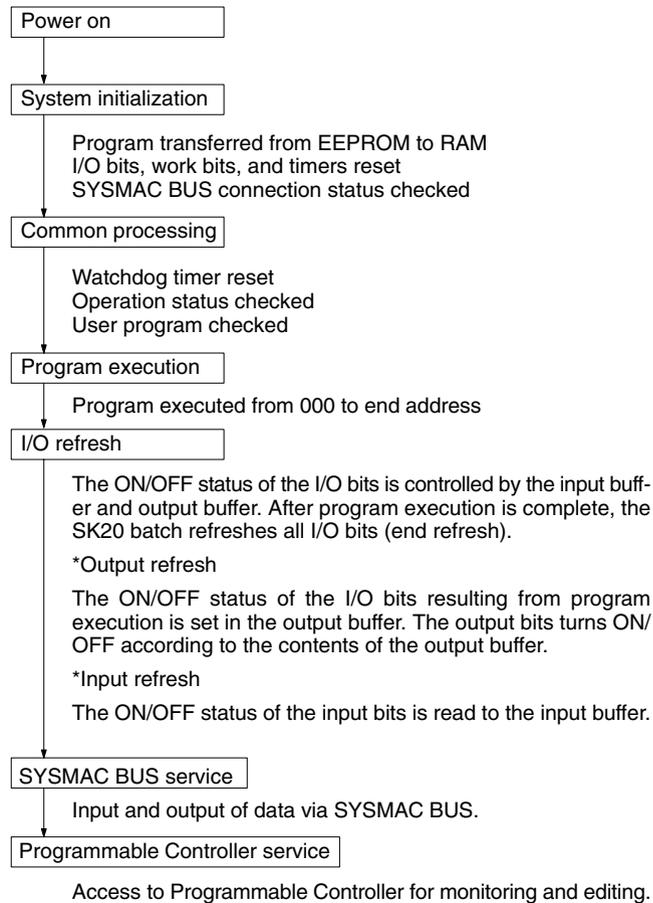
**Note** The watchdog timer is a timer which monitors the SK20 processing time. It monitors the processing time for each cycle and stops the CPU if the cycle time exceeds 100 ms.
