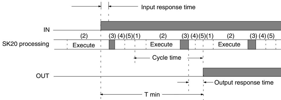
$$\text{Minimum response time} = \text{Input response time} + \text{Filter value} + \text{Cycle time} + \text{Output response time}$$
