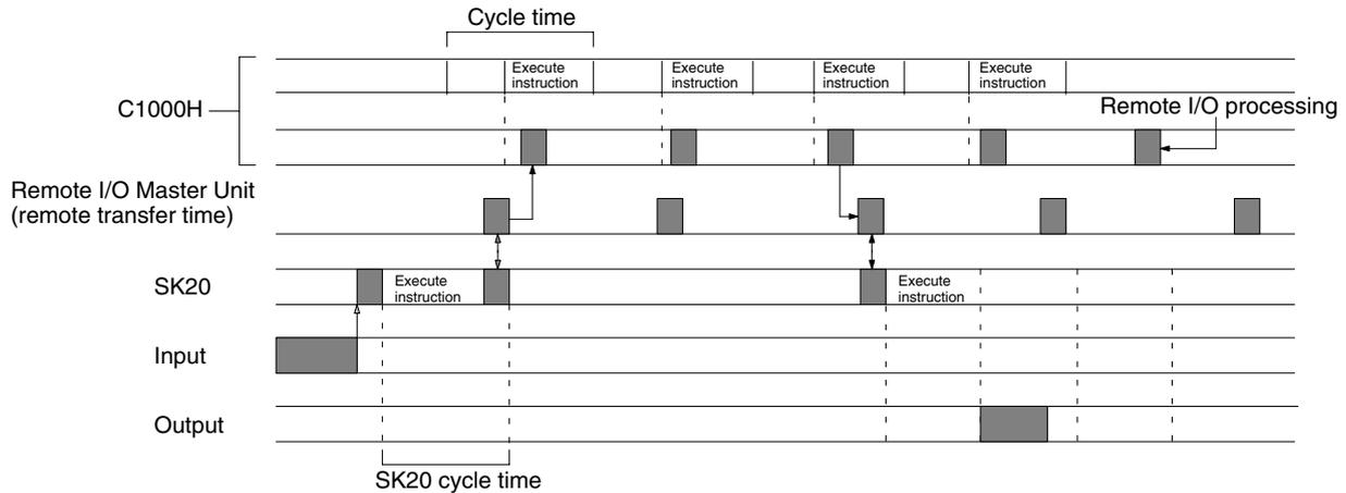
$$\text{Minimum response time} = (\text{C1000H cycle time} \times 2) + T_{RM} + \text{Output ON response time (10 ms)} + (\text{SK20 cycle time} \times 2)$$
