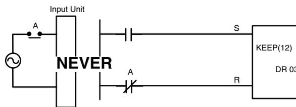
Bits used in KEEP are not reset in interlocks. Refer to the 3-7-10 *INTERLOCK and INTERLOCK CLEAR - IL(02) and ILC(03)* for details.
