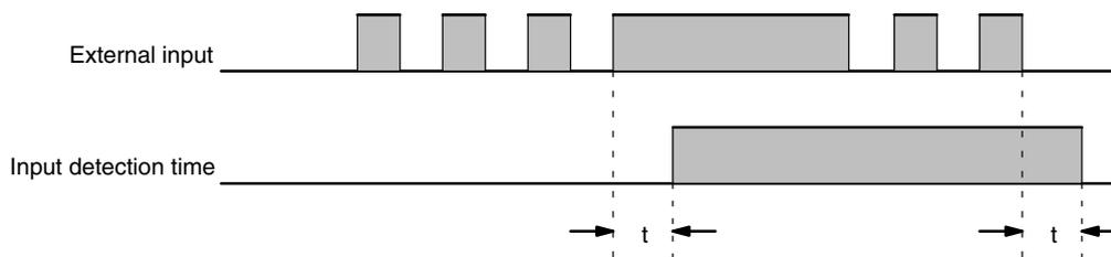
The input detection time,  $t$ , for the various possible settings is given in the following table. The “key” column shows which key is pressed to input each setting in the key sequence below.
