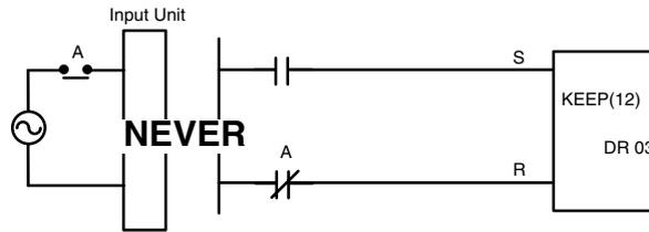
Bits used in KEEP are not reset in interlocks. Refer to the 3-7-10 INTERLOCK and INTERLOCK CLEAR - IL(02) and ILC(03) for details.
