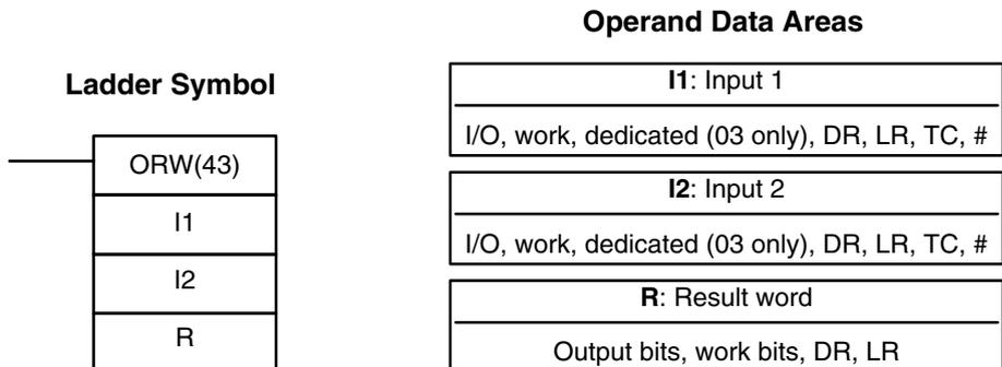
**Description** When the execution condition is OFF, ORW(43) is not executed. When the execution condition is ON, ORW(43) logically OR's the contents of I1 and I2 bit-by-bit and places the result in R.
