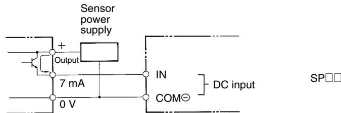
**Note** When using the DC model (SP□□-D□-D), do not input the signal through a NC contact (which makes the PC operate when the externally input signal
