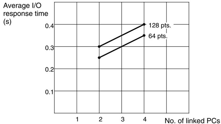
**Note** The duration required to process linked PCs is increased if a PC already linked is disconnected from the network.
