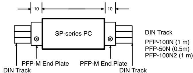
**Note** Remove the mounting screws when mounting on a track.
