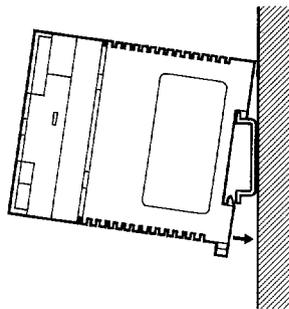
Engage the top hook to the track and push the PC in until the bottom hook locks onto the track.
