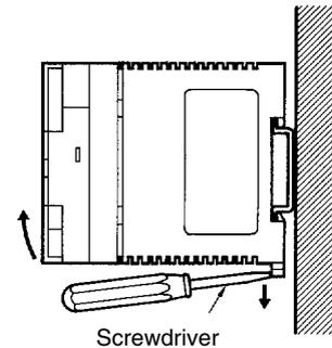
Push down the bottom hook with a screwdriver and push the PC upward.
