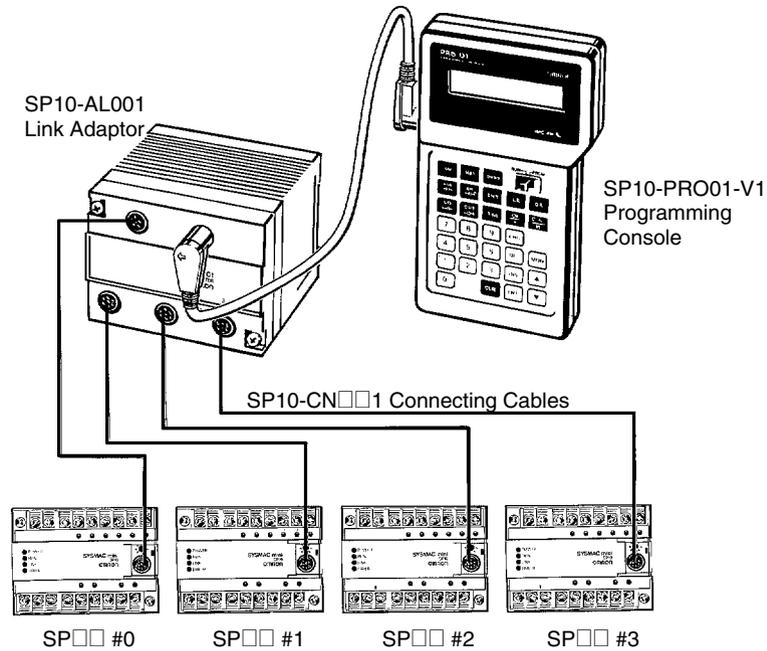
**Connecting Cable** Use one of the following Connecting Cables to connect the Programming Console.
