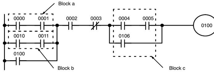
The first logic block instruction is used to combine the execution conditions resulting from blocks a and b, and the second one is to combine the execution condition of block c with the execution condition resulting from the normally closed condition assigned bit 0003. The rest of the diagram can be coded with OR, AND, and AND NOT instructions. The logical flow for this and the resulting code are shown below.
