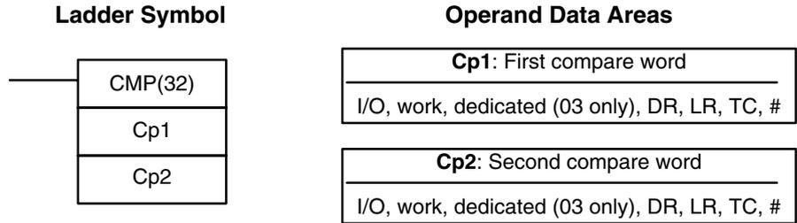
**Limitations** When comparing a value to the PV of a timer or counter, the value must be in BCD.
