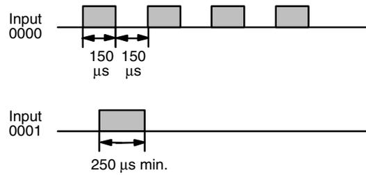
Inputs 0000 and 0001 can be used as normal inputs when CNTH(24) is not used, but the input signals must be 1 kHz max. (500  $\mu$ s wide min.).
