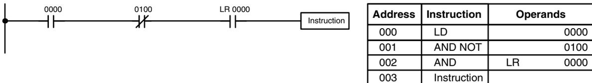
The instruction would have an ON execution condition only when all three conditions are ON, i.e., when bit 0000 was ON, bit 0100 was OFF, and LR 0000 was ON.
