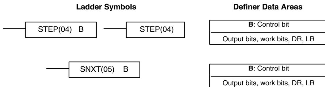
**Limitations** Control bits within one section of step programming must be sequential and from the same word.
