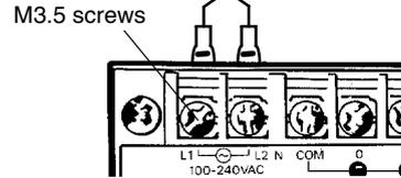
To reduce noise interference from the power lines, use twisted pair cables. Noise can also be significantly reduced by connecting a 1-to-1 isolation transformer.
