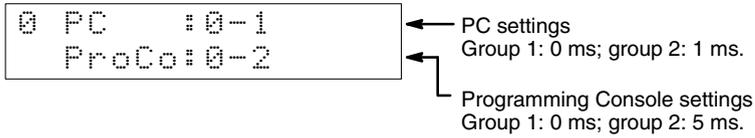
The display will show the settings for groups 1, 2, and 3 when the Programming Console is connected to an SP16 or SP20.
