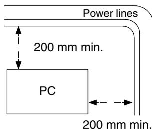
Whenever possible, use wiring conduit to hold the I/O wiring. Standard wiring conduit should be used, and it should be long enough to completely contain the I/O wiring and keep it separated from other cables.
