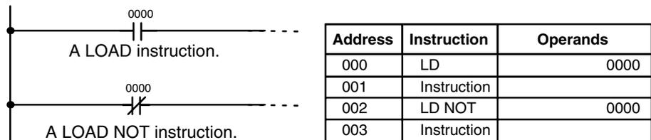
When this is the only condition on the instruction line, the execution condition for the instruction at the right is ON when the condition is ON. For the LOAD instruction (i.e., a normally open condition), the execution condition would be ON when bit 0000 was ON; for the LOAD NOT instruction (i.e., a normally closed condition), it would be ON when bit 0000 was OFF.
