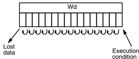
The execution condition on P functions like a differentiated instruction, i.e., I will be shifted into the register only when P is ON and was OFF the last time SFT(33) was executed. If execution condition P has not changed or has gone from ON to OFF, the shift register will remain unaffected.
