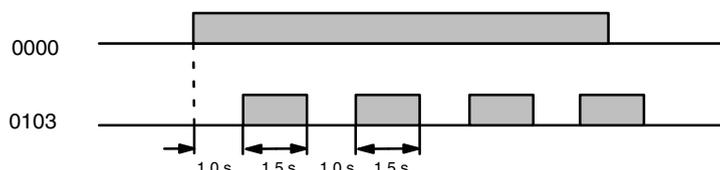
A simpler but less flexible method of creating a flicker bit is to AND one of the dedicated clock pulse bits with the execution condition that is to be ON when the flicker bit is operating. Although this method does not use TIM, it is included here for comparison. This method is more limited because the ON and OFF times must be the same and they depend on the clock pulse bits available.
