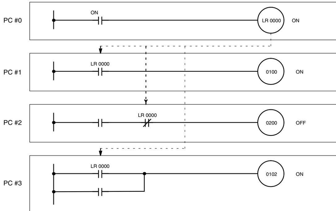
When LR 0000 of PC #0 is turned ON, LR 0000 of PC #1, #2 and #3 are also turned ON (OFF). LR 00 is the write area of PC #0, i.e., LR 00 of PC #1, #2 and #3 are used to read data written by PC #0.
