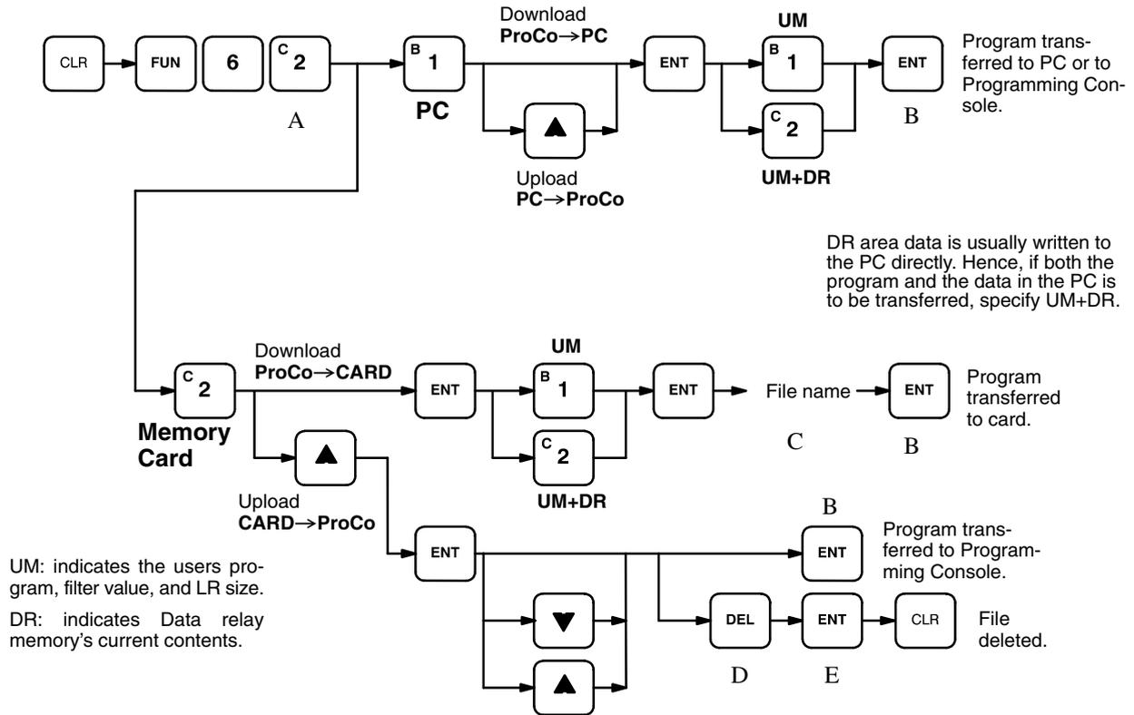
The Programming Console displays at different stages of the keying sequence are shown below.
