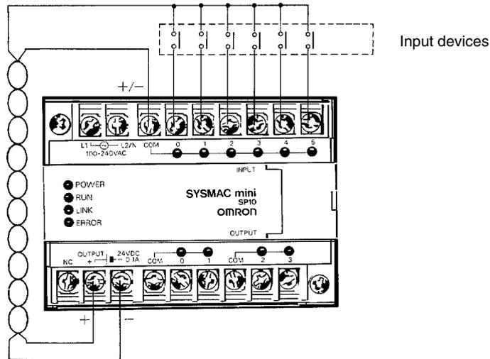
The power source of the SP10 for external supply is rated at 0.1 A, 24 VDC max., and the power source of the SP16 and SP20 is rated at 0.2 A, 24 VDC max. The input circuit consumes about 7 mA (typ. at 24 VDC) per input point.
