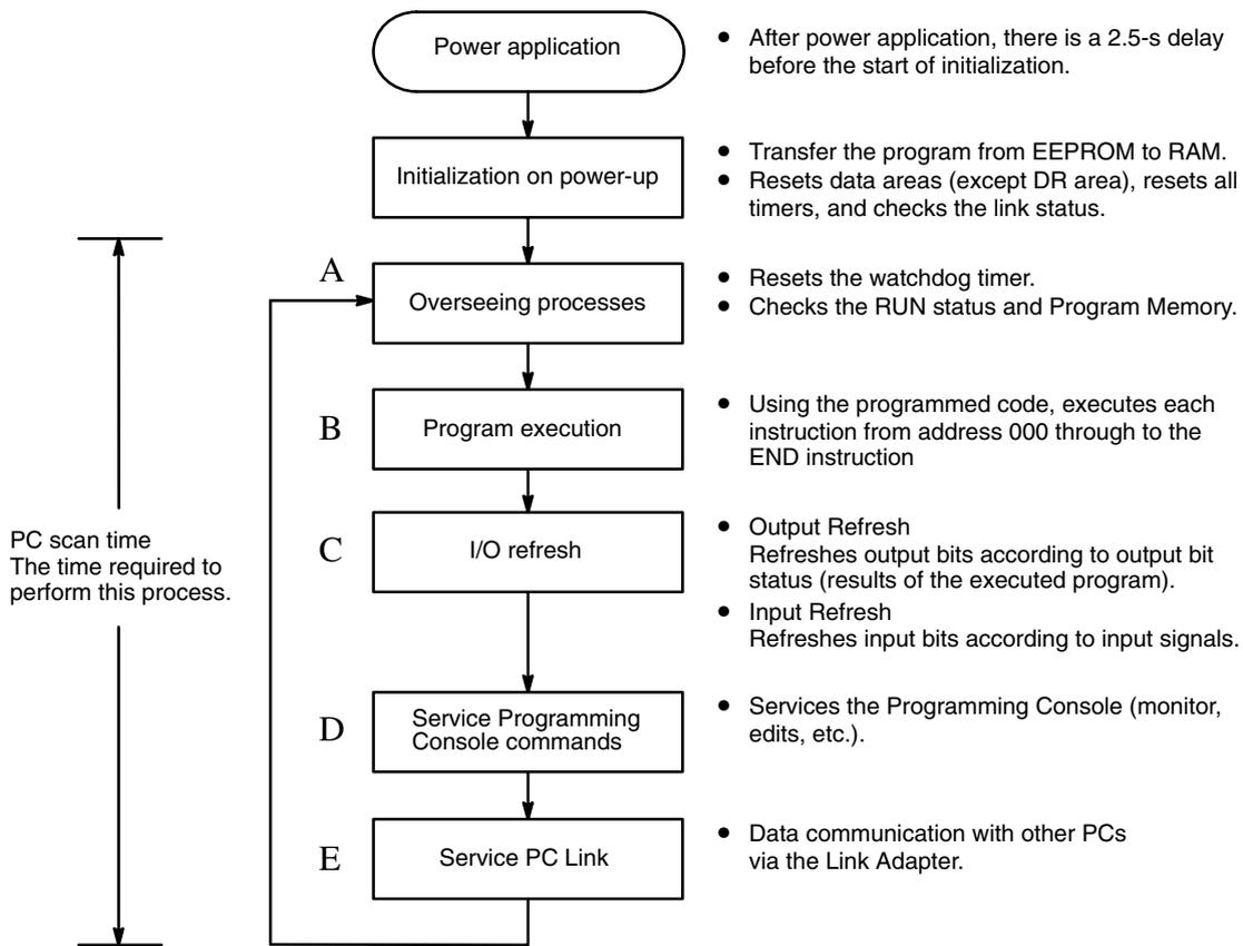
The first initialization process is performed only once, immediately after power is applied to the PC. The remaining operations are performed in cyclic fashion, with each cycle forming one scan. The scan time is the time that is required for the CPU to complete one of these cycles. This cycle includes basically five types of operation.
