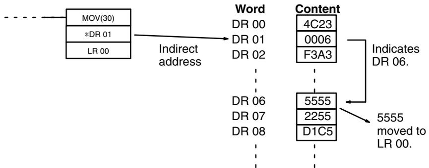
When using indirect addressing, the address of the desired word must be in BCD and it must specify a word within the DR area. In the above example, the content of \*DR 00 would have to be in BCD and between 0000 and 1515.
