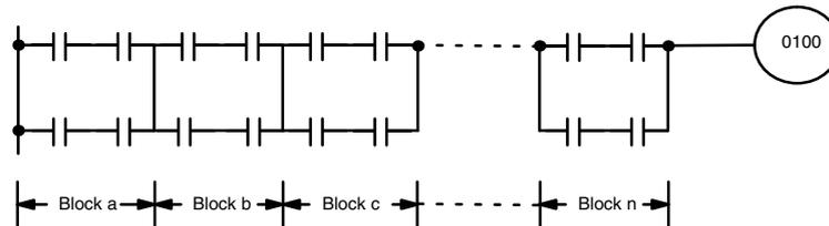
The following diagram requires an OR LOAD followed by an AND LOAD to code the top of the three blocks, and then two more OR LOADs to complete the mnemonic code.
