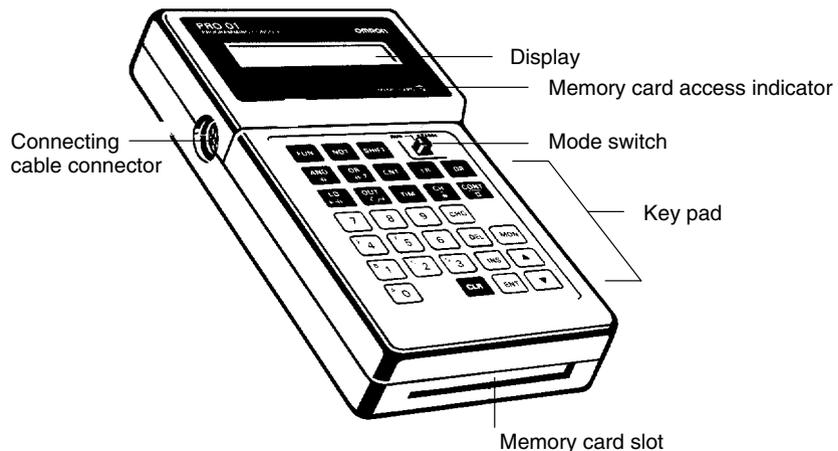
The Programming Console is used to write and transfer programs to the PC. It is also used to monitor operation and modify data. The Programming Console can be connected directly to the PC for single PCs. It can also be connected via a Link Adapter when PCs are connected in a PC Link configuration to access each PC individually without reconnection.
