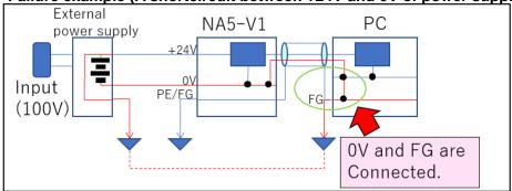
\*If a shortcircuit is made between the 24V-side of the NA5-V1 and the ground terminal (Positive grounding), change the wiring (measure 1), or isolate the external power supply and NA5-V1(measure 2).
