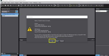
6. The Sysmac Studio goes online and the color of the bar under the toolbar changes to yellow. Then, click the Synchronization icon. Or, select Synchronization – NA Device from the HMI Menu.
