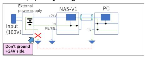
Measure 2 (Isolate the external power supply and NA5-V1)
