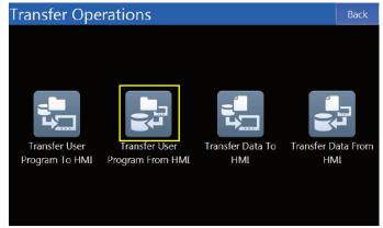
Specify the destination media and file name and touch the Transfer from HMI Button. The project is uploaded to the specified media.
