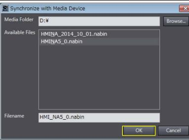
The project on the Sysmac Studio is compared with the project in the storage media and the Synchronization Window is displayed.
