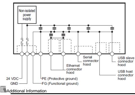
The internal power supply of the NA5-□□W□□□□ Product uses an isolated DC power supply, and therefore is not susceptible to the effects of grounding of the 24V side.
