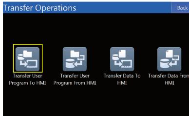
8. Select the project to transfer and touch the **Transfer to HMI**Button. The selected project is downloaded to the HMI.
