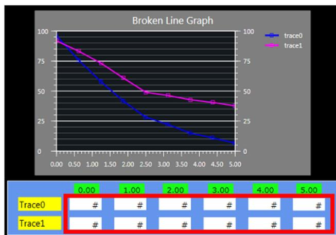
4. Transfer the project to the actual NA unit. Click [HMI]-[Online] to set the unit in the online status. Then, click [HMI]-[Synchronization]-[NA Device]. Connect the PC with the NA unit in advance using the cable that complies with the communications setup. Perform the communications setup in [Communications Setup] under [HMI] on the menu bar.
