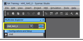
Change the NA name for easy identification. Right-click the NA NA Training - HMI\_NA5\_0 - Sysmac Studio File Edit View Insert Project HMI Simulation Tools Hel icon and select "Rename". 単 課 品 図 図 く Multiview Explorer HMI\_NA5\_0 dd Device Change Dev Configurations and Setup Rename 6. Change the name to "NA\_1". NA Training - NA\_1 - Sysmac Studio File Edit View Insert Project HMI Simulation Tools He 11 元 4 日 日 公 人 ? Multiview Explorer NA\_1 Configurations and Setup
