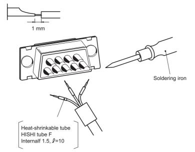
**4** Push the heat-shrinkable tubes back over the soldered joints, then heat them using a jetter to shrink them in place.
