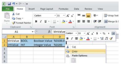
Paste the variables in the device variable table of the HMI project.
