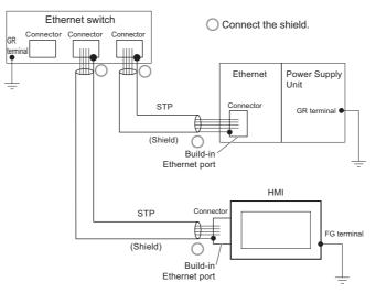
(b) Connecting each shield only to the switching hub side
