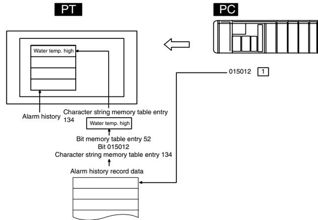
The PC bit allocated to the bit memory table entry for which the history property has been set is continually monitored: when the bit turns ON (1), the time, the number of times, and the contents of the character string memory table entry registered for the bit memory table entry are recorded in the alarm history record data.
