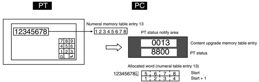
**Reference:** When the PT is set to NT20S or NT30/620 compatible mode, the word configuration is identical to that of the earlier NT20S, NT30, NT30C, NT620S, NT620C, and NT625C PTs.
