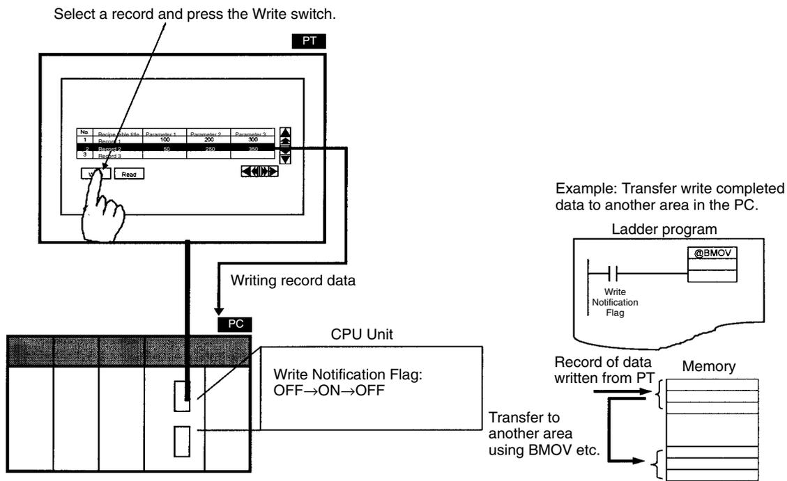
**Reference:** Recipe tables and recipe elements are stored in flash memory within the PT and memory (recipe data memory) that is backed up by a battery. (The Battery is an option for the NT21.) The way that the data is stored is explained below and illustrated in the diagram following.
