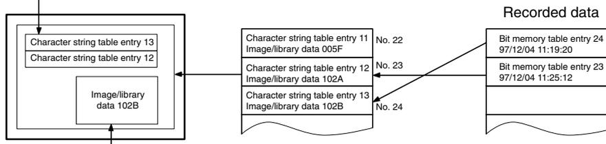
When the upper message displayed is pressed, the image/library data (102B) set for bit memory table entry 13 is displayed.
