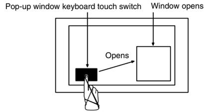
Also, by creating window move touch switch on window, it is possible to move a window by touch panel operation at the PT.
