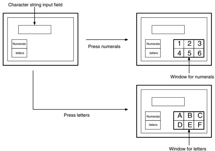
**Reference:** In order to make numeral/character string settings, a key to confirm the input numeric value or character string is required. Assign the ENT input key-control or Enter (
