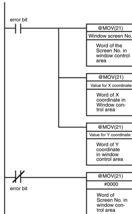
With this ladder program, the specified window is displayed at the designated position when the error bit comes ON, and the window is closed when the error bit goes OFF.
