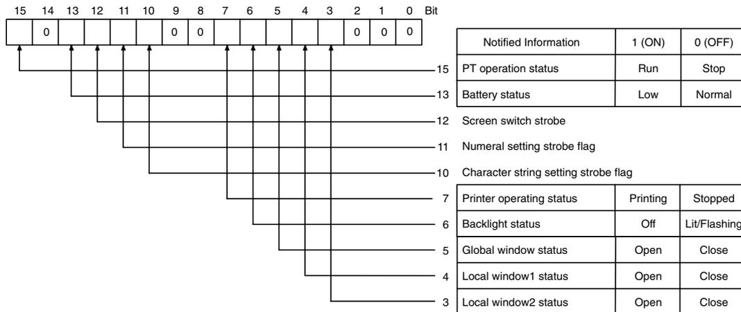
The printer operating status (bit 7) is not supported by the NT21.
