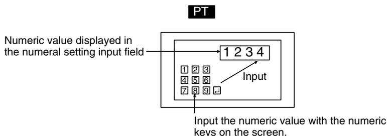
2. On confirming the input numeric value with the ENT key or touch switch it is written to a numeral memory table entry.
