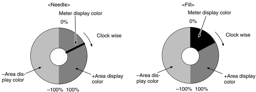
**Donut-shaped Analog Meter (Width Rate)**
