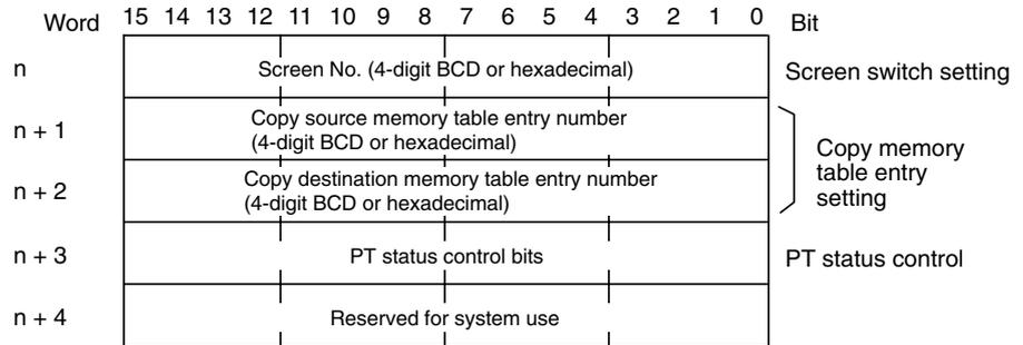
The configuration and functions of these words are different when the PT is in NT20S or NT30/620 compatible mode.
