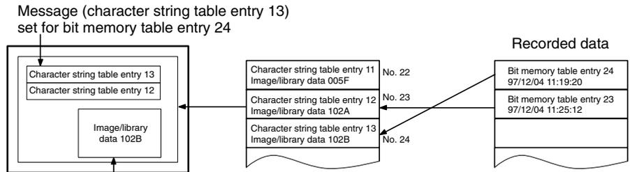
When the upper message displayed is pressed, the image/library data (102B) set for bit memory table entry 13 is displayed.
