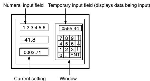
However, if there is not even one numeral setting input field (numeric key type) or character string input field on the base screen, the temporary input field will not be displayed (cannot be used).
