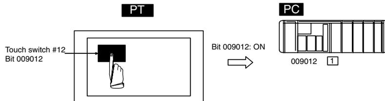
The lamp comes on (flashes) when the PC's bit (lamp bit) is ON (1) and goes OFF when it is OFF (0). When the touch switch is pressed, the PC's notification bit comes ON (1) or goes OFF (0).
