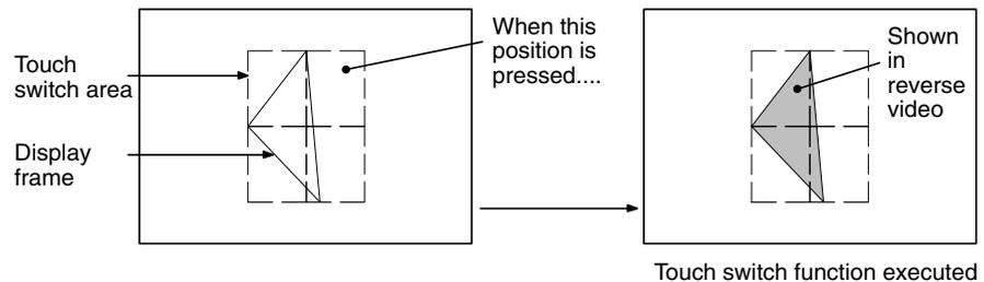
**Note** Do not press touch switches with a force of greater than 30 N. Applying higher force may cause the glass to break, cause injuries, and prevent operation.
