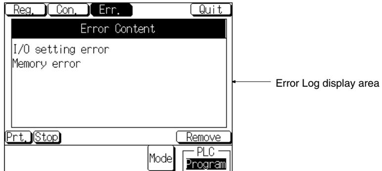
With the NT31/NT31C, 5 error records can be displayed in one screen. The highest priority error must be cleared in order to display the sixth error record.
