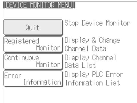
2. Select the desired Device Monitor screen. The selected screen will be displayed.
