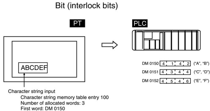
Allocate any desired words in the PC to character string table entries. When text is input with a character string input, the new character string will be written to the character string memory table entry and the contents of the words allocated in the PC will be changed automatically. This function allows text to be written from the PT to the PC easily.
