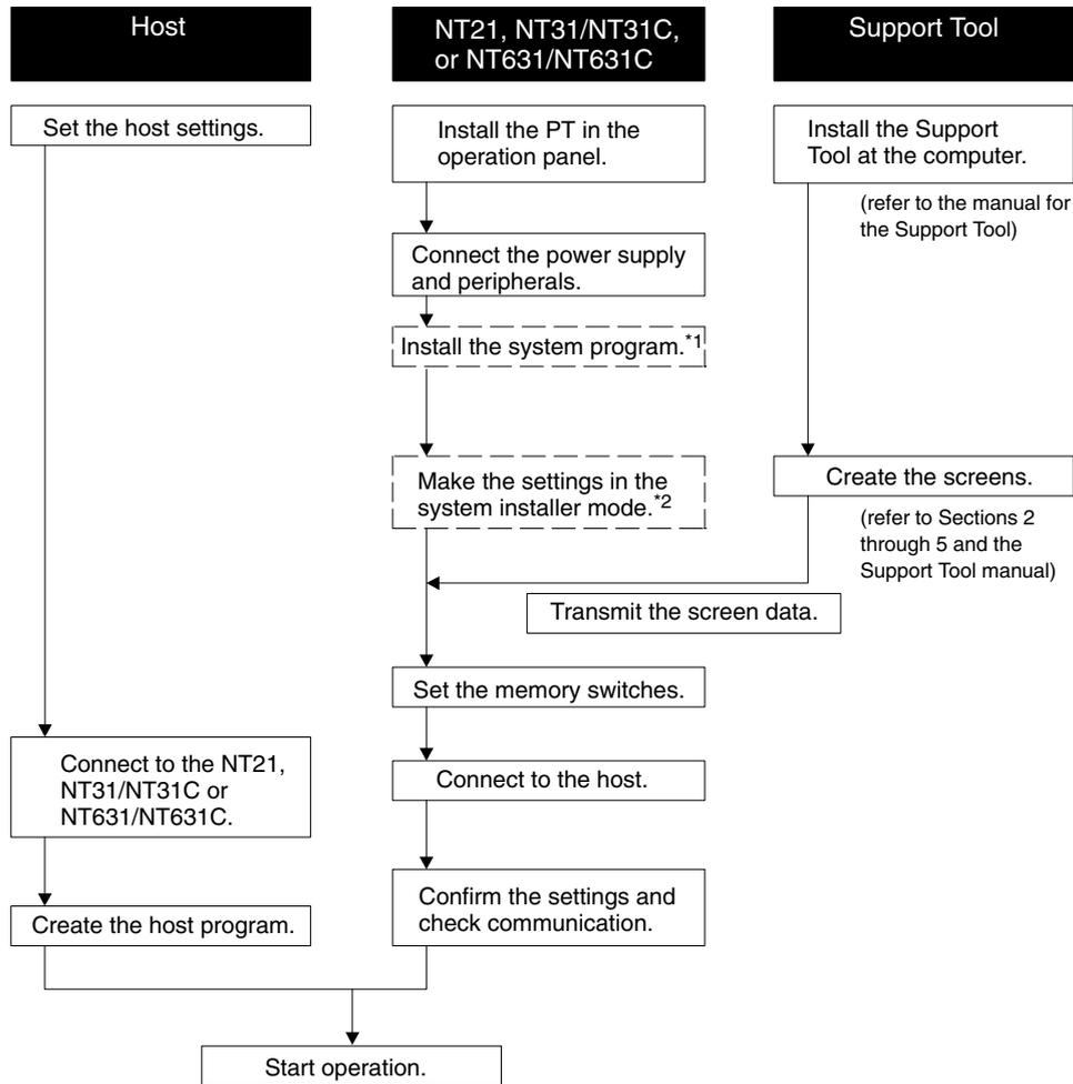
\*1: System program installation is only done in special circumstances, for example when changing the system program, or to recover the original status of the installed program. This operation is not normally necessary. When using other PC models (sequencers), however, it is necessary to install specific system programs.
