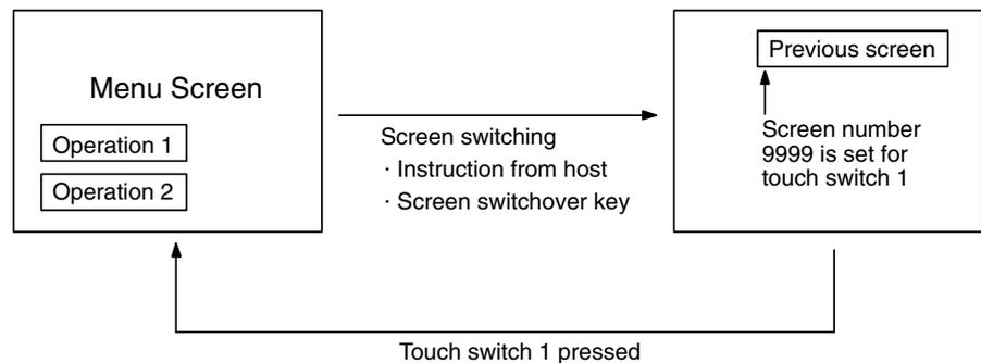
**Switching the Screen by Using the Switch Screen Function of the Bit Memory Table**
