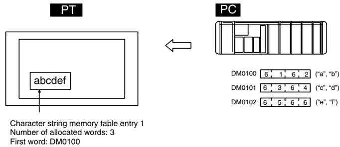
Allocate any desired words in the PC to character string memory table entries. If the contents of the allocated words are changed while the character string memory table data is being displayed on the screen as text, the corresponding display on the screen will also change automatically. This function allows any desired message to be displayed easily.
