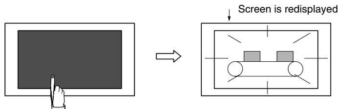
**Caution** Do not press the touch panel carelessly while the backlight is off or while the screen is displaying nothing.
