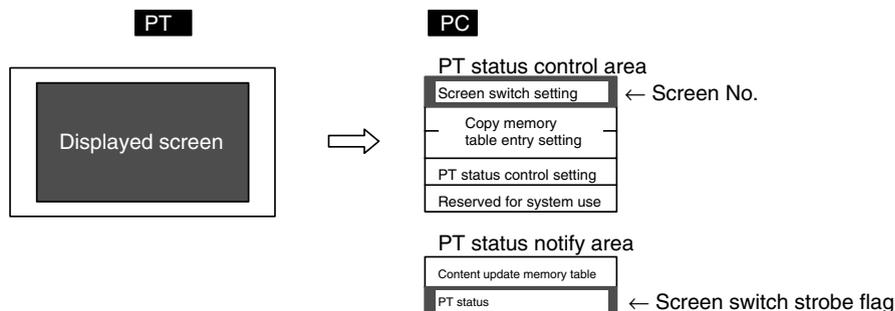
**Reference:** When NT20S or NT30/620 compatible mode is being used, the current screen number occupies the first word of the PT status notify area and the word containing the PT status notify bits is shifted down one word. (Refer to page 451.)
