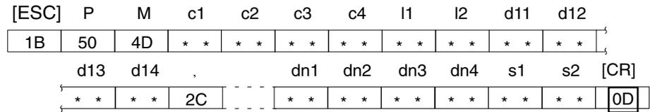
c<sub>1</sub> to c<sub>4</sub>: Word address of the changed direct area (4 BCD digits)
