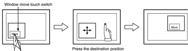
**Reference:** When a window control area is allocated words in the host, the bottom left coordinate of the window after moving operation is notified to the window control area. (Refer to page 312)
