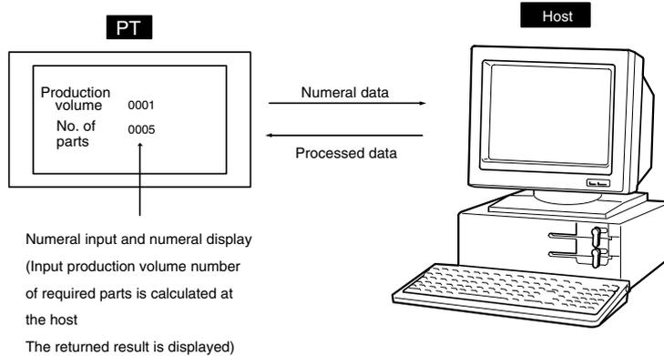
When the numeral was input on PT, numeral input notify command (sent from PT to host) is issued from the PT. At the host, numeral data was taken out and processed, then it is written to the PT by the numeral memory table write command (sent from host to PT).
