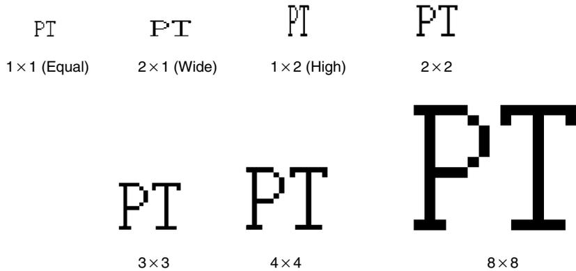
With ISO 8859-1 font type, the character strings of 2 × 2 or larger scale are automatically displayed in 32 dot high-definition font. However, the marks inserted into a string are always displayed in 16 × 16 dot font.
