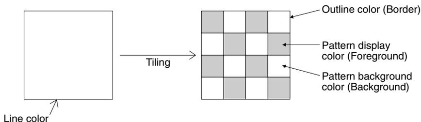
**Reference:** When a lamp, a touch switch, and a graphic are displayed in color, part of the frames of the display elements may be invisible because of the combination of the background, outline, and tiling colors. This is a phenomenon peculiar to a color LCD, not a failure of the system. In such a case, change the color combination.
