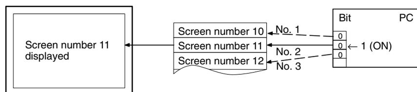
If the allocated bits of multiple bit memory table entries come ON at the same time, the bit memory table entry with the smallest number takes priority.
