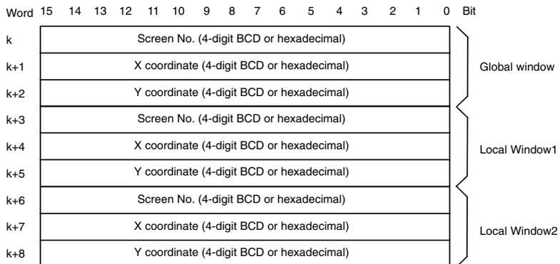
**Reference:** It is not necessary to allocate words in the host for window control area when the window is not controlled from the host or when the window is not used.
