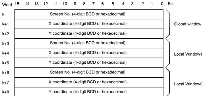
With the program in the host, read out window screen number, X coordinate and Y coordinate in a window control area that corresponds to the window of which display status is to be checked.
