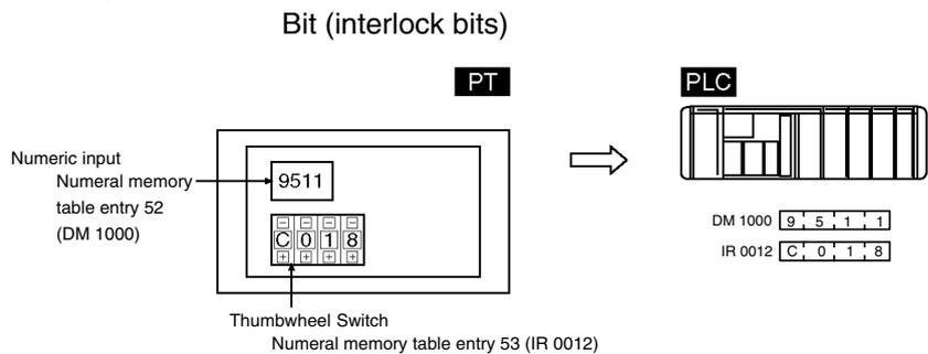
Allocate any desired words in the PC to the numeral memory table entries. When a value is input or changed with the numeric input or thumbwheel switch, the new value will be written to the numeral memory table entry and the contents of the words allocated in the PC will be changed automatically. This function allows word PVs to be changed easily from the PT.
