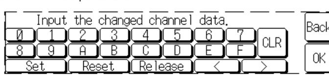
When the input window is displayed, the binary PV cell will change as shown below to receive the new hexadecimal PV.
