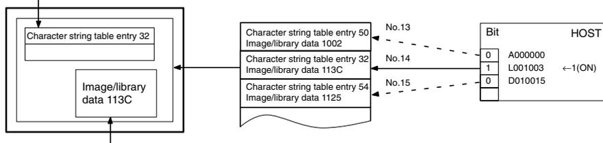
When the message displayed is pressed, the image/library data (113C) set for bit memory table entry 14 is displayed.
