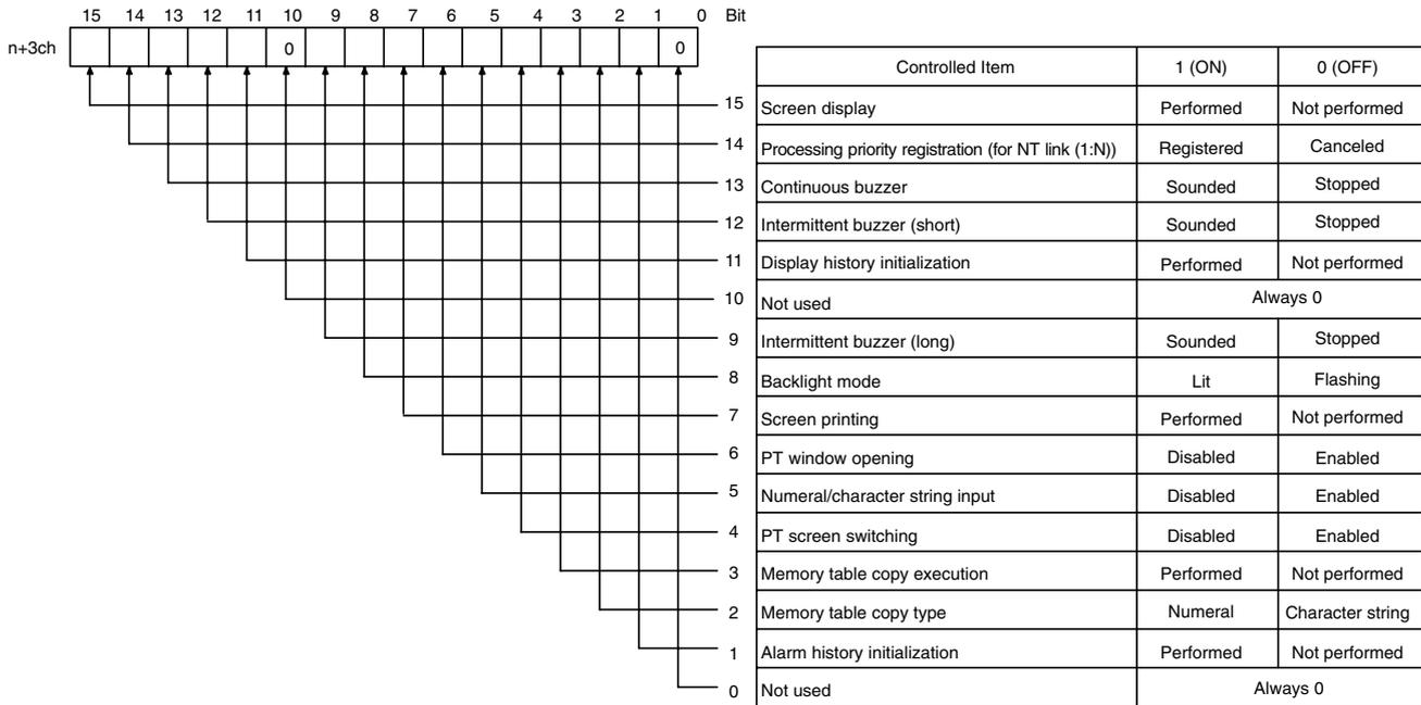
The backlight mode bit (bit 8) is not supported by the NT631.
