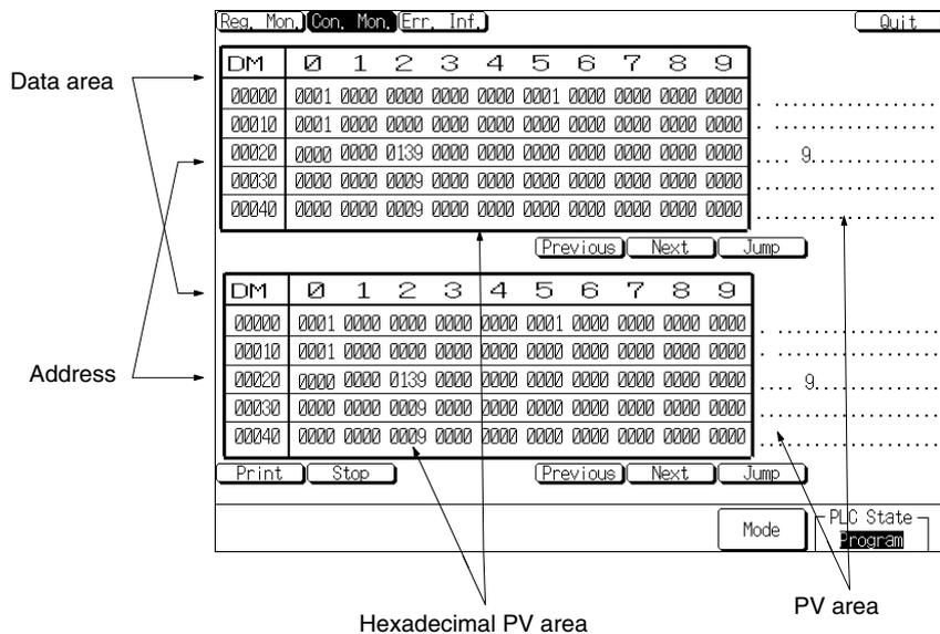
With the NT631/NT631C, two tables of 50 words (10 words × 5 rows) can be displayed simultaneously for a total of 100 words.
