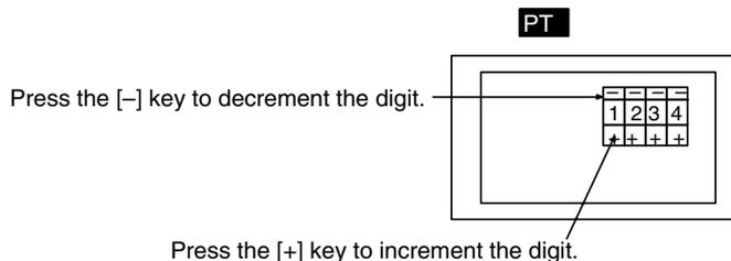
2. Each time a change is made to the numeric value it is confirmed and the occurrence of the change is notified to the host via the PT status notify area.
