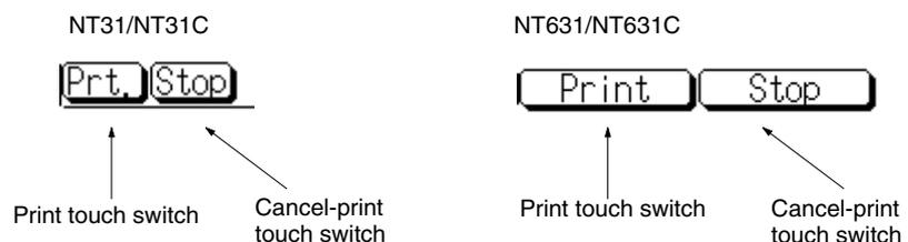
Press the print touch switch to print a copy of the current Device Monitor screen. The screen print can be cancelled by pressing the cancel-print touch switch.
