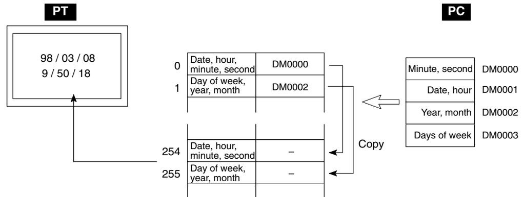
To copy a memory table entry, either use the PT status control area or the touch switch copy setting function. Here, the procedure for copying a memory table entry using the PT status control area is described. For the procedure for using the touch switch copy setting function, refer to *Changing Numeric Values/Character Strings by Pressing a Touch Switch That Has the Copy Setting Function* (page 325).
