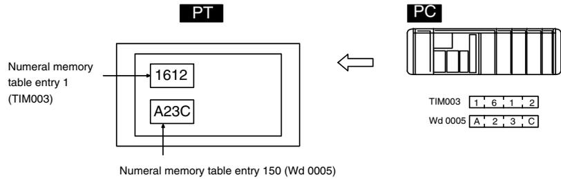
Allocate any desired words in the PC for numeral memory table entries. If the contents of the allocated words are changed while the numeral memory table data is being displayed on the screen as numeric values or lamps, the display on the screen will also change automatically. This function allows the contents of allocated words to be monitored easily.
