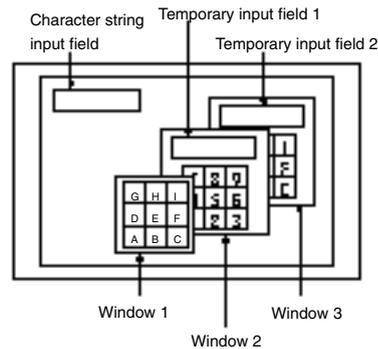
In the example above, window 2 is a focus window. All the input indicated below is performed to a temporary input field on window 2.
