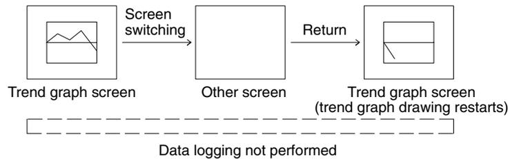
**When the Data Logging Function Is Used and the Background Function Is Not Used**
