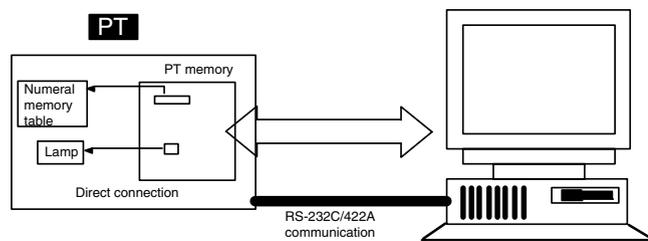
In the memory link method, the only difference is that the PT finds its communication target inside instead of outside. In the memory link method, therefore, change of the target is all that is needed to be capable of using the exact screen data that is acquired by the direct connection. (With the NT21, NT31/NT31C, and NT631/NT631C, the Support Tool must be used to convert the data to screen data for the memory link.)
