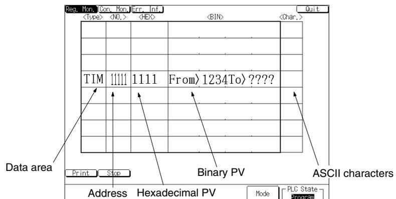
With the NT631/NT631C, the PVs of up to 8 words can be displayed simultaneously.
