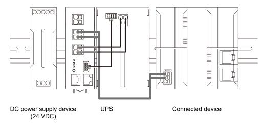
When using the UPS monitoring software or the I/O signal, connect the unit to the target device with a connection cable.
