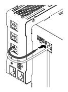
(5) Battery communication cable UPS control unit side
