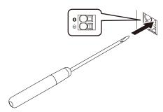
With the tip of the flat blade screwdriver in the hole, insert a cable into a round hole at the left of the terminal block.
