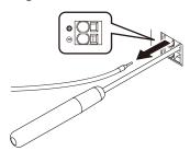
2 Pull out the flat blade screwdriver.
