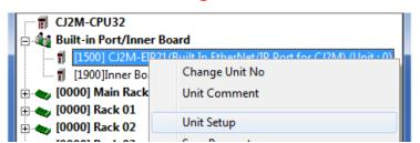
The Edit Parameters Dialog Box is displayed. Select the **TCP/IP**Tab.
