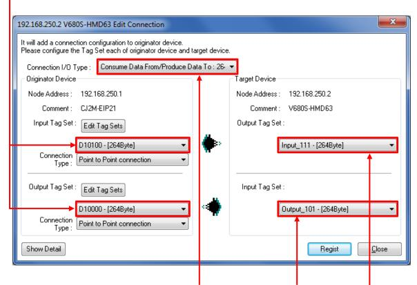
■Setting the connection I/O types and tag sets of target device (RFID Reader/Writer)
