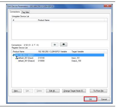
When the connection setting is completed, the registered node address is displayed under the device icon of node 2 on the Network Configuration Pane.
