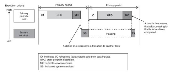
For the NX Controller that incorporates a multi-core CPU, tasks and system services are executed in parallel. Even if a DoS attack occurs, control tasks remain unaffected and therefore do not virtually affect the control period.
