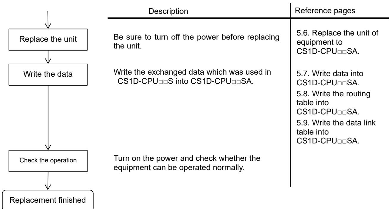
**Figure 2-4: Replacement flow using the support tool**
