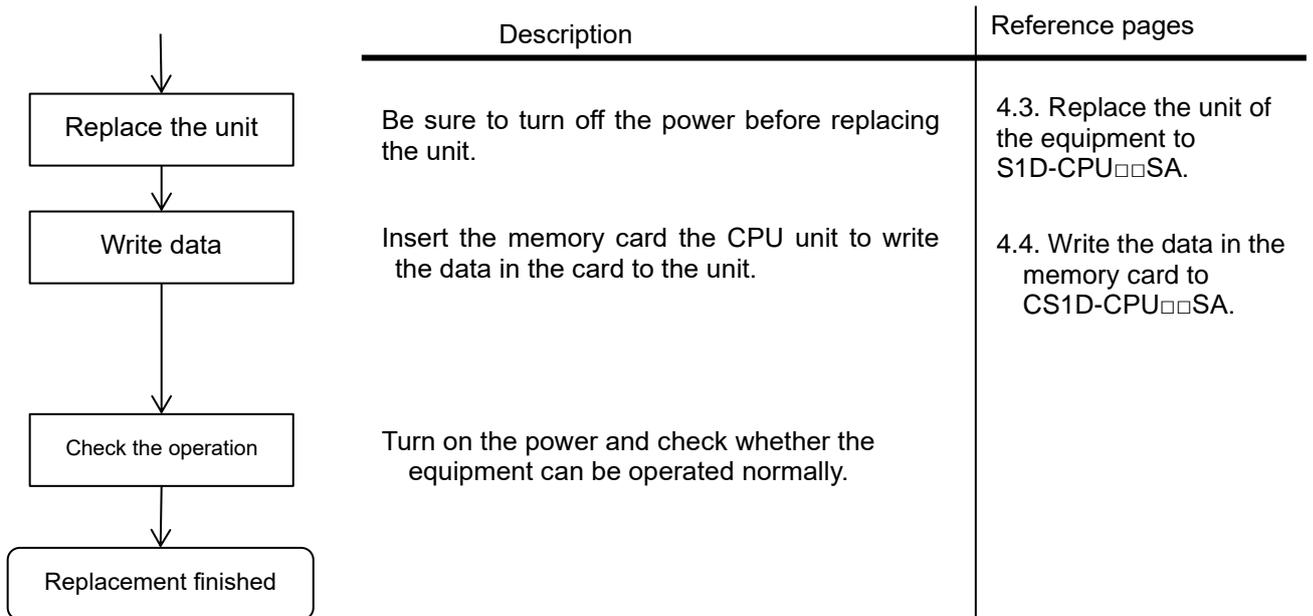
**Figure 2-2: Replacement flow using a memory card**
