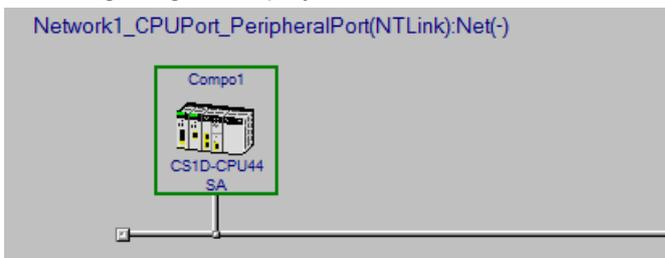
(7) Select **Data link table setting tool** of the CX-Integrator. (**Tools –Start Data Link**)
