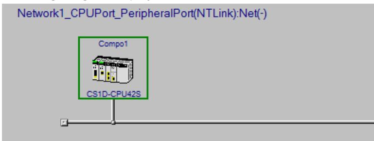
(7) Open the data link table setting tool from the CX-Integrator. (**Tools – Start Data link**)
