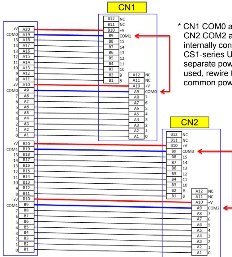
\* CN1 COM0 and COM1 and CN2 COM2 and COM3 are internally connected in the CS1-series Unit. When separate power supplies were used, rewire to use one common power supply.
