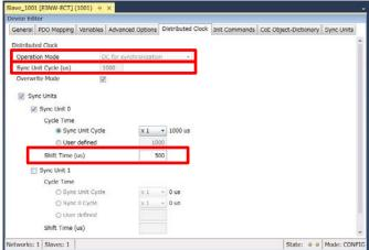
Correspondence between the servo frequencies of the Controller and **Shift Time** values is as follows:
