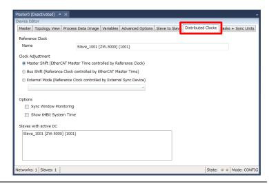
2 Select Master Shift (EtherCAT Master Time controlled by Reference Clock).
