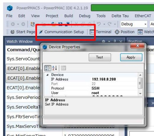
**8** In the Device Properties dialog box, select *No Device* for IP Address, then click the **Apply** button.
