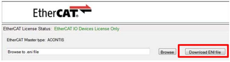
A screenshot of the "EtherCAT" system setup window. The "EtherCAT License Status" is "EtherCAT IO Devices License Only" and the "EtherCAT Master type" is "ACONTIS". There is a "Browse to .eni file" button and a "Download ENI file" button. The "Download ENI file" button is highlighted with a red rectangular box.
