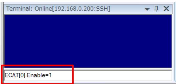
The screenshot shows a terminal window titled "Terminal: Online[192.168.0.200:SSH]". The command "ECAT[0].Enable=1" is entered in the input field at the bottom of the terminal, highlighted with a red box.
