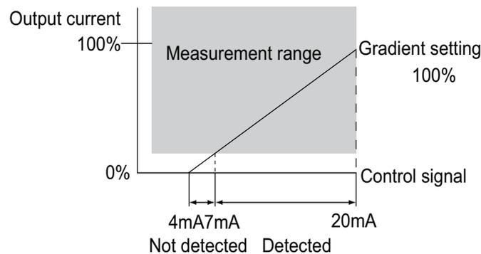
When the power regulator's gradient settings are changed, the operation gate current level is set to so that the output current is within the measurement range. (In the following diagram, 14mA is set.)
