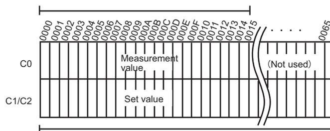
Variable type C0: Read-only parameters for the measurement value (load current, trip count, etc.)
