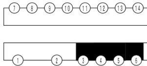
Alarm outputs are output from the terminal number (3) to (6).
