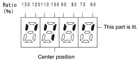
With the value at the center as a standard value, when the “set value is smaller than the measurement value”, the indicator moves to the left from the center, and when the “set value is larger than the measurement value”, the indicator moves to the right.
