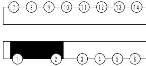
Supply power to terminal number (1) and (2). The power supply specifications are outlined below.
