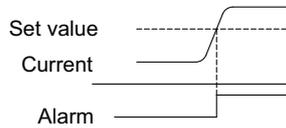
Transistor output models: ALM indicator lit, ALM transistor output
