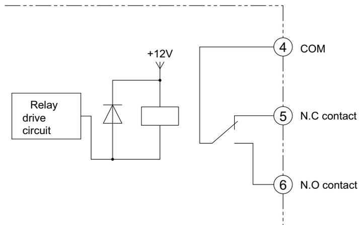
Note: For contact outputs, the same outputs are used for SSR error and for heater burnouts and heater layer short circuit alarm outputs.
