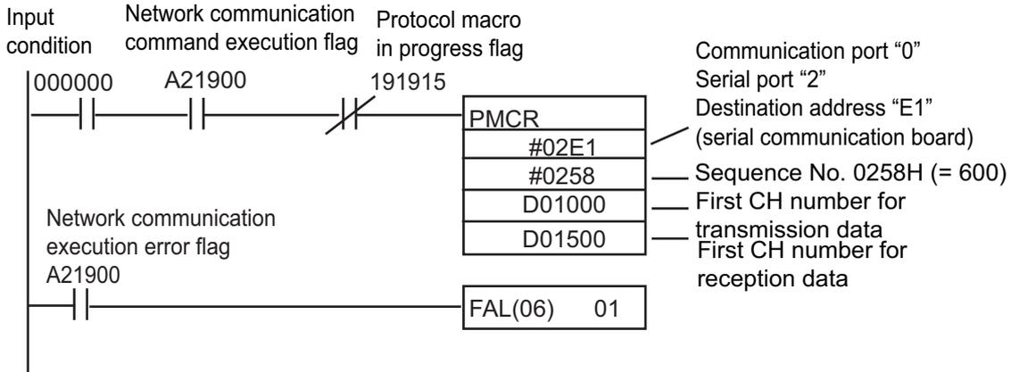
Placing the "read present value" command in D01000 or a higher-numbered location causes the present value to be stored in D0152 to D0153. If a communication error occurs, an FAL command (continuous operation failure diagnosis command) is executed.
