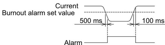
Transistor output models: ALM indicator lit, ALM transistor output
