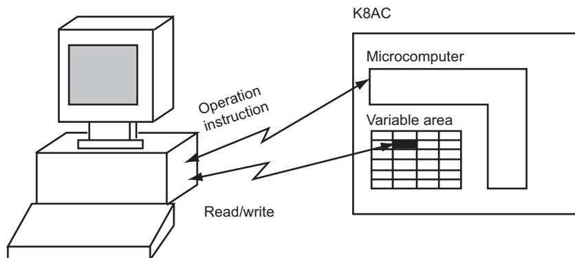
A variable area is accessed by specifying the position of a variable within the variable area using the variable type and address.
