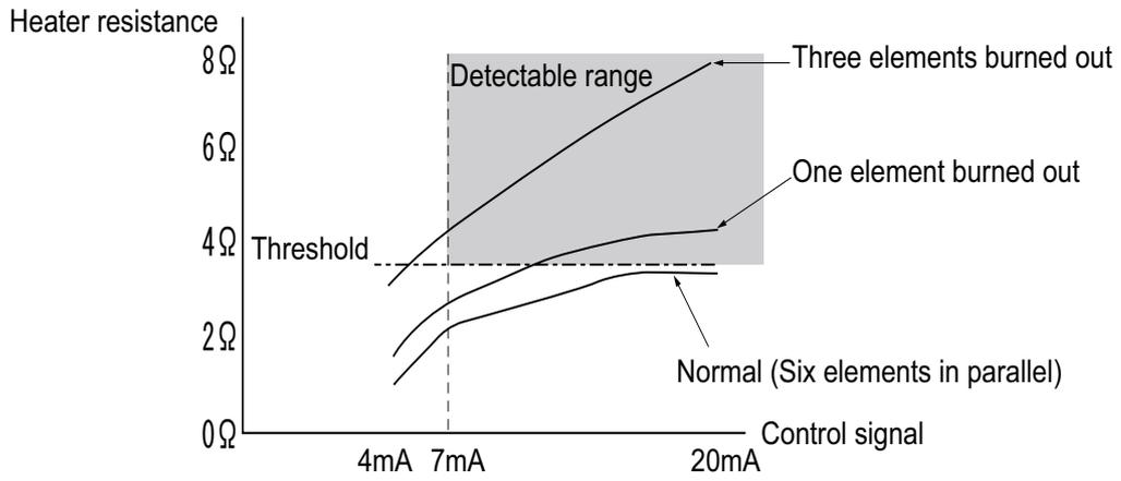
Note: The K8AC-H is designed to detect the disconnection of a load close to a pure resistance (e.g. electric wire heater).
