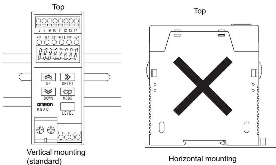
Wrong mounting may deteriorate heat dissipation, resulting in damaged or broken internal elements. Do not use the K8AC-H if not mounted using the standard mounting procedure.
