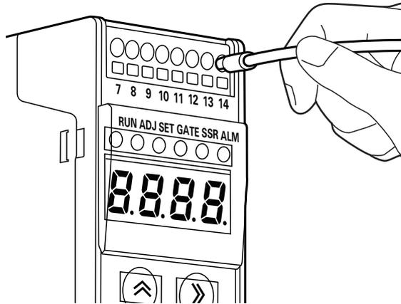
**Removing wires from the screw-less clamp terminal**
