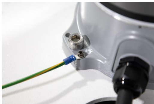
Figure 37: Grounding position for the robot
