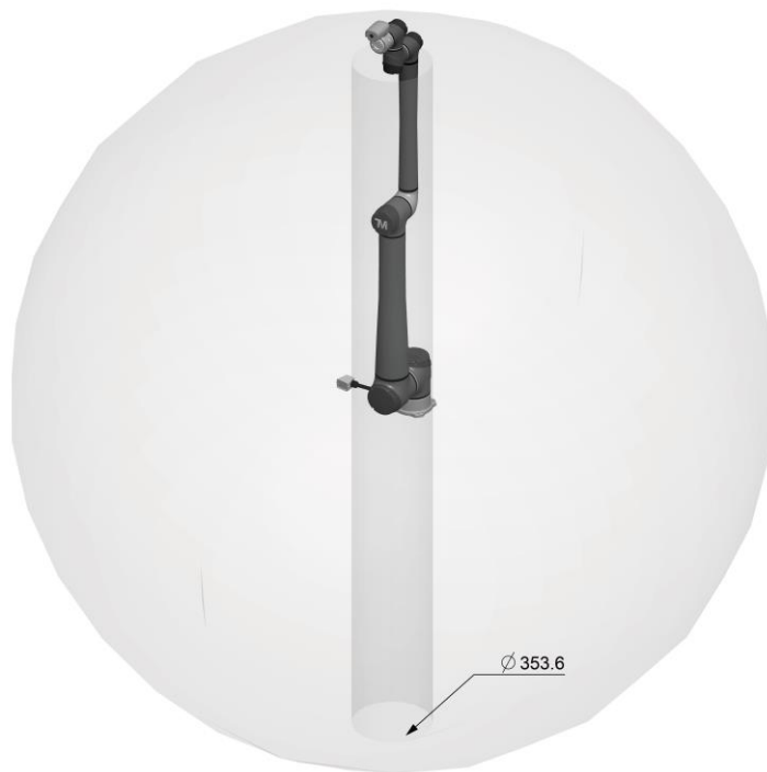
Figure 21: Pictorial view of TM6S / TM6S-M / TM6S-X / TM6S-MX Movement Range Diagram
