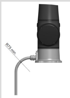
Figure 97: Connecting the Robot and the Control Box
