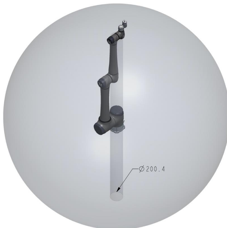
Figure 11: Pictorial view of TM25S / TM25S-M / TM25S-X / TM25S-MX Movement Range Diagram
