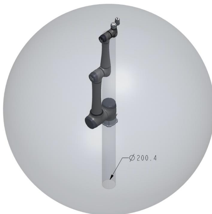
Figure 14: Pictorial view of TM30S / TM30S-M / TM30S-X / TM30S-MX Movement Range Diagram
