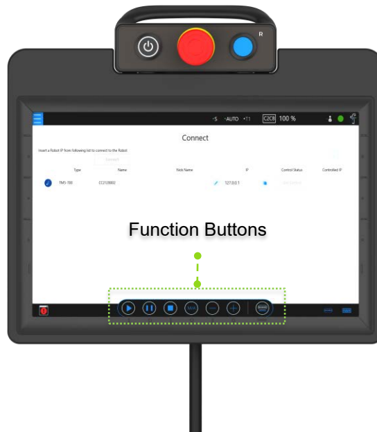
Figure 32: TM Teach Pendant (consisting of the TM Screen and Robot Stick)
