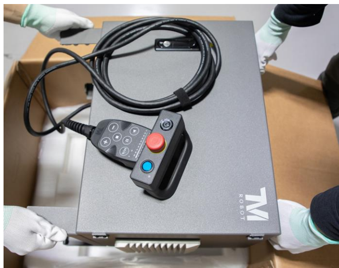
Figure 66: Moving the Control Box (2/2)
