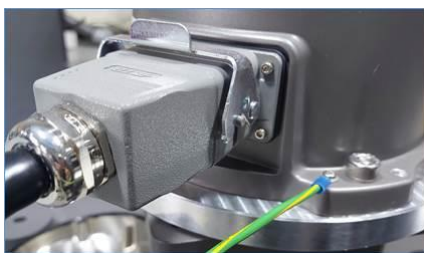
Figure 14: Grounding position for the robot
