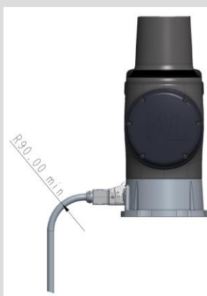
Figure 69: Connecting the Robot and the Control Box
