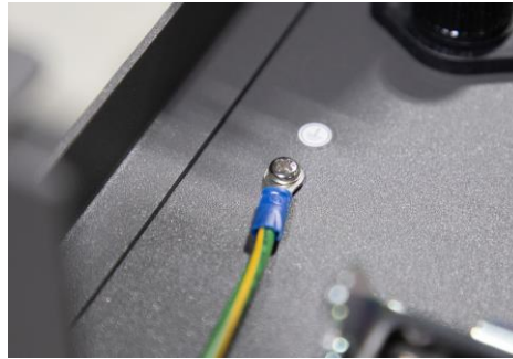
Figure 20: Securing the ground wire with control box
