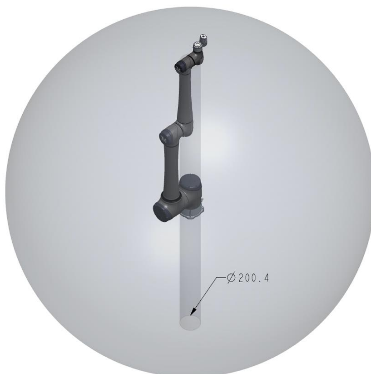
Figure 9: Pictorial view of TM25S / TM25S-M / TM25S-X Movement Range Diagram
