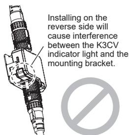
**Step5:** Secure the K3CV firmly with a cable tie.
