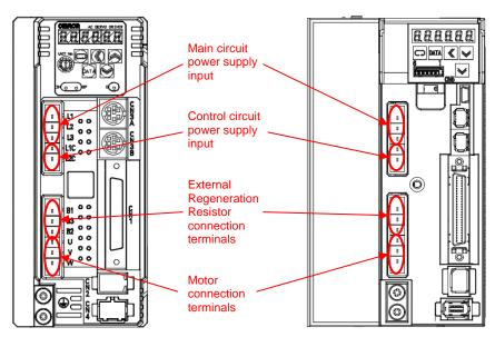
In both the G and the G5 series, input single-phase 100 V and 200 V to the L1 terminal and the L3 terminal.
