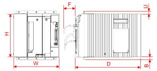
■ Main circuit power supply voltage 200 V drive dimensions
