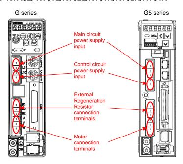
In both the G and the G5 series, input single-phase 100 V and 200 V to the L1 terminal and the L3 terminal.
