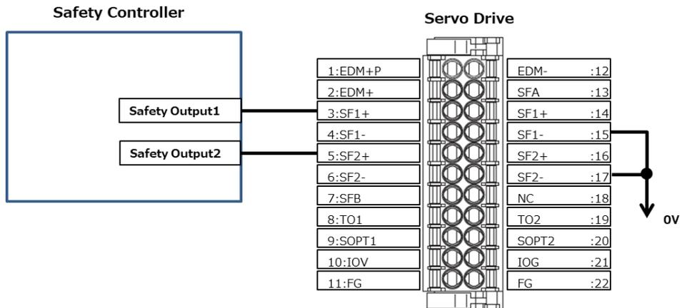
3. When using hard-wired STO for multiple Servo Drives, make the wiring between the Safety CPU Unit and the Servo Drives as shown below.
