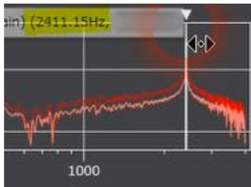
Activate the 1<sup>st</sup> notch filter to remove this resonance frequency at 2411 Hz:
