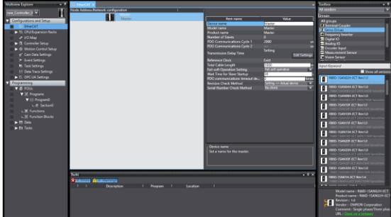
3. Drag a Servo Drive from the Toolbox to the Master in the EtherCAT Tab Page.
