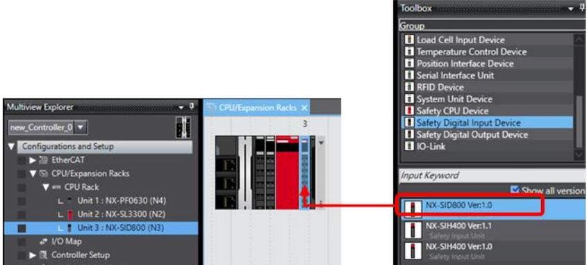
5. **Drag a digital input device to the location where you want to add it in the CPU and Expansion Racks Tab Page.**
