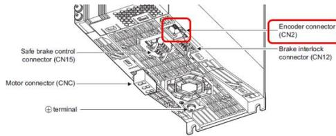
11. **When you use a motor with a brake, plug the brake cable into the Servo Drive. (CN12)**
