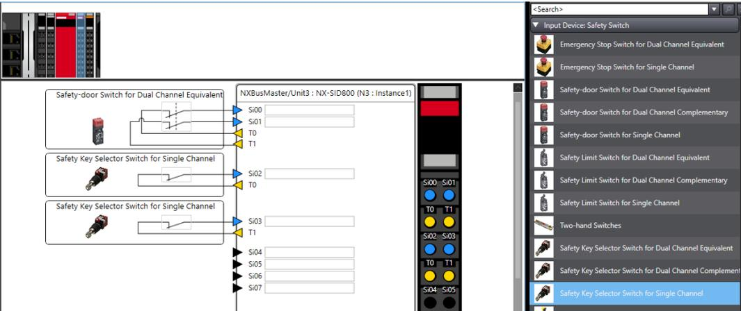
5. Drag an emergency stop pushbutton switch to the desired I/O terminal.
