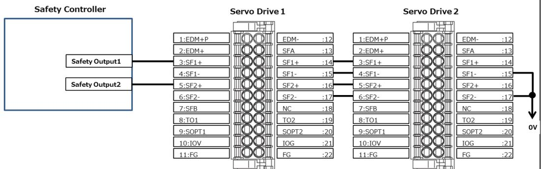
**Note:** When using a G9SP-series Safety Controller, you can connect up to four 1S-series Servo Drives.
