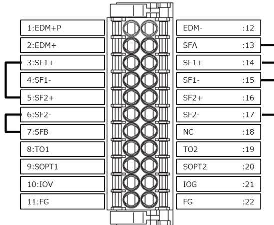
2. When using hard-wired STO, make the wiring between the Safety CPU Unit and the Servo Drive as shown below.
