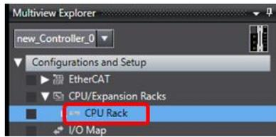
2. Drag a system unit device to the location where you want to add it in the **CPU and Expansion Racks Tab Page**.
