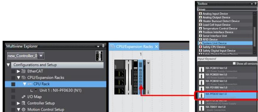
3. Drag a safety CPU device to the location where you want to add it in the **CPU and Expansion Racks Tab Page**.
