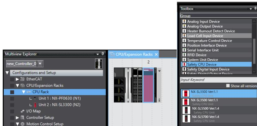
4. **Drag a safety digital input device to the location where you want to add it in the CPU and Expansion Racks Tab Page.**
