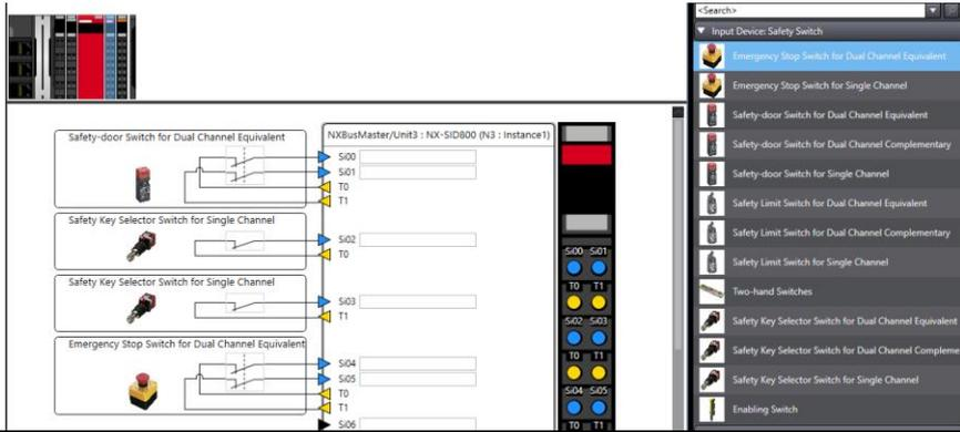
6. Drag a reset switch to the desired I/O terminal.
