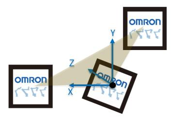
Figure 2: Vision base created on the basis of three OMRON Landmarks
