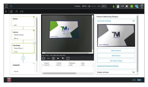
Figure 9: Object Positioning
