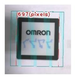
Figure 36: Caliper (Peak-to-Peak Width) Example
