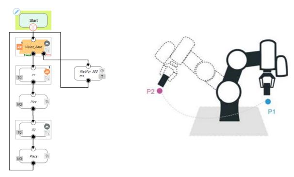
Figure 6: The Flow of Pick and Place
