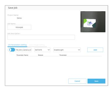
Figure 7: Set I/O Parameters Based on Results
