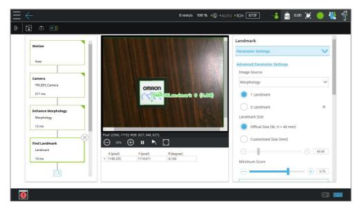
Figure 11: Landmark Positioning (1/2)
