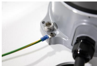
Figure 17: Grounding position for the robot
